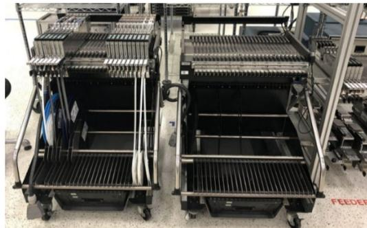
Figure 1: Example of a feeder unit cart
