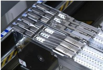
Figure 5: Example of tape feeders
