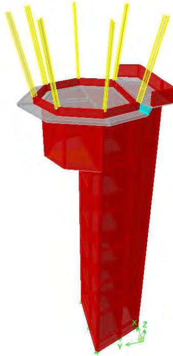
**Figure 4-57 Finite Element Model for the Airport Control Tower of British Virgin Island [202].**
