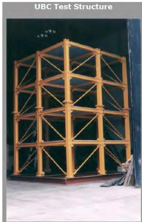
**Figure 4-17 ASCE Benchmark model in University of British Columbia**
