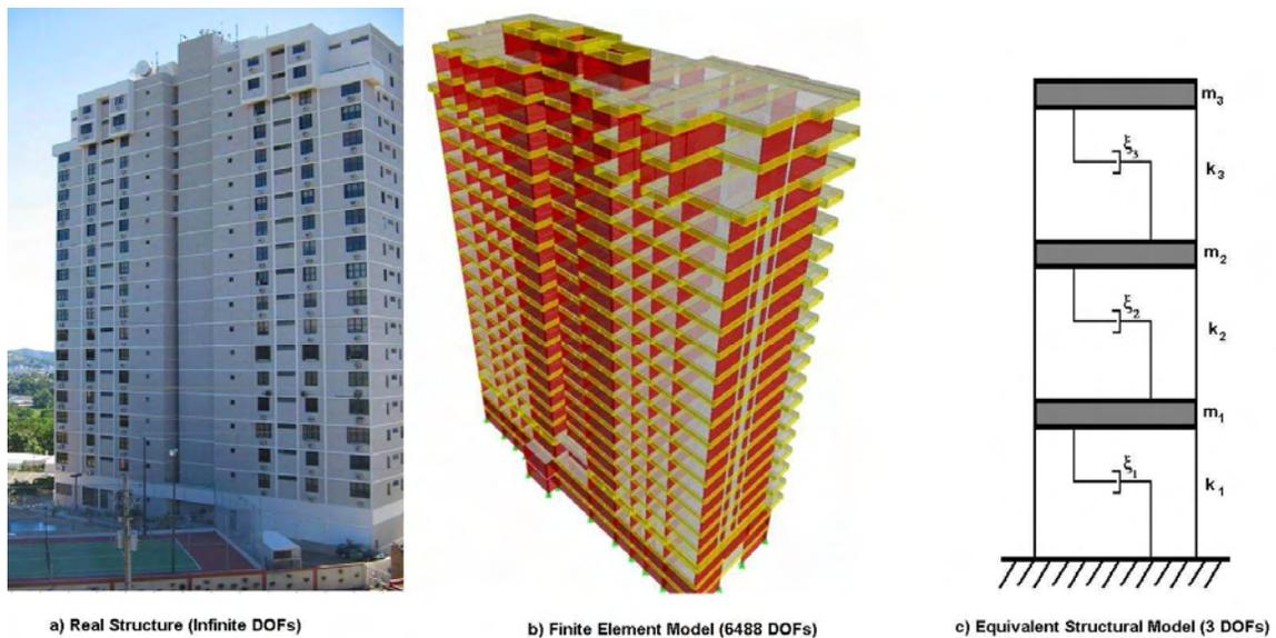
**Figure 4-2 Typical Equivalent Structural Model**
