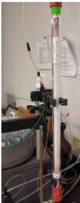
**Figure 3.2. XK 16/70 column with strong anion exchange Q Sepharose High Performance (QHP).**
