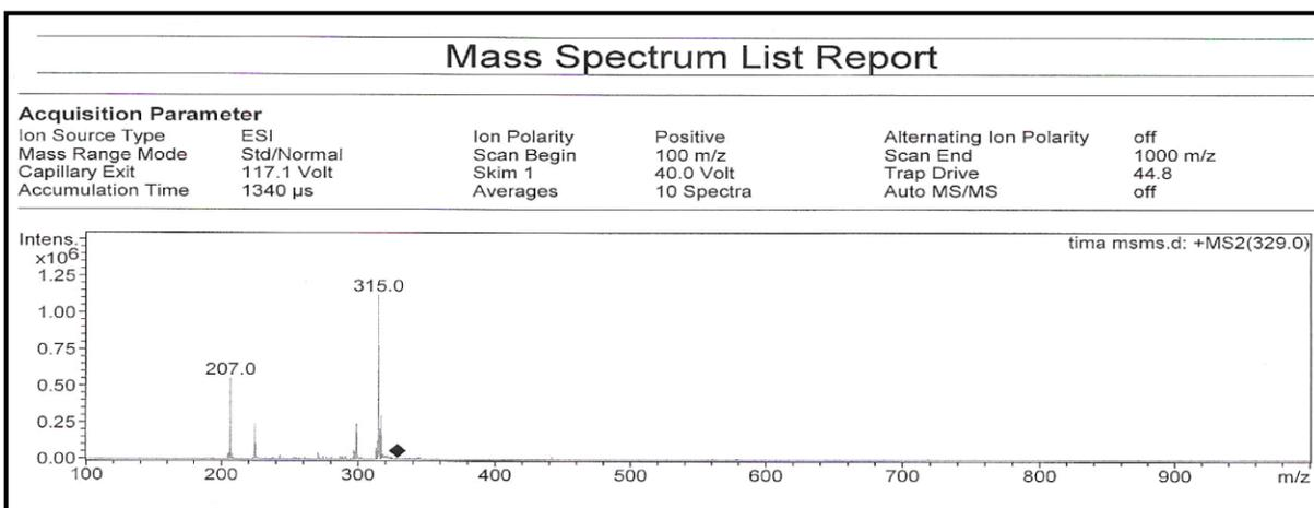
Figure 3- 8: MS spectrum for the fragmentation of the parent peak 329 m/z
