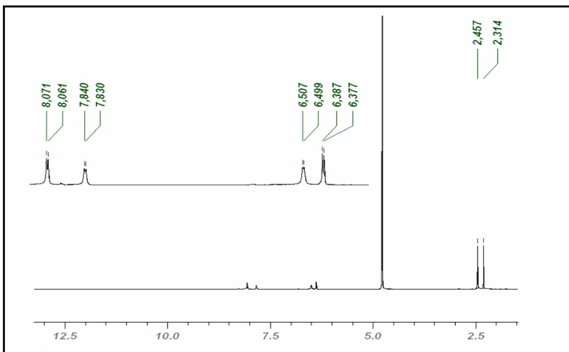
**Figure 3-2: The 500-MHz <sup>1</sup>H NMR spectrum of Ti(maltolato)<sub>2</sub>(OH)<sub>2</sub> in DMSO-d<sub>6</sub> after the addition of D<sub>2</sub>O to the sample solution at room temperature**
