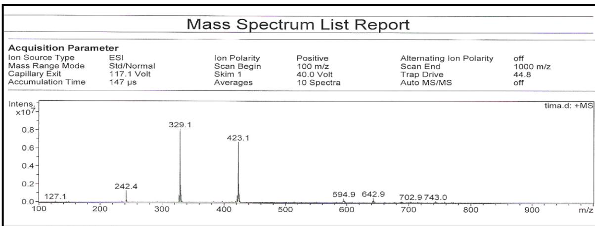
Figure 3- 7: MS spectrum for  $\text{Ti(maltolato)}_2(\text{OH})_2$
