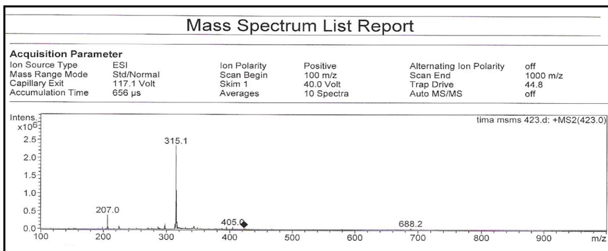
**Figure 3- 9: MS spectrum for the fragmentation of the 423 m/z peak**
