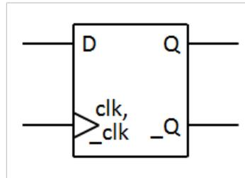
Figure 3–6: D flip-flop symbol, where D, `clk`, and `_clk` are inputs; and Q and `_Q` are outputs.
