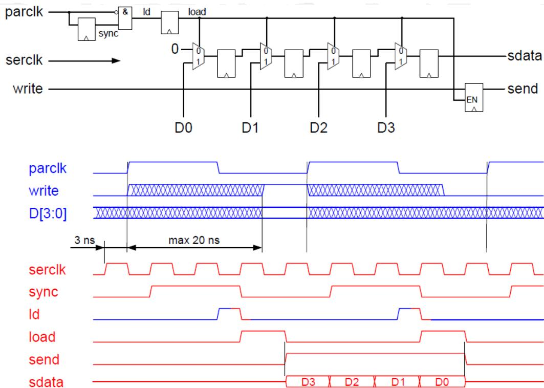
Figure 5–14: Diagram of the serializer and signal involved in its performance.
