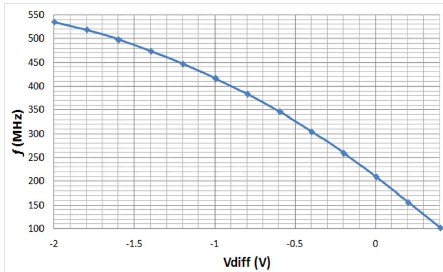
Figure 4–4: The VCO frequencies for different  $V_{diff}$  values when  $V_{DD} = 2$  V and  $V_{com} = 1$  V.
