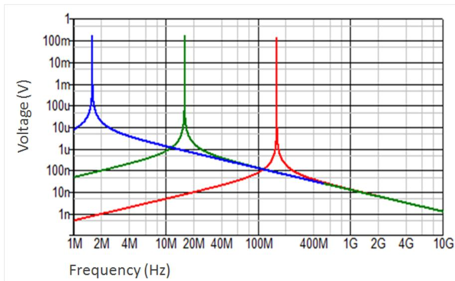
Figure 4-10: Voltage fluctuations as a function of frequency when adding a 1 F capacitor in parallel to the connecting cable. Each curve is for a different cable inductance. 1 pH (red), 100 pH (green), 10 nH (blue).
