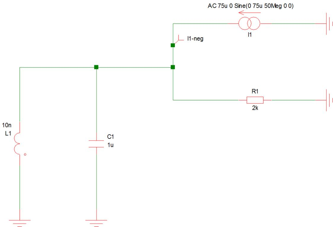
Figure 4–8: AC equivalent circuit for the connection to the power supply.
