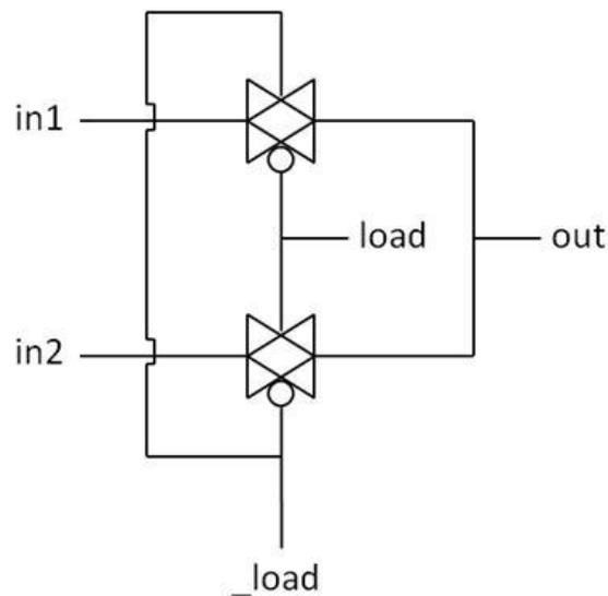
Figure 5–13: Block 4 design using 2 transmission gates interconnected.
