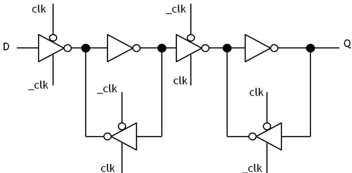
Figure 5-4: D flip-flop design called dff.
