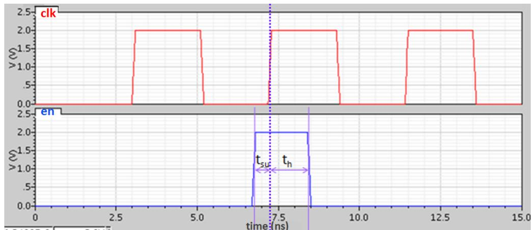
Figure 5–8: Parameters of the enable signal.
