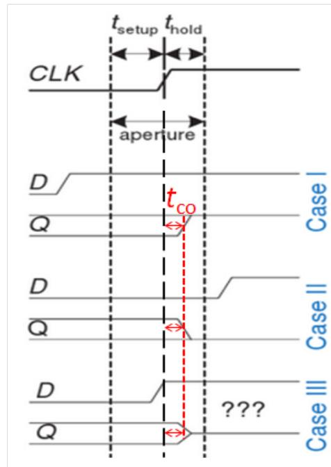
Figure 3–7: Three different cases in which D input signal is stable [26].
