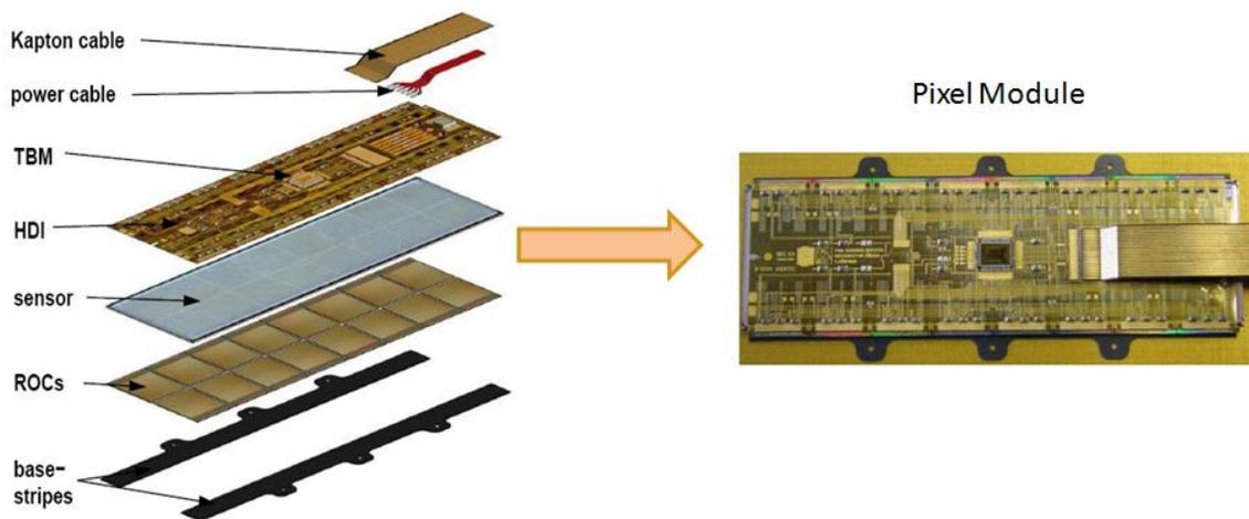
Figure 2–3: Components and view of the pixel module [14].
