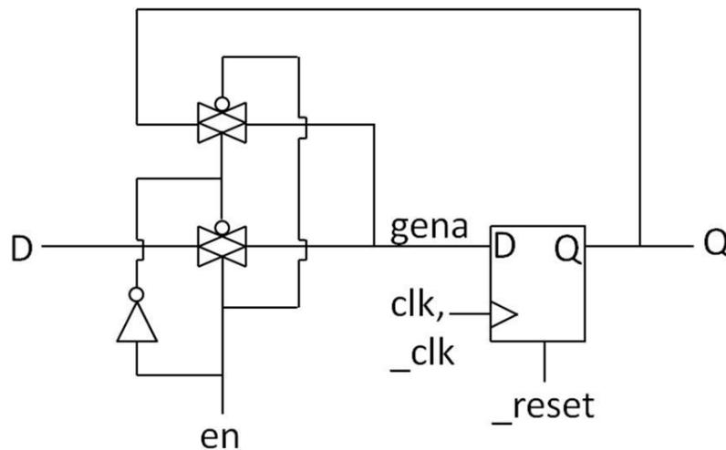
Figure 5–9: Two transmission gates interconnect between them and join to a D flip-flop with a \_reset input to make up the block 3 design.
