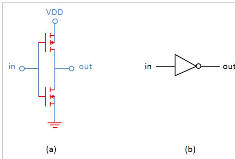
Figure 3–2: Inverter circuit on CMOS technology (a) and symbol (b) [24].
