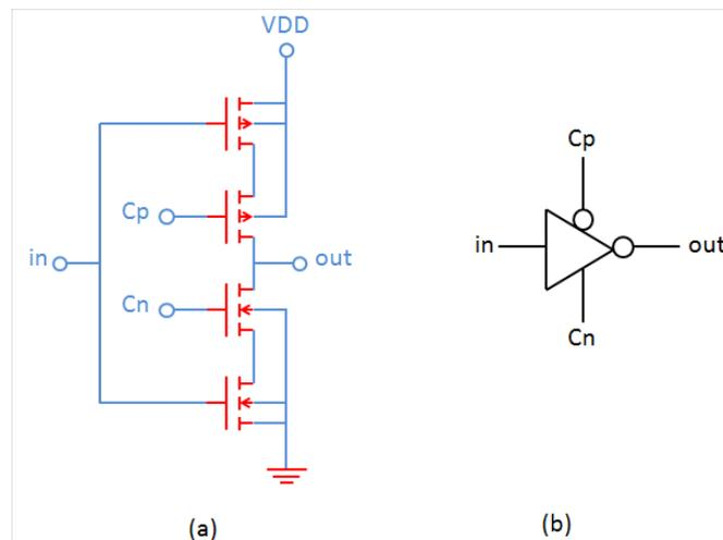
Figure 3-5: Tri state inverter buffer on CMOS technology built with two NMOS and two PMOS are connected in series (a), and symbol (b).
