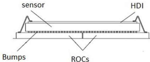
Figure 2–8: Transverse view of the assembly scheme of the module.
