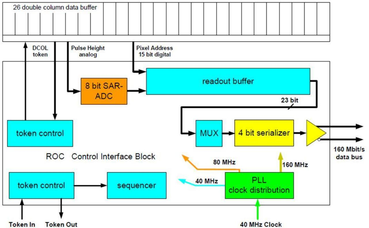
Figure 2–12: New components of the control interface block [13].
