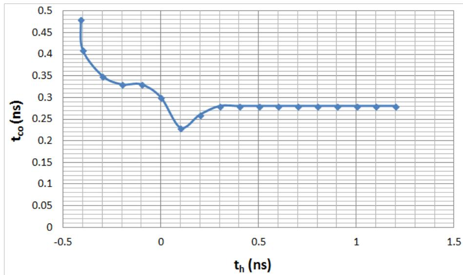
Figure 5-12:  $t_{co}$  values for different  $t_h$  values with 1.5 ns of  $t_{su}$ .
