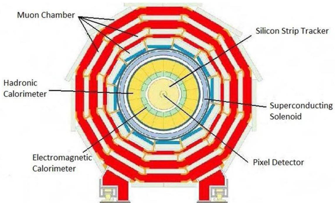
Figure 1–2: Transverse cross-section of the CMS detector [8].
