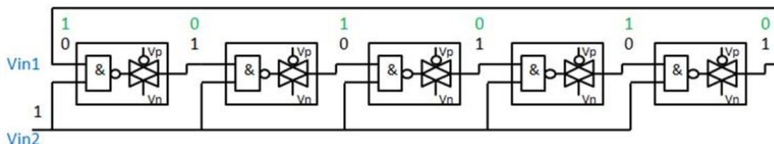
Figure 4-1: The VCO scheme to be used in new ROC design.
