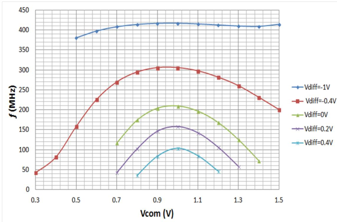
Figure 4-3: The VCO frequencies for different  $V_{diff}$  and  $V_{com}$  values, when  $V_{DD} = 2$  V.
