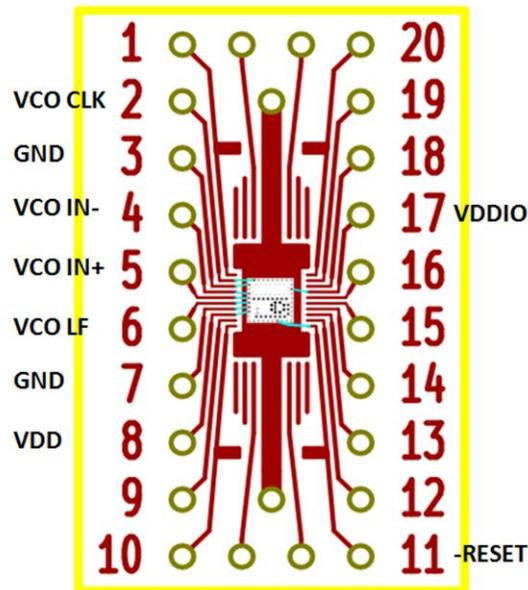
Figure 4–6: Sketch of PSI\_CDG001 connected to board. (Board drawn by Silvan Streuli, PSI).
