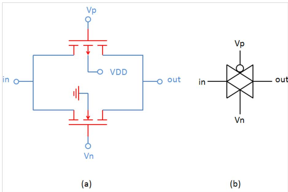
Figure 3–4: Transmission gate on CMOS technology using a NMOS and a PMOS transistors (a), and symbol (b).
