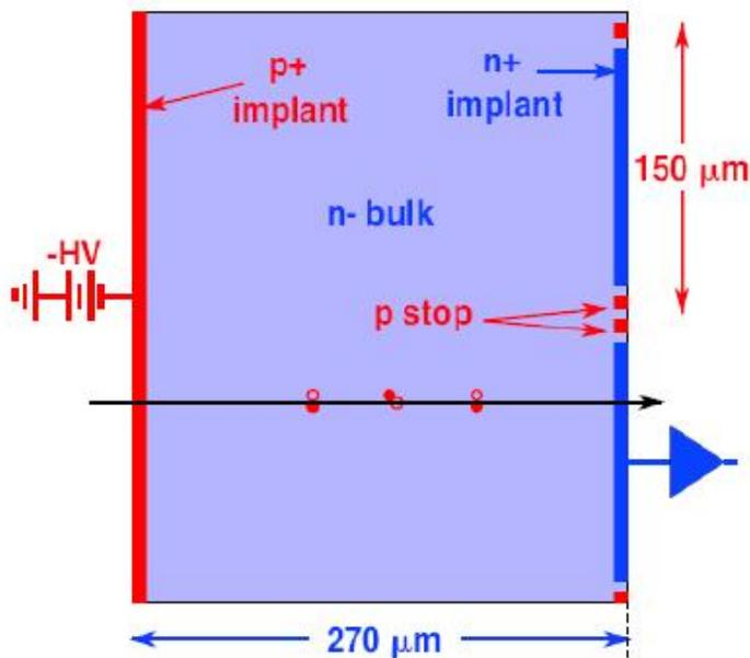
Figure 2-4: Structure of a pixel sensor [15].
