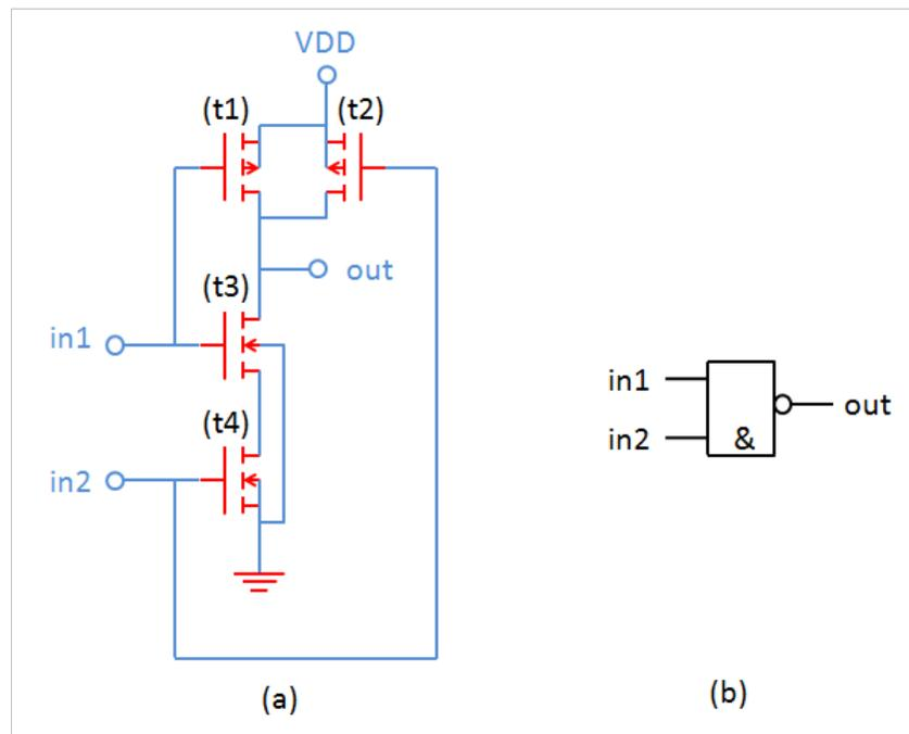
Figure 3–3: NAND gate on CMOS technology using two PMOS in parallel connection (t1 and t2), and two NMOS in serie (t3 and t4) (a); and symbol (b) [24].
