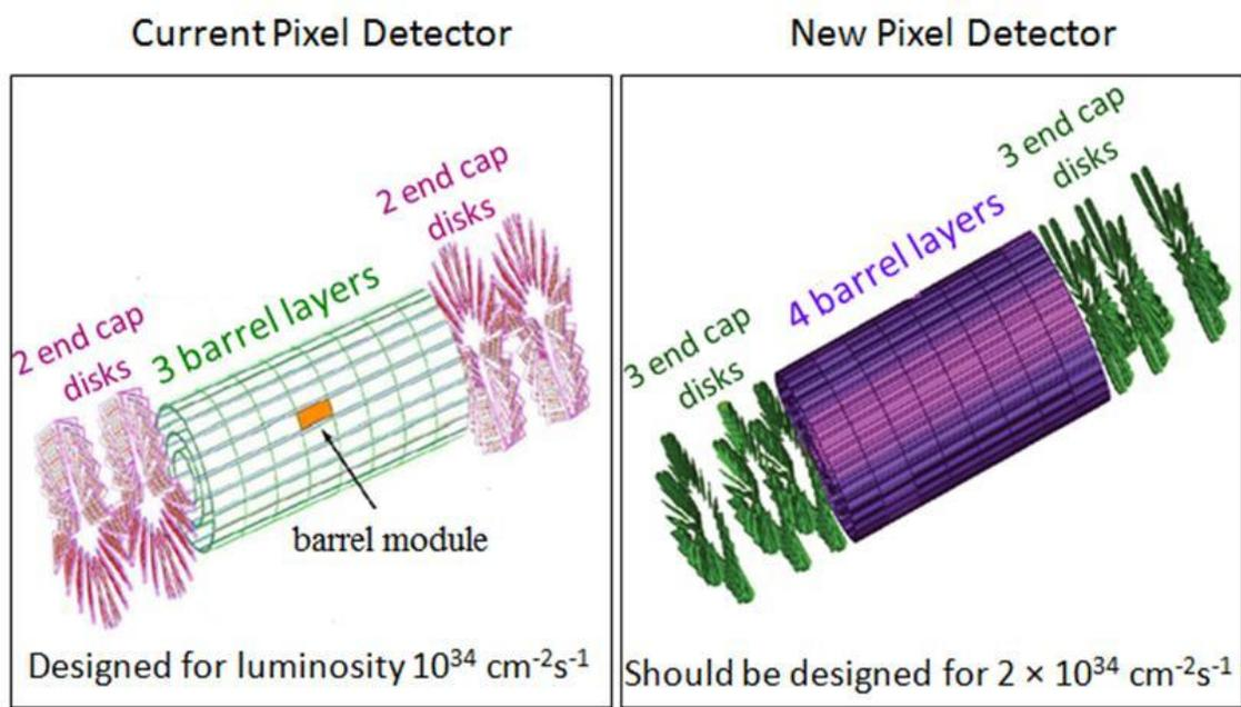
Figure 1–3: Current pixel detector and a new design for the pixel detector upgrade [7, 10].
