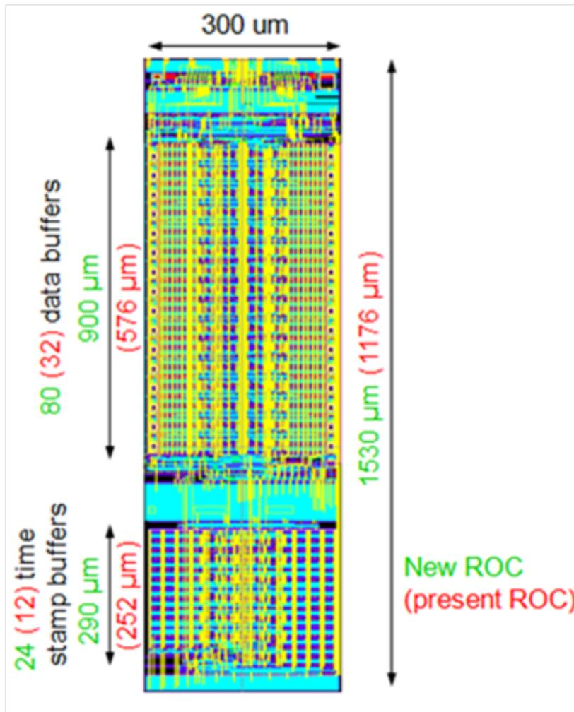
Figure 2–10: One of the twenty six Double Column Interface with size and number of buffers, for current (red) and new (green) ROC. interface [18].
