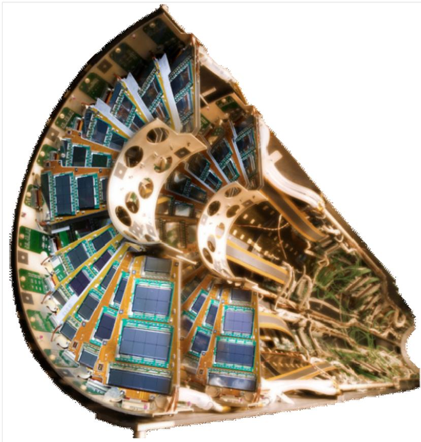
Figure 2-2: Half disks of the forward pixel detector in the FPIX service cylinder [13].
