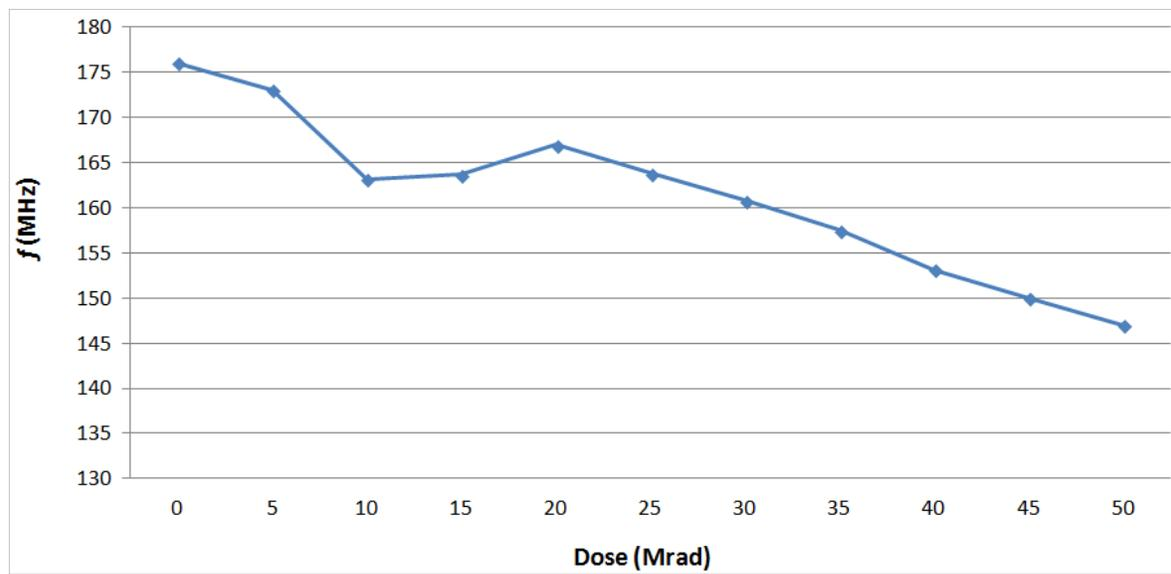
Figure 4–12: Average operation frequency for 3 irradiated test chips ( $V_{DD} = 2$  V,  $V_{com} = 1$  V,  $V_{diff} = 0$  V).
