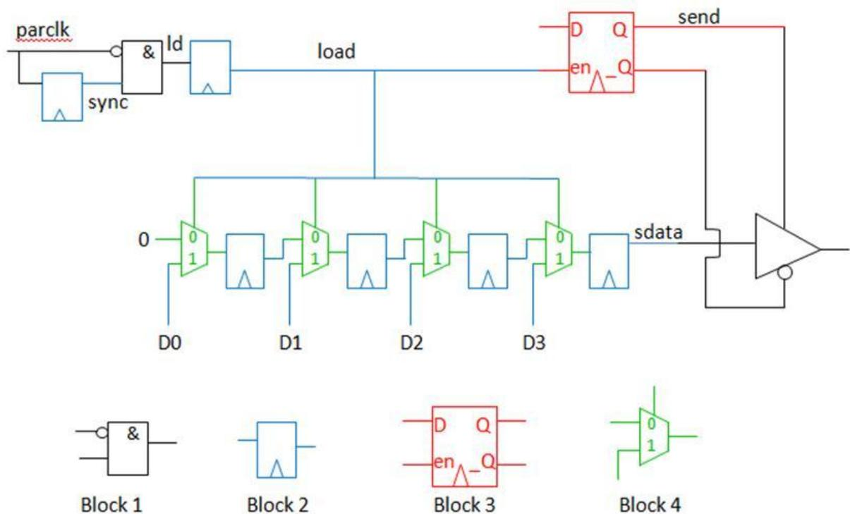
Figure 5–2: Serializer components. The triangles in the flip-flops are the serclk and \_serclk inputs.
