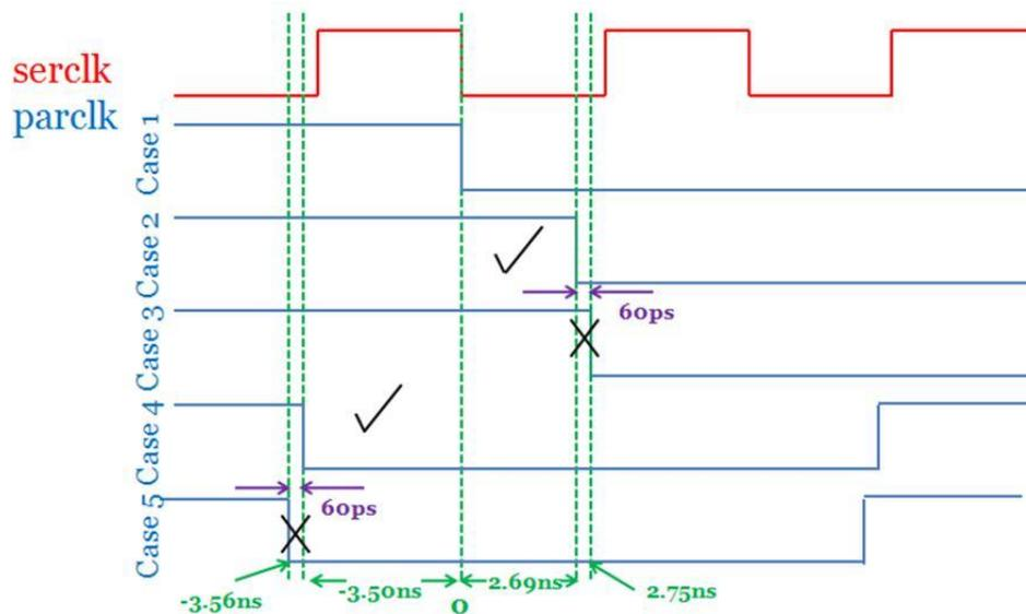
Figure 5–15: Intervals of the operation time for parclk signal in relation to serclk signal for their falling edge.
