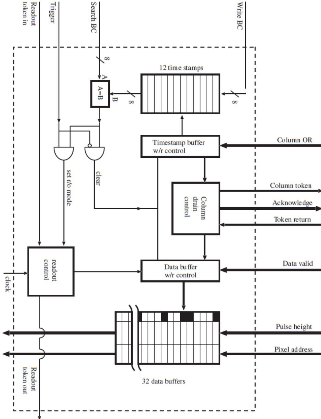
Figure 2-7: Readout system of the double column interface Readout system of the pixel unit cell (PUC) [17].
