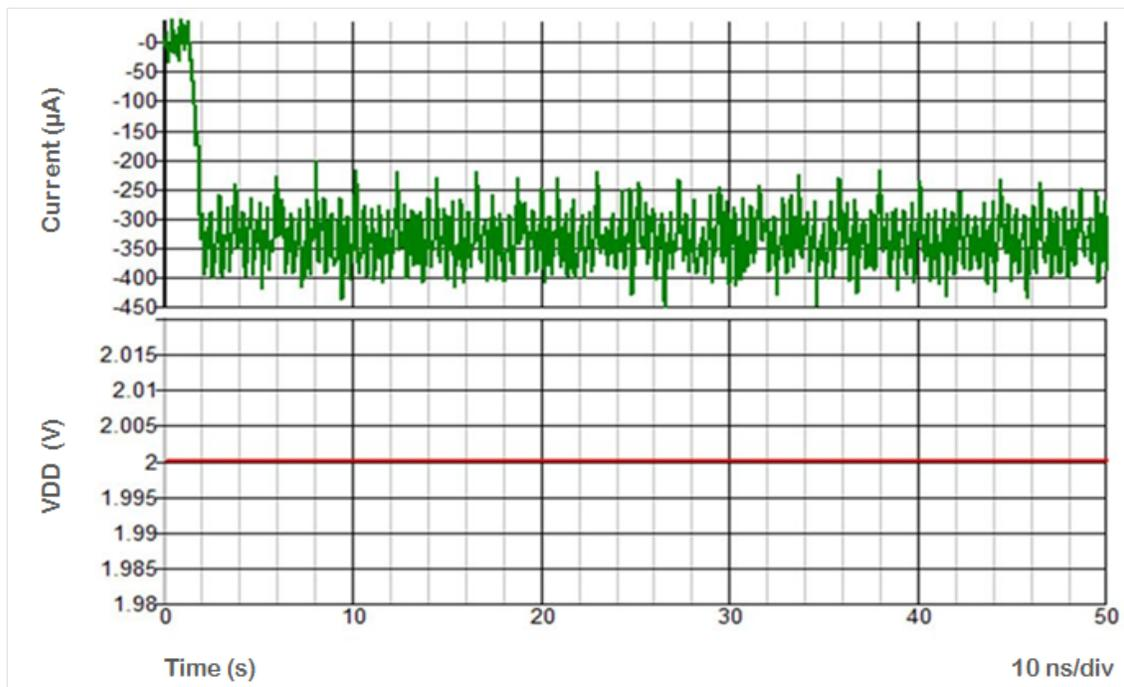
Figure 4-7: Green plot shows the current between source and VCO for a constant voltage represented by the red plot.
