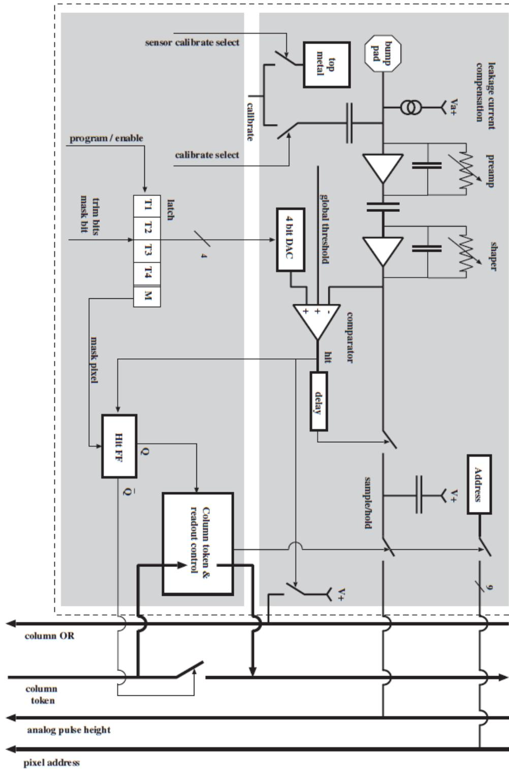
Figure 2-6: Readout system of the pixel unit cell (PUC) [17].
