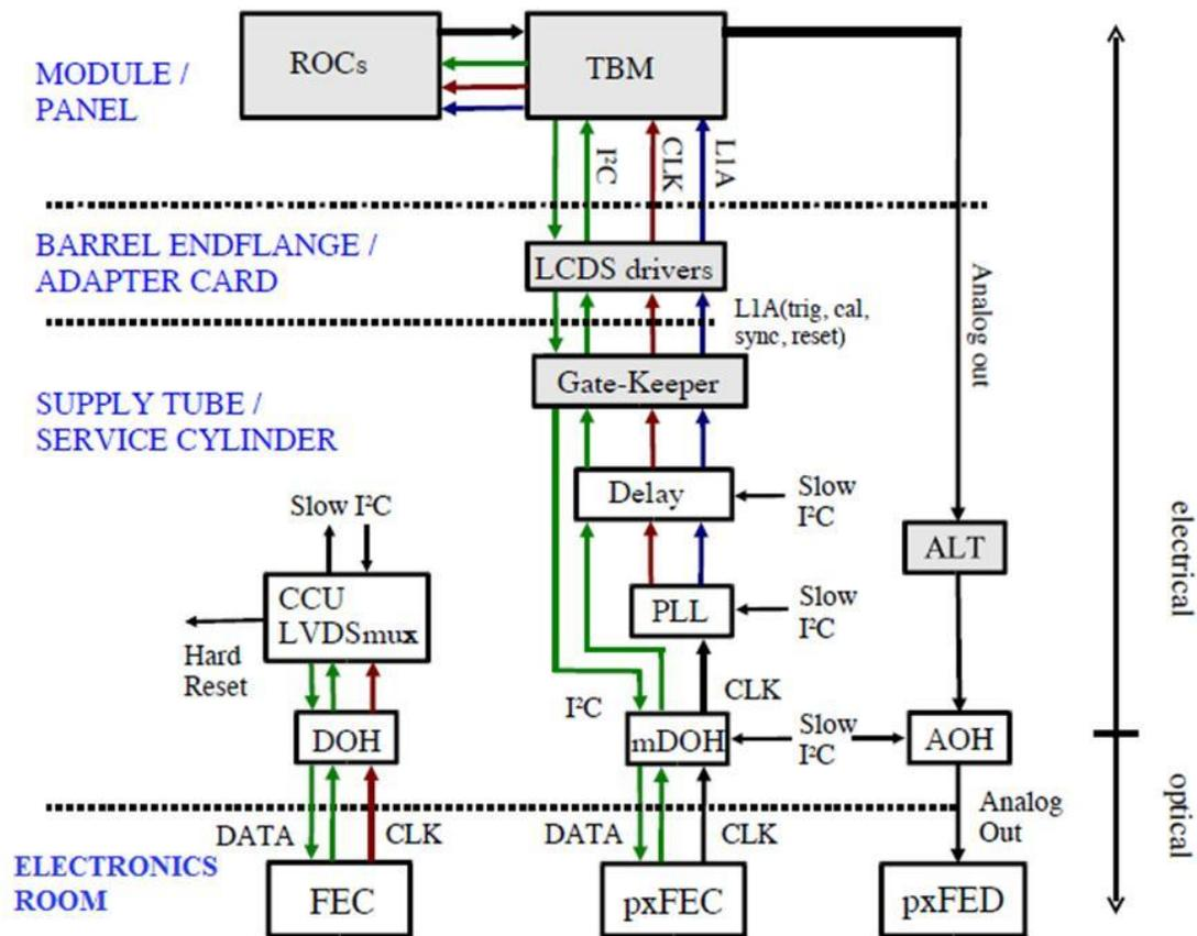
Figure 2–9: External readout of the pixel detector [3].
