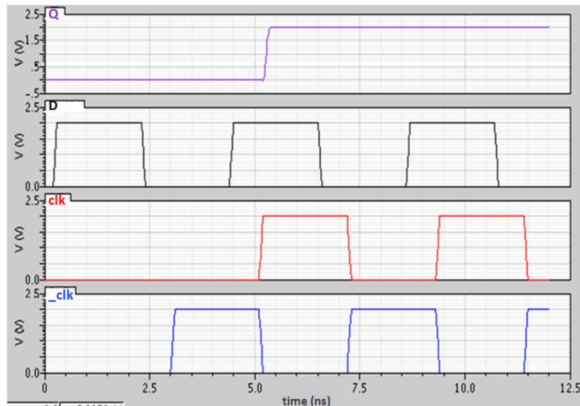
Figure 5–6: Output (Q), Input (D), Clock, and \_Clock, and signals for dff design.
