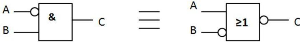
Figure 5-3: Two equivalent gates for the first serializer block.
