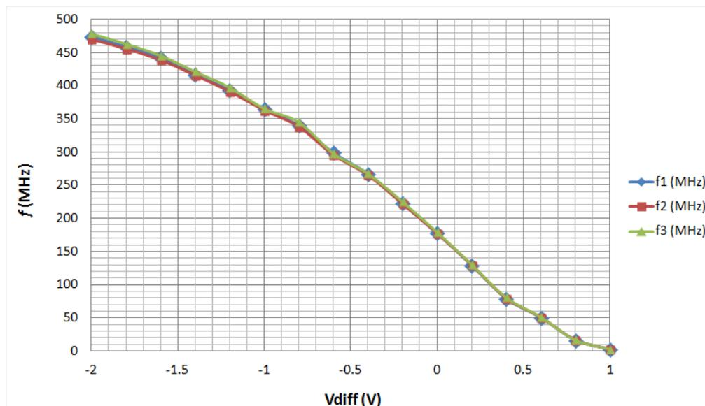
Figure 4-11: Frequencies in unirradiated chips for  $V_{com} = 1$  V and  $V_{DD} = 2$  V.
