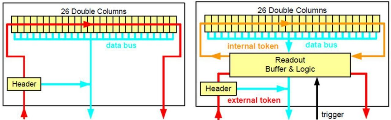
Figure 2–11: Present readout of the double column interface (left) and readout schema of the Double columns with a new buffer (right) [19].
