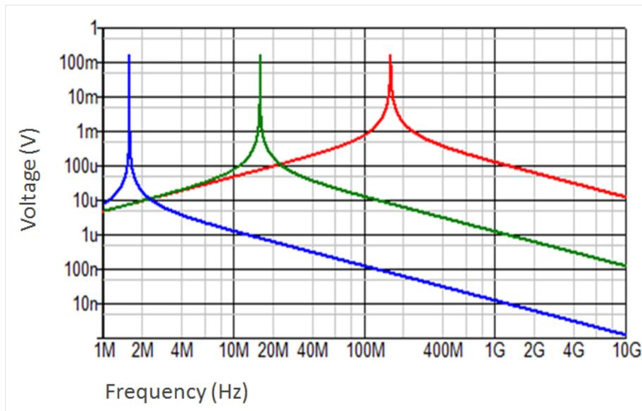
Figure 4–9: Voltage fluctuations as a function of frequency for a cable with 10 nH inductance. Each curve is for a connecting a different size capacitor in parallel. 100 pF (red), 10 nF (green), 1 F (blue).
