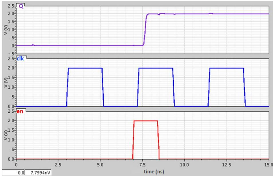
Figure 5–10: Enable (en), clock, and output (Q) signals for block 3.
