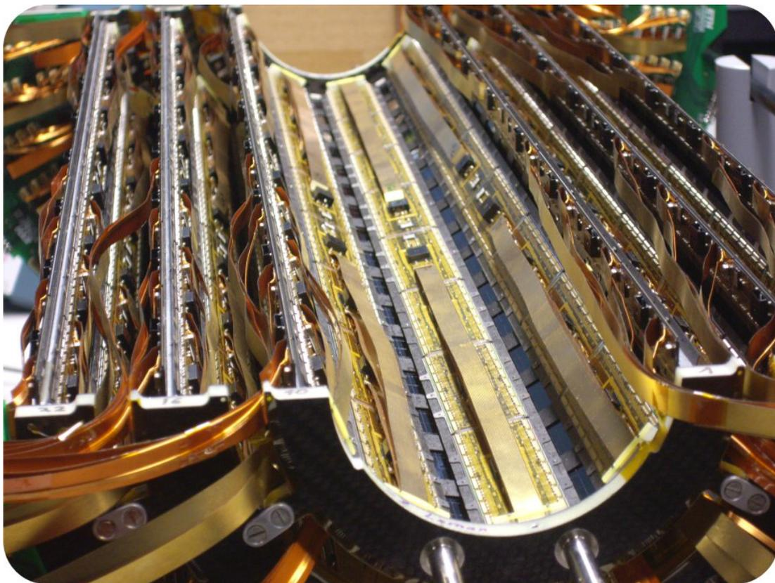
Figure 2-1: Barrel pixel detector half shells filled with 360 modules [12].
