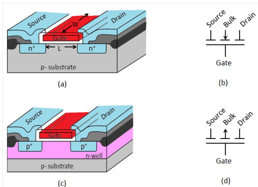
Figure 3-1: Cross-section view of an NMOS (a) and PMOS (c). MOS device symbol for NMOS (b) and PMOS (d) [22, 23].
