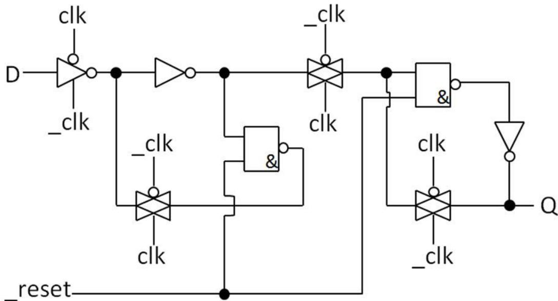
Figure 5-5: D flip-flop design with a `_reset` input called.
