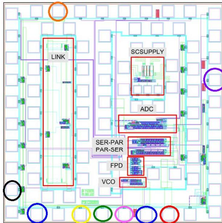
Figure 4-5: PSLCDG001 chip scheme with different circuit to be tested including the VCO, designed in PSI.
