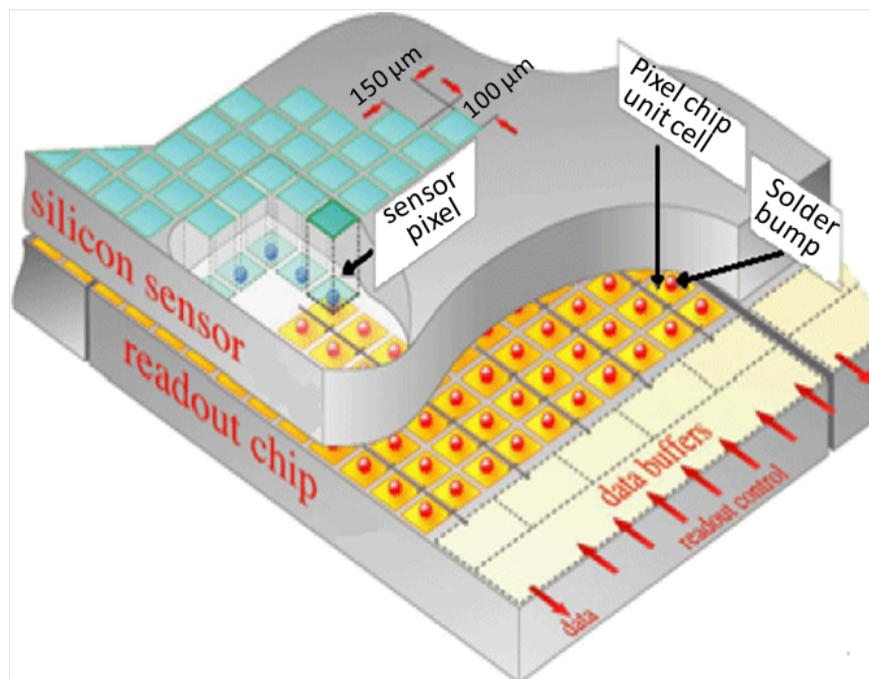
Figure 2–5: Schematic of the pixel sensors connected to the readout chip (ROC) by indium bumps [16].
