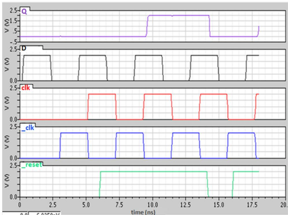
Figure 5–7: Output (Q) Input (D), Clock, \_Clock and \_Reset signals for dffr design.
