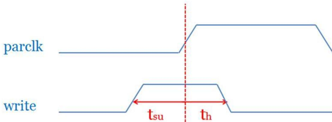
Figure 5–16: Write signal time parameters with respect to the parclk signal rising edge.
