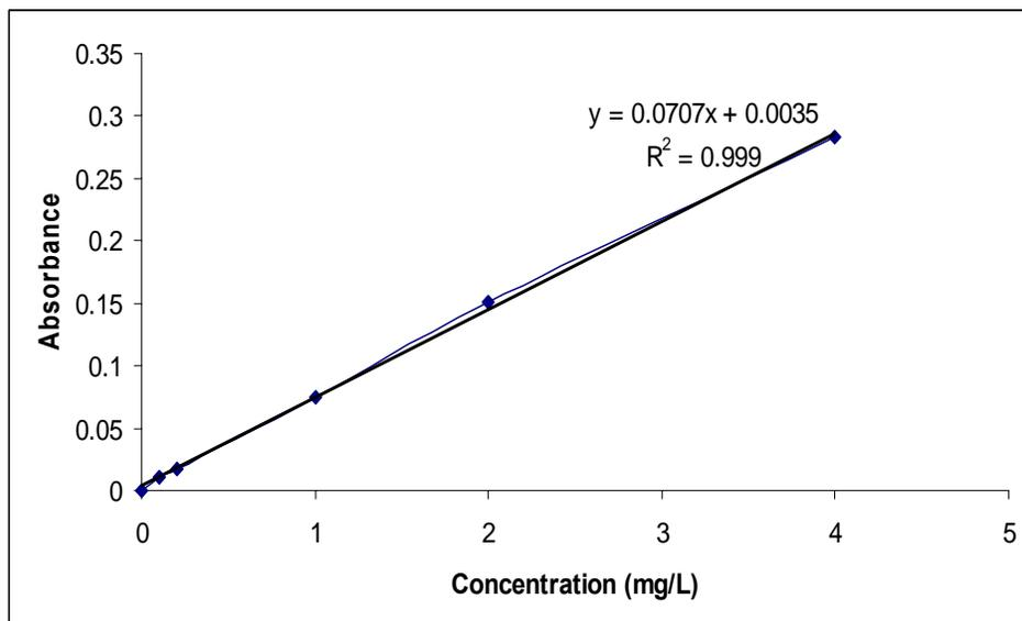
**Figure 5. Example of a calibration curve obtained during FAAS optimization**
