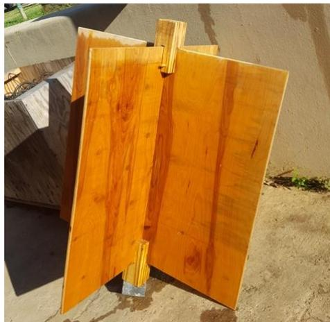
Fig. 3.4 ECO drifter prototype after its first buoyancy trial run at CAOSE hydrostatic tank.
