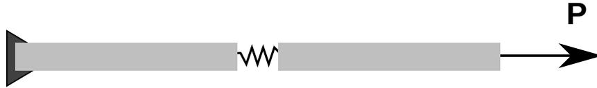
Figure 3.8: 1D Set Spring Elements with Cohesive Crack using XFEM
