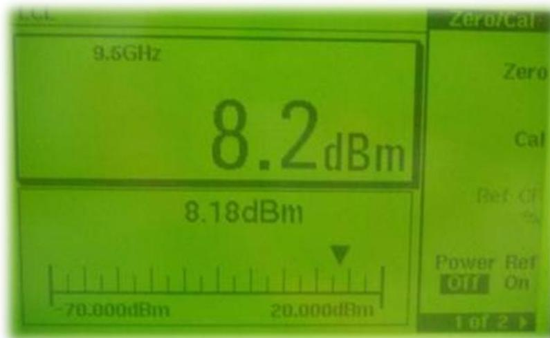
**Figure 4-35 21dB Power Amplifier output with a 13dB input signal to the transmitter**
