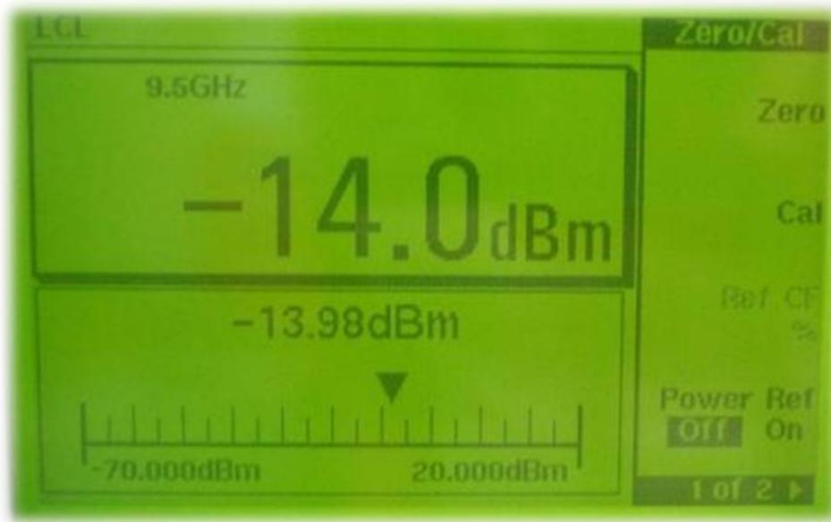
**Figure 4-30 Mixer HMC521LC4 output with 13dBm transmitter input.**
