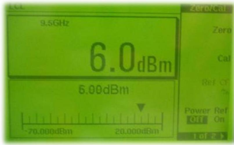
**Figure 4-36 21dB Power Amplifier output with 5dB input signal to the transmitter.**
