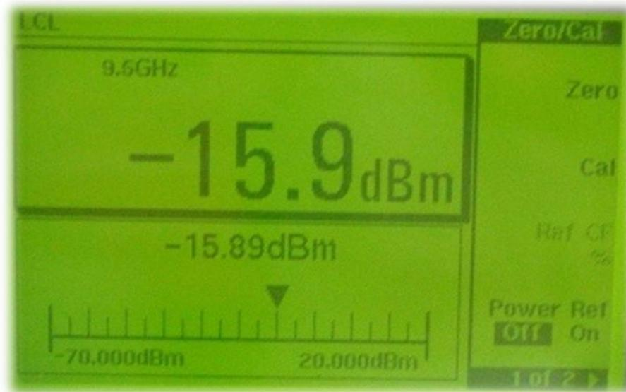
**Figure 4-31 Mixer HMC521LC4 output with 5dBm transmitter input.**
