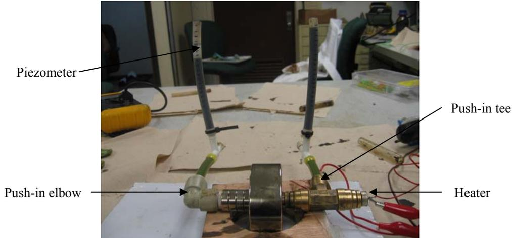
**Figure 31: Magnetocaloric pump working with the Mn-Zn produced ferrofluid**
