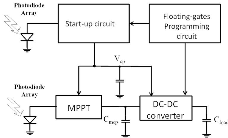
Figure 1.1 : Block diagram of the proposed energy harvesting system
