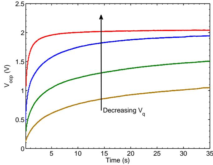
Figure 3.10 : Output voltage of the charge pump for different values of  $V_q$  with an input voltage of 0.4V.
