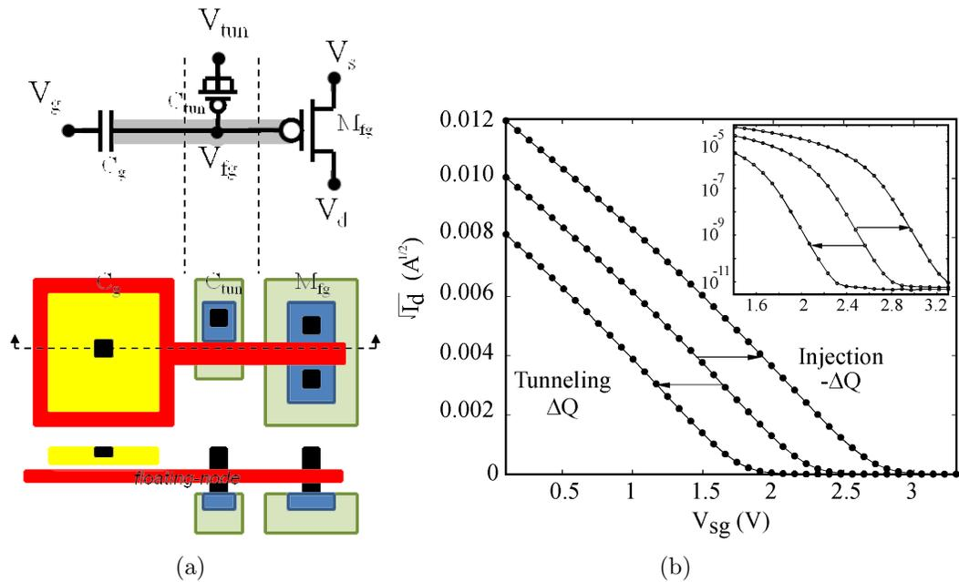
Figure 2.3 : Floating-gate Transistor: (a) Circuit schematic and layout of a floating-gate PMOS transistor. (b) Threshold variation of a PMOS floating-gate.
