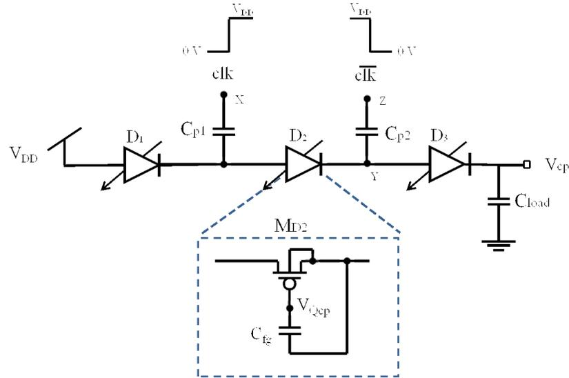
Figure 3.9 : Three stage charge pump with floating-gate diode-connected transistors.
