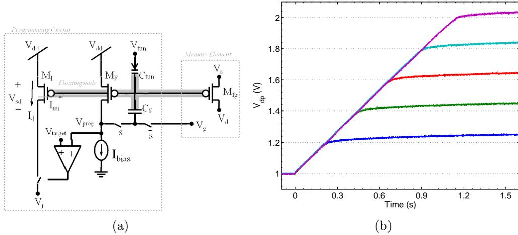
Figure 2.4 : (a) Schematic representation of a single programming unit (PU). (b) Programming of a single PU for different voltages at maximum injection rate.
