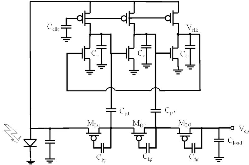
Figure 3.16 : Schematic of a 3-stage representation the proposed start-up circuit.
