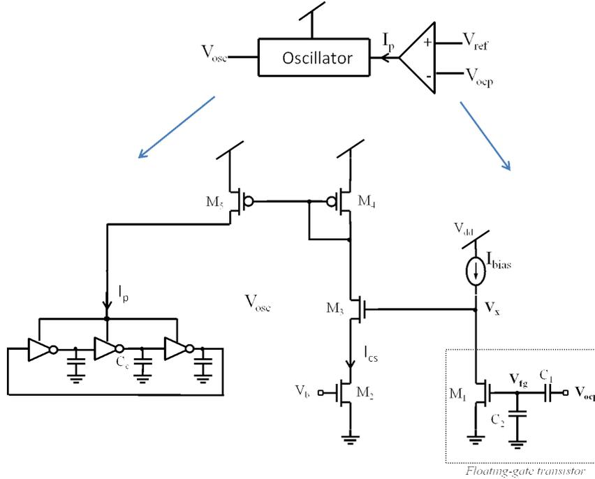
Figure 3.7 : Main oscillator feedback circuit
