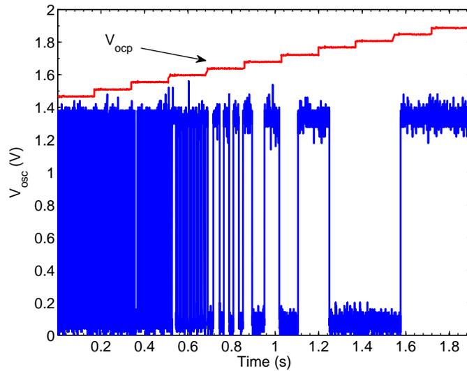
Figure 3.8 : Frequency variation change with a sweep of  $V_{ocp}$  in the feedback circuit.
