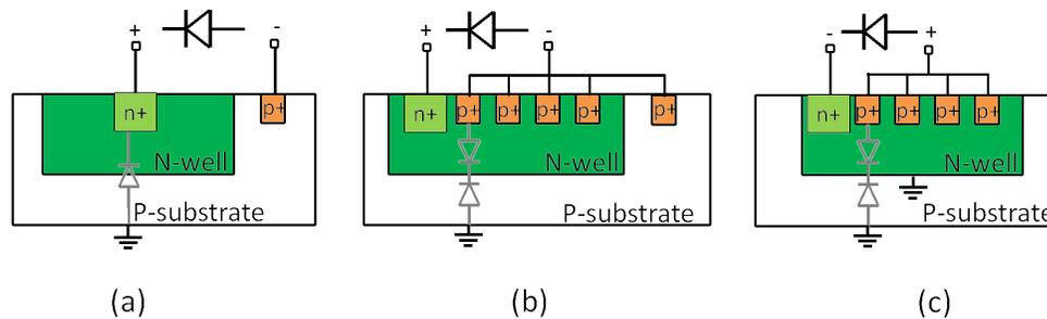
Figure 2.1 : Cross section view of the integrated photodiodes and the types of connections available in a standard CMOS process: (a) n-well/substrate, (b) n-well/p-diff/substrate, (c) n-well/p-diff
