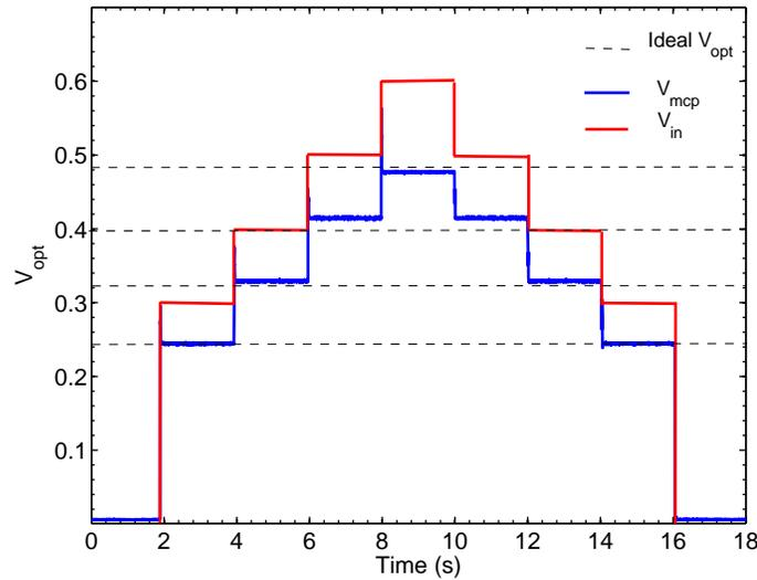
Figure 3.5 : Measured output of the MPPT circuit for input values ranging from 0.3V to 0.6V.
