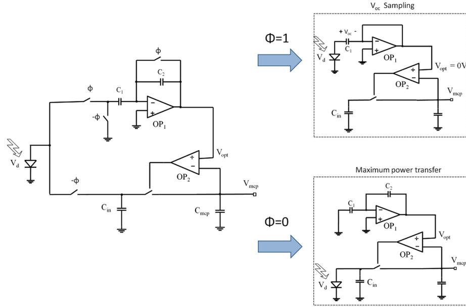
Figure 3.4 : Schematic of the MPPT scheme and the equivalent circuits during the sample and hold cycles.
