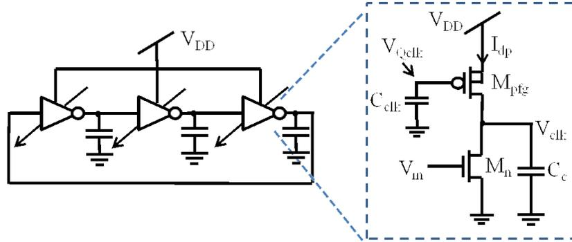
Figure 3.13 : Schematic of a 3-stage ring oscillator with floating-gate PMOS transistor.
