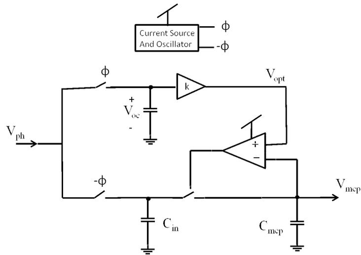
Figure 3.1 : Block diagram of Maximum Power Point Tracking circuit.
