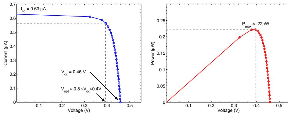
(a) Current and voltage graph of the photodiode.
