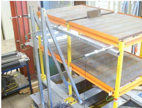
**Figure 4-10 View of the LVDTs**
