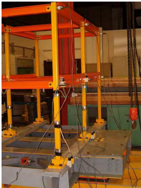
**Figure 4-2: Accelerometers layout**
