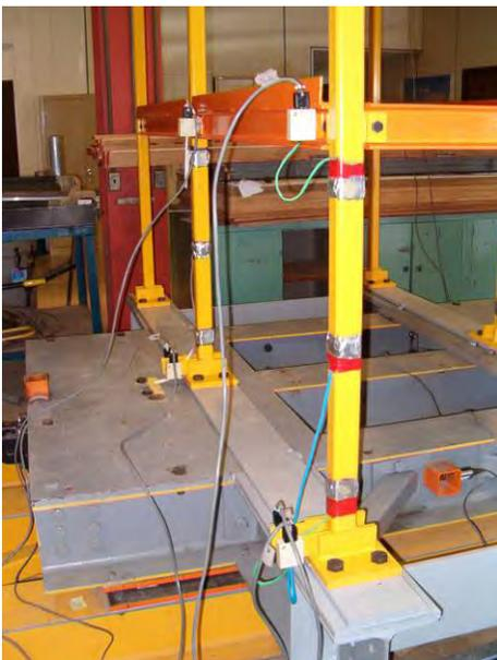
**Figure 4-3: View of the Load Cells in Column**
