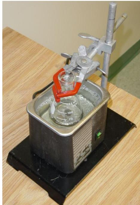
**Figure 3-3.** Ultrasonic cleaning process
