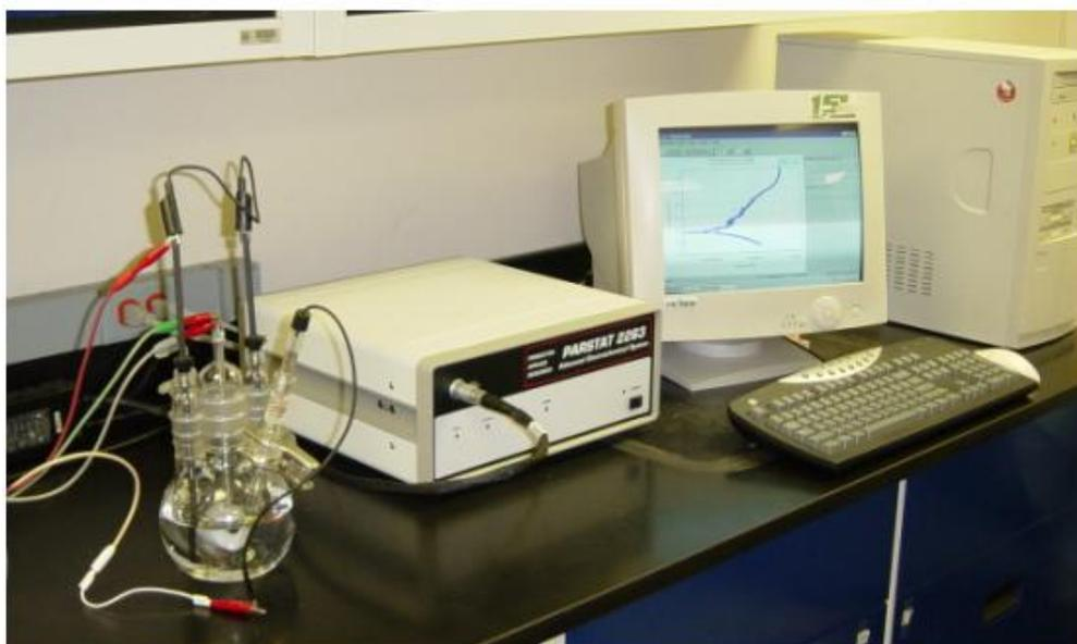
**Figure 3-6.** Experimental setup for corrosion measurements
