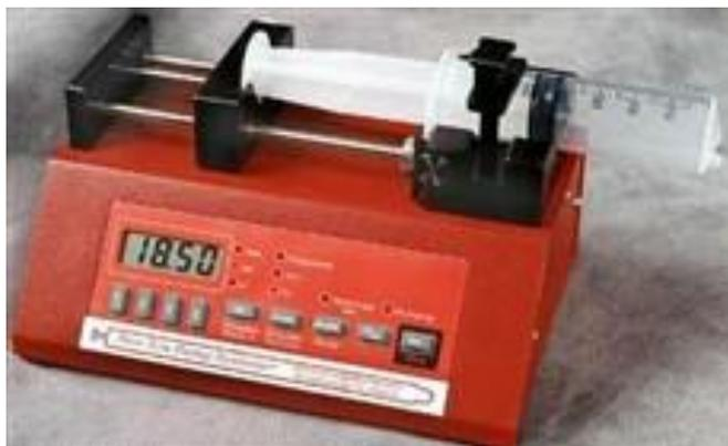
**Figure 4.2: New Era Syringe Pump model NE-1000 (photo courtesy of New Era Pump Systems, Inc.).**
