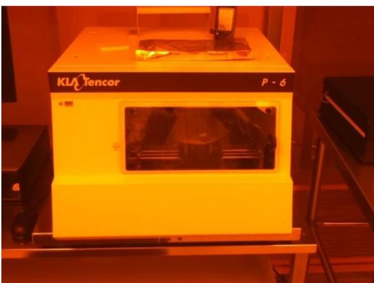
**Figure 3.9: KLA Tencor Stylus Profiler Model P-6.**
