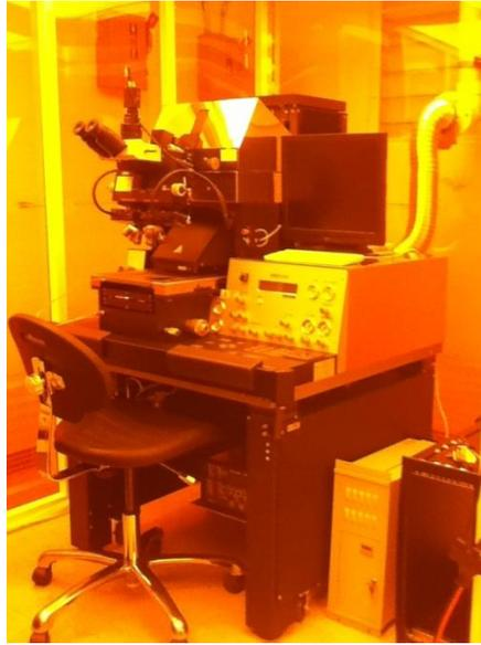
**Figure 3.8: SUSS MicroTec MA-6 Mask Aligner.**
