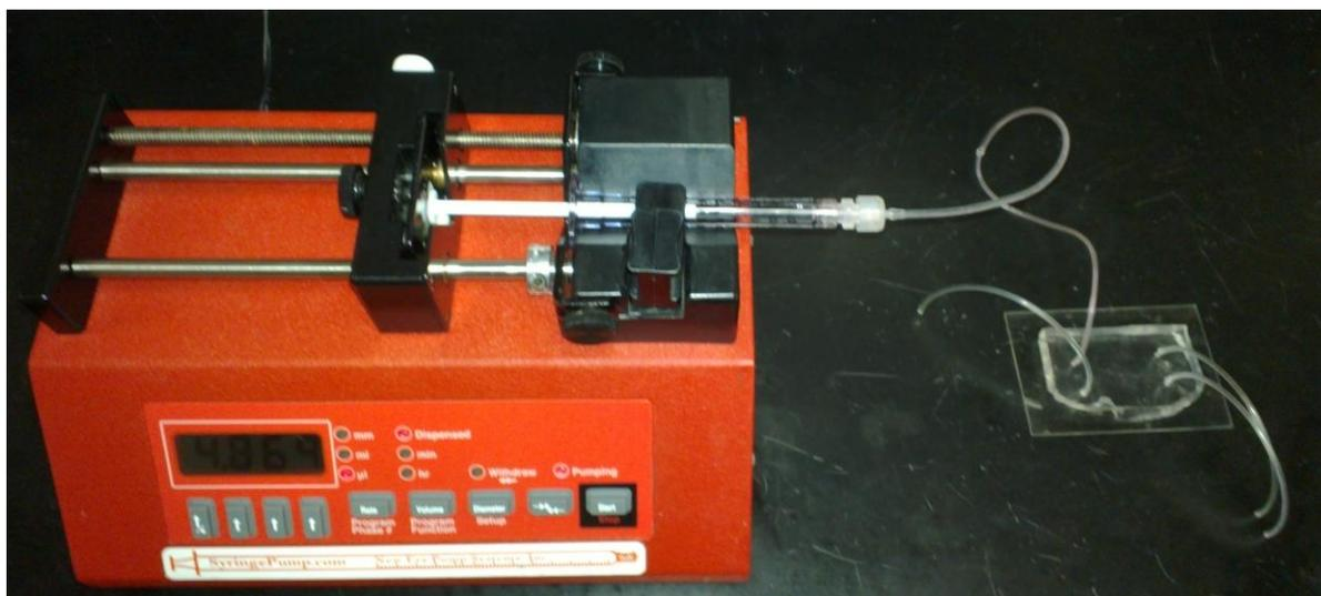
**Figure 3.122. PBS flushing of the micro-fluidic device.**
