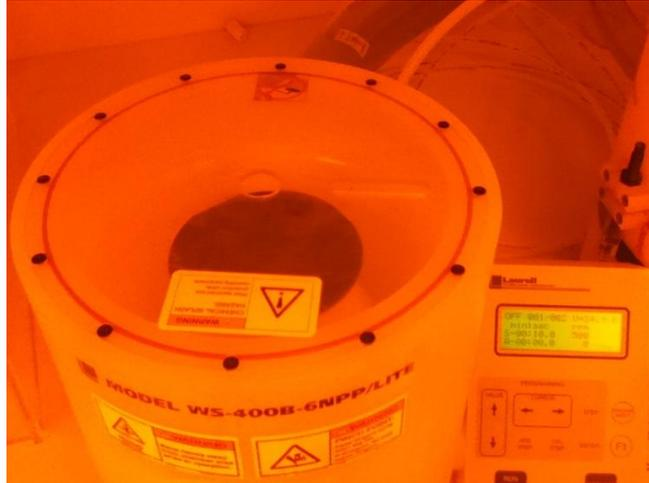
**Figure 3.7: Laurell Model WS-400B-6NPP/LITE spin coater.**
