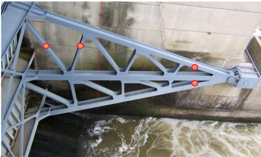
**Figure 29: Location of the transducers in the Carlyle Tainter Gate. Picture from the experimental procedure performed in Carlyle Lake Dam by Dr. Gopalaratnam and Dr. Riveros.**
