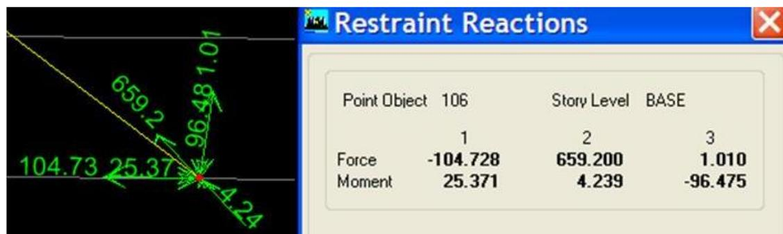
**Figure 24: Reaction in the pin due to dead and hydrostatic load, and cable pressure.**
