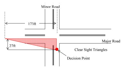
Figure 5-8 Intersection Sight Triangles for Right Turns from the Minor Road.
