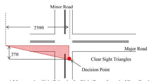
Figure 4-3 Intersection Sight Triangles for Right Turns from the Minor Road.
