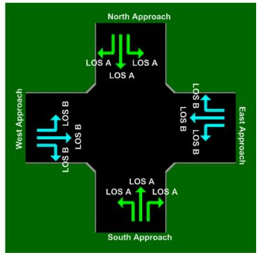
Figure 6-17 Level of Service for Critical Gaps Found in the Field.
