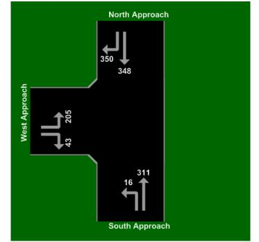
Figure 6-3 Input Volumes in the Three Leg (T) Intersection.
