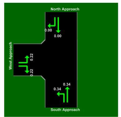
Figure 6-8 Queue Storage Ratio for Critical Gaps Found in the Field.
