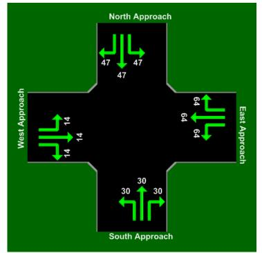
**Figure 6-12 Queue Distance for the Four Leg Intersection.**
