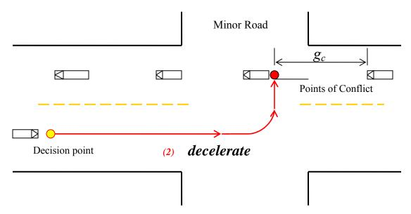
Figure 5-11(2) Vehicle Decelerates Until a Desirable Gap is Provided.
