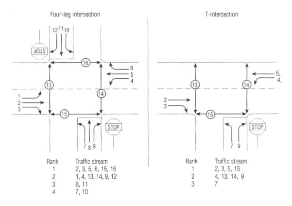
Figure 2-5 Intersection Priority Diagrams for a TWSC.
