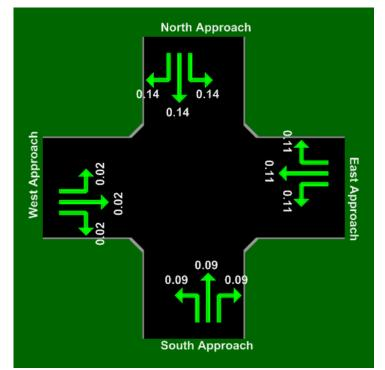
Figure 6-16 Queue Storage Ratio for Critical Gaps Found in the Field.
