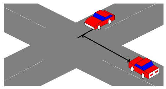
Figure 2-2 Lag Time Between Two Vehicles.
