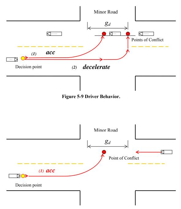
Figure 5-10 (1) Vehicle Accelerates and Enters the Intersection Aggressively.
