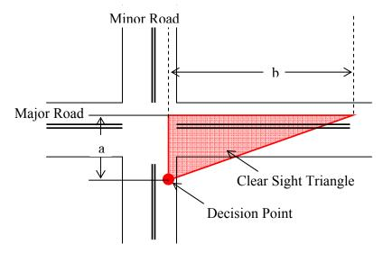
**Figure 4-1 Departure Sight Triangle for Left Turns.** Traffic approaching from the right
