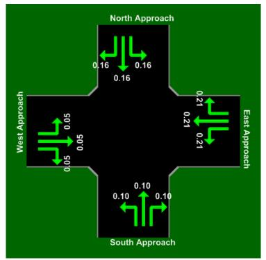
Figure 6-13 Queue Storage Ratio for the Four Leg Intersection.
