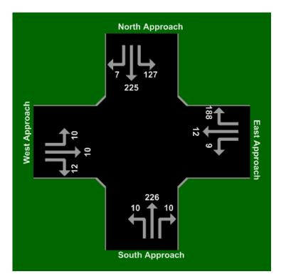
**Figure 6-11 Input Volumes in the Four Leg Intersection.**
