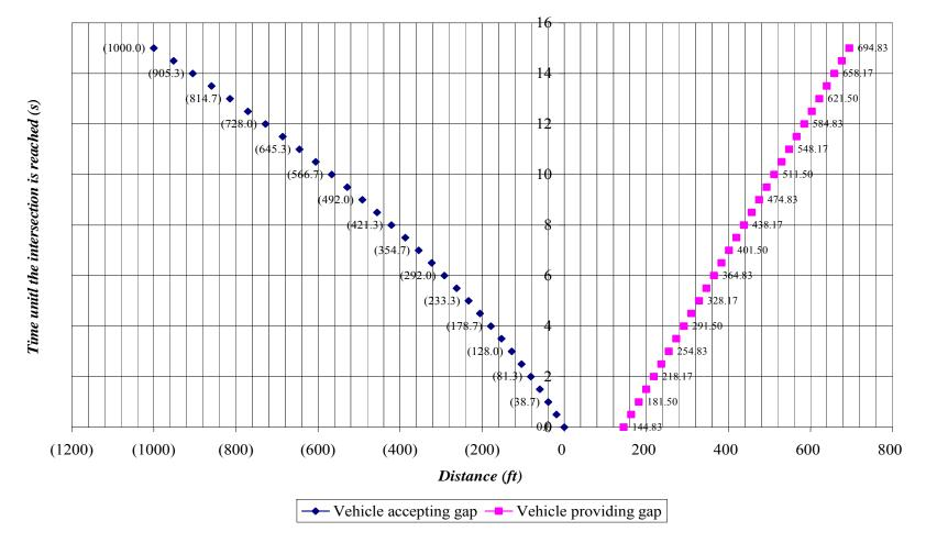
Figure 5-14 Distance traveled by vehicles approaching the intersection from opposing access stream for a Critical Gap of 3.95s
