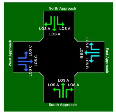
**Figure 6-14 Level of Service for the Four Leg Intersection.**
