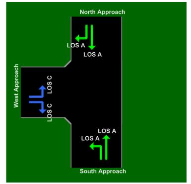
Figure 6-9 Level of Service for Critical Gaps Found in the Field.
