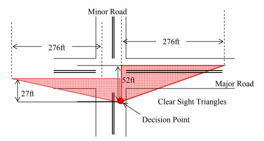
Figure 4-2 Intersection Sight Triangles for Left Turns from the Minor Road.
