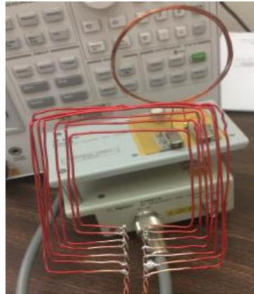
**Fig A.0.4 Parallel square shape antenna configuration**
