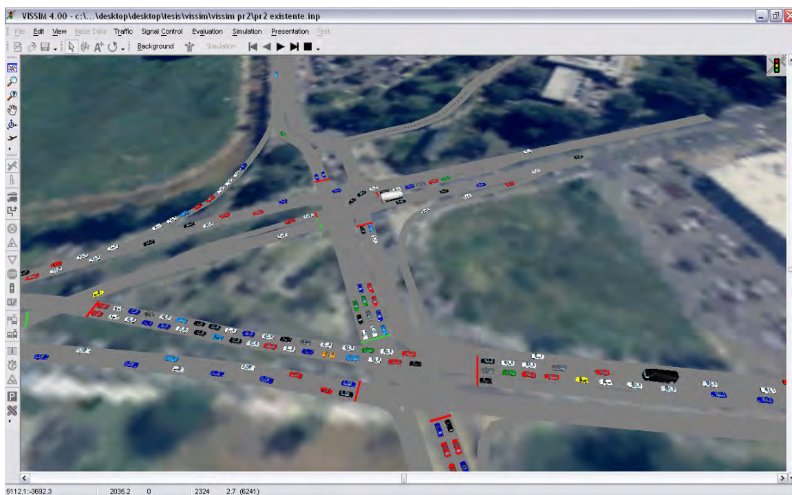
Figure 6.8 Spill back simulation at intersections
