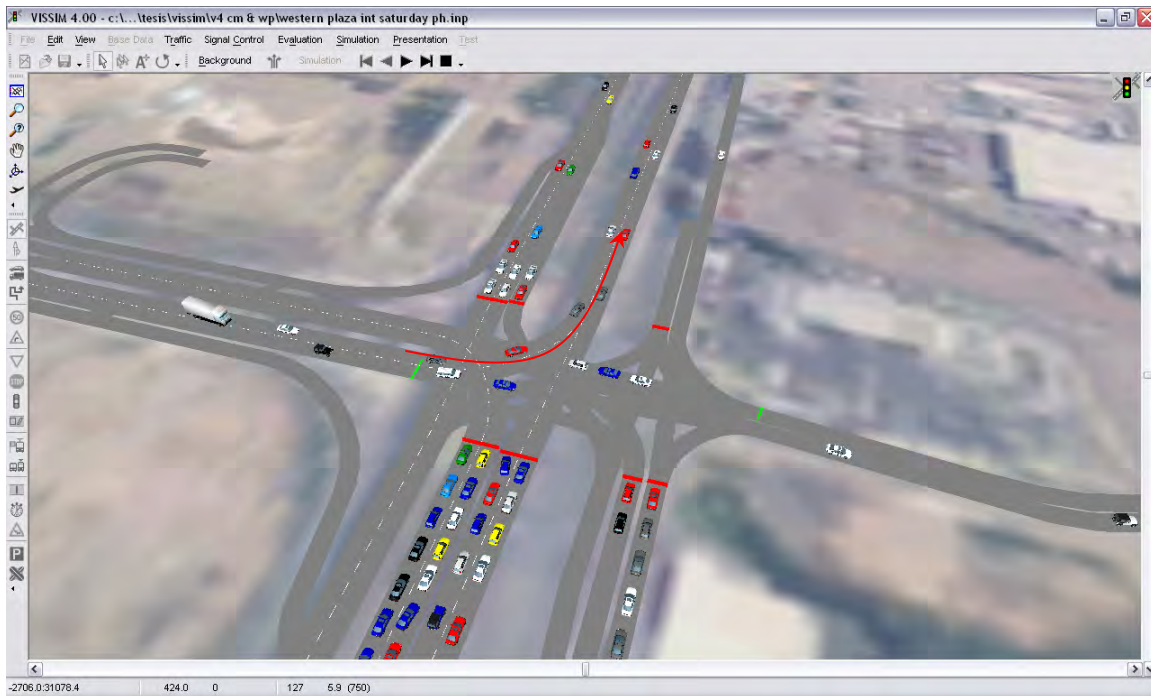
Figure 6.6 Left turn movements priority from straight movements
