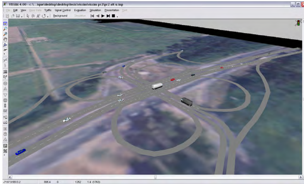
Figure 4.11 Example of a clover leaf intersection for the PR-2 network at the PR-109 and PR-115
