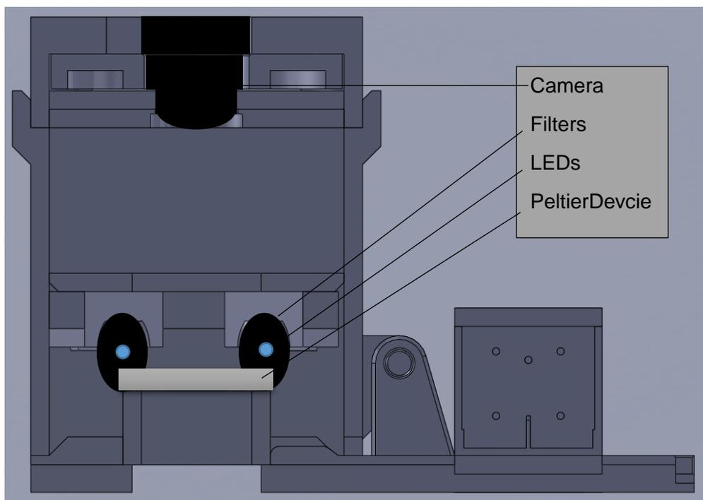
Figure 18: Device Cross-section Arrangement
