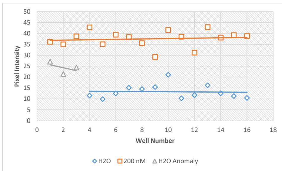
A clear difference is observed between the 200 nM chip and the H<sub>2</sub>O control. Fluorescence is observable using the software analysis method hence the device can function without the emission filter as the 200 nM sample gives over twice the pixel intensity as the water.
