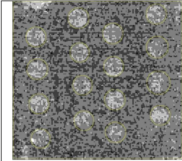
The entire chip is selected using a square section and each well is excluded from the selection. The areas excluded are slightly larger than the wells in order to eliminate the well edges to ensure a clear measurement.
