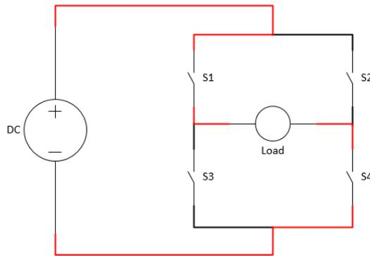
Figure 13: H-Bridge Enabling S1 and S4. Enabling S1 and S4 causes the current to flow from the left side of the load to the right.
