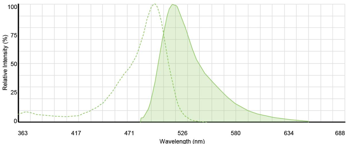
Figure 10: 6-Fam Excitation and Emission curves.
