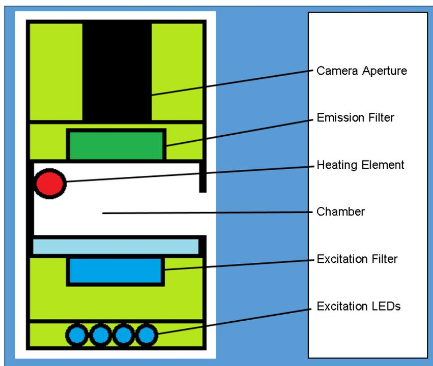
*Figure 5: Sketch of Weibel Lab's initial device design.*
