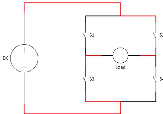
Figure 14: H-Bridge Enabling S2 and S3 Enabling the S2 and S3 switches allows the current to flow from right to left on the motor.
