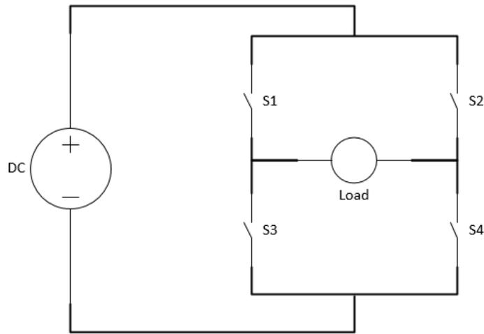
Figure 12: Basic H-Bridge Diagram The H-bridge consists of 4 switches. Enabling the correct sequence of switches reverses the current flow through the load. Enabling S1 and S3 or S2 and S4 will create a short circuit.
