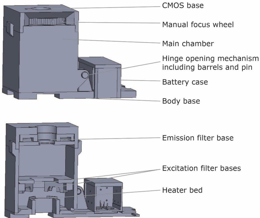
Figure 17: Final device design CAD and Cross-section
