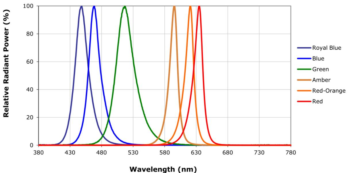
Figure 9: Emission spectrum for the Cree Xlamp XB-D LEDs. The closest peak to the desired wavelength corresponds to the Blue LED [24].
