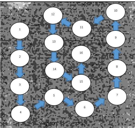
The selection and measurement is repeated for each well in a counterclockwise spiral order. This groups the more outer wells from 1 to 12 and the inner wells from 13 to 16.
