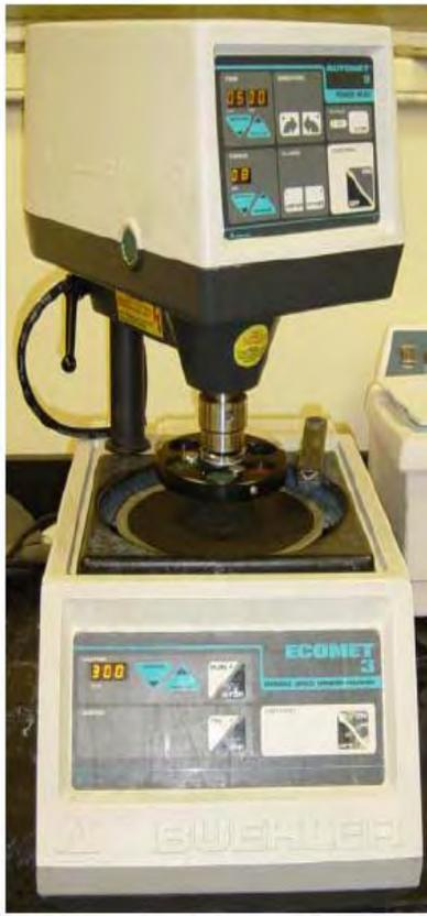
Figure 2.5 Mechanical grinding and polishing machine
