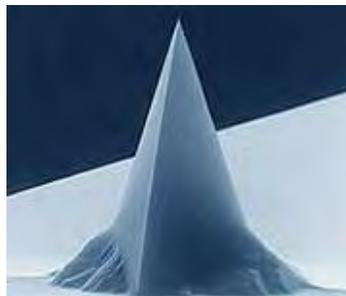
Figure 2.2 Schematic AFM contact mode probe [16]
