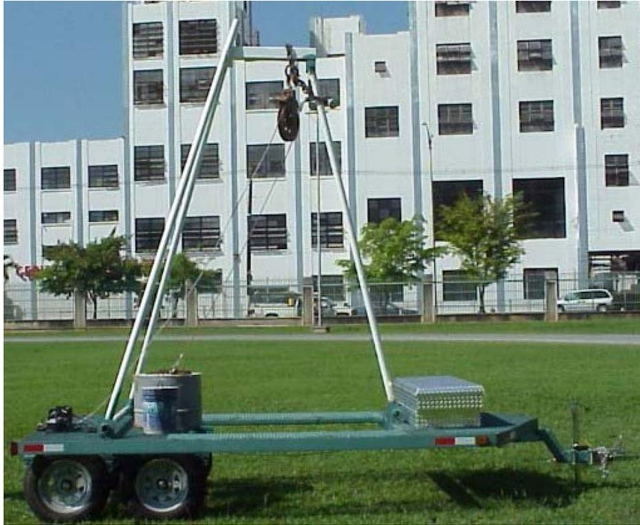
Figure 3.2: Weight drop system constructed at UPR-Mayagüez CE Department.
