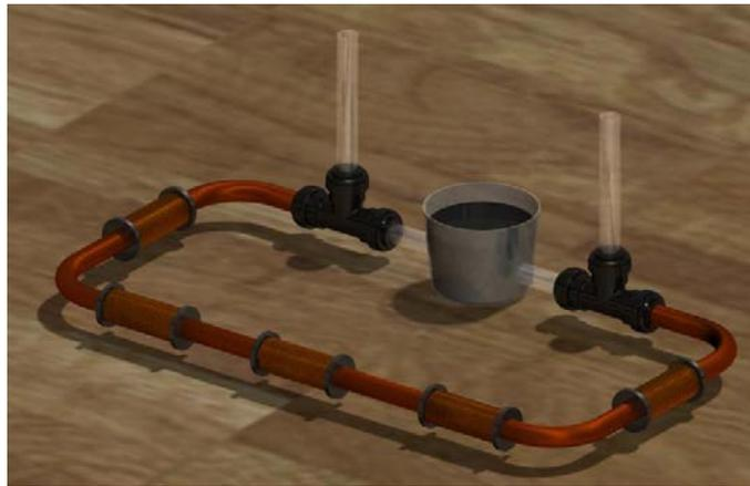
Figure 1-1: Device prototype, arrangement of the solenoids around the loop
