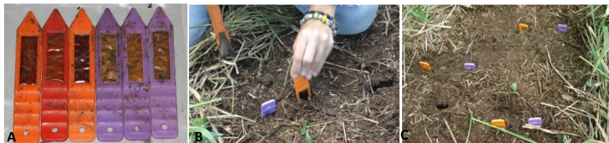
Fig. 1.2 Example of PRS TM -Probes samples and installation in field. (A) Three anion (orange) and three cation (purple) probes. (B) Probe installation and (C) probes installed at field.
