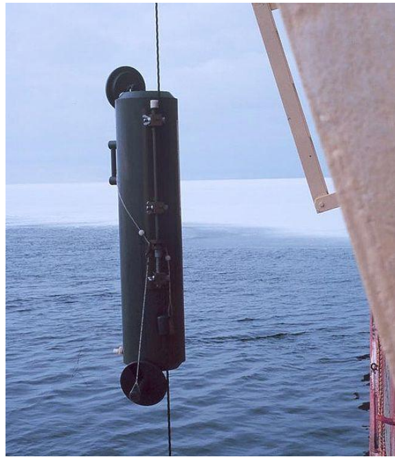
Figure 1.1. A Niskin bottle being deployed from the side of a boat.
