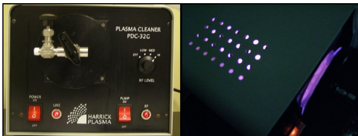
Figure 3-3. Plasma chamber (Harrick Plasma). The characteristic pink glow inside the chamber indicates that the plasma is working.
