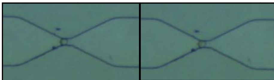
Figure 6-2. HeLa cell expansion of a cell experiencing a 10V pulse.
