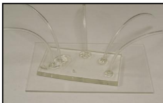
Figure 3-6. Picture of previous microchannel fabrication. Finished microchannel has Tygon tubing at the inlet/outlet ports.
