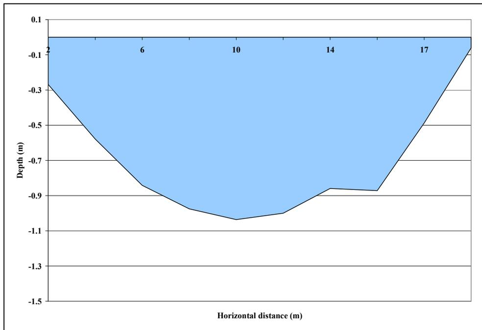
Figure 20. Río Grande de Arecibo cross section at grab sampling site.
