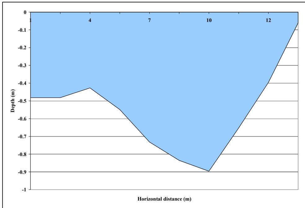
Figure 21. Río Caonillas cross section at grab sampling site.
