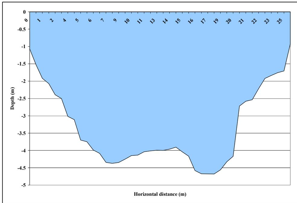
**Figure 17. Río Caonillas cross section at storm sampling site.**
