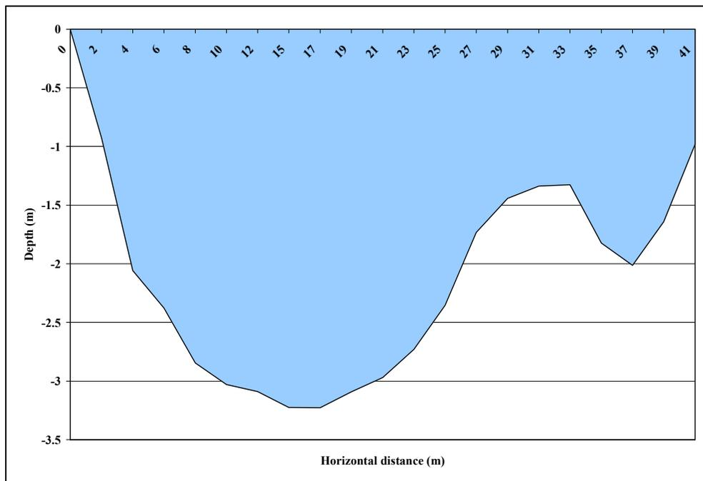
**Figure 16. Río Grande de Arecibo cross section at storm sampling site.**
