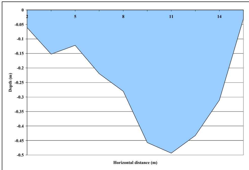
Figure 19. Río Limón cross section at grab sampling site.
