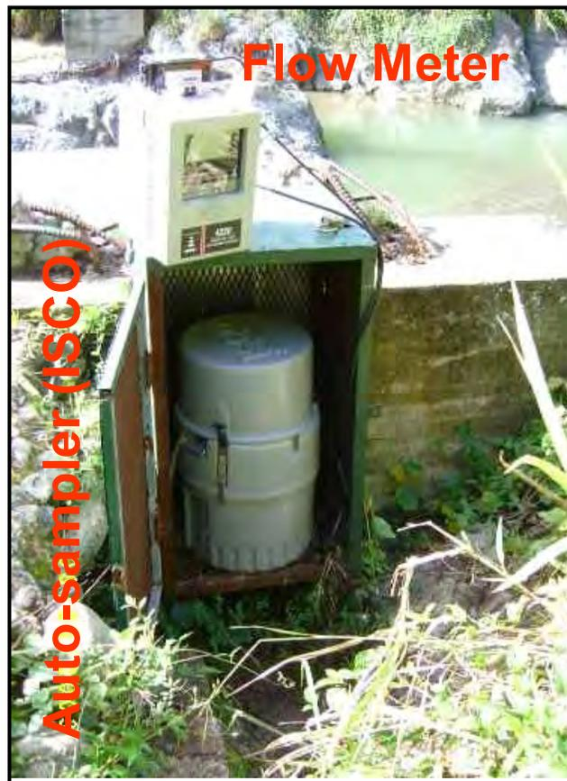
**Figure 9. ISCO - flow meter (4220) and auto sampler (3700).**
