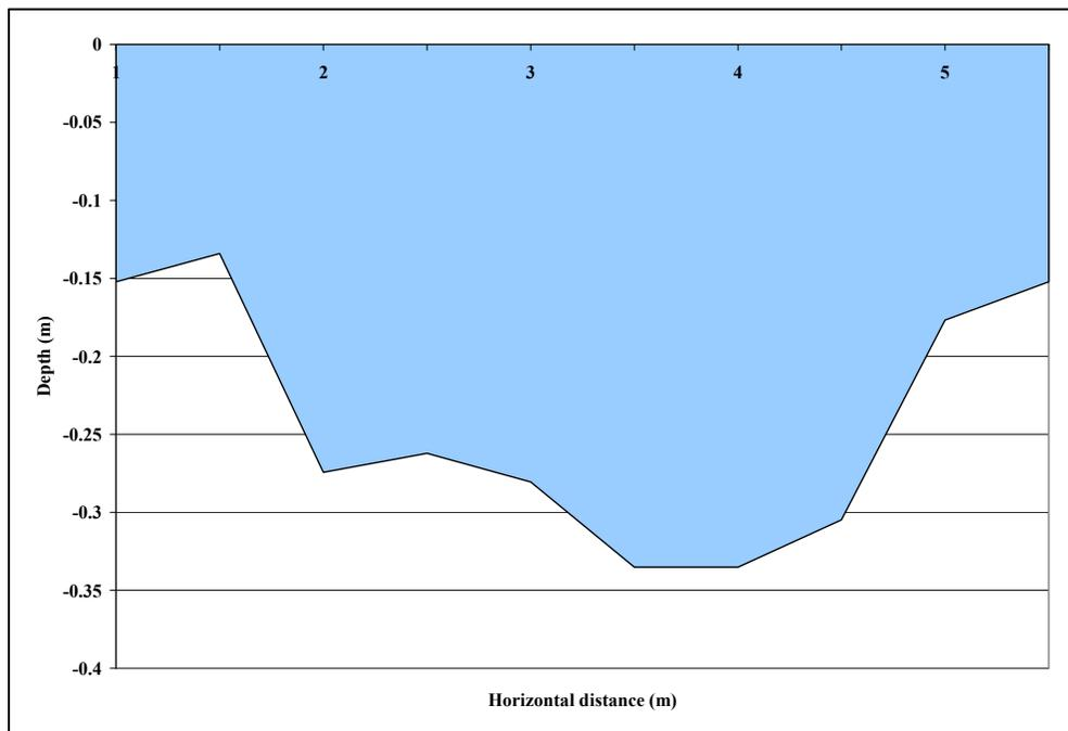
Figure 22. Río Jauca cross section area at grab sampling site.
