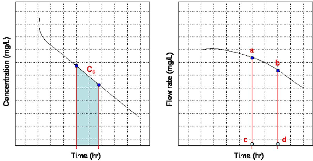
Figure 10. Concentration (TP, DP, TKN or TSS) versus time and flow versus time for predetermined equal flow volumes between time intervals.
