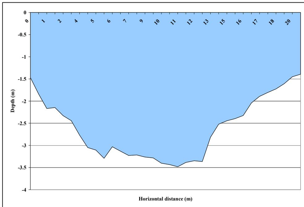
**Figure 18. Río Jauca cross section at storm sampling sites.**
