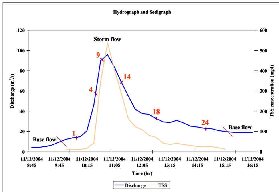
Figure 40. Typical sampling scheme for nutrients during a storm event.
