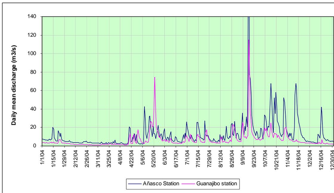
**Figure 5.3.7. Daily mean discharge for the *Rio Grande de Añasco near San Sebastian* and *Rio Guanajibo near Hormigueros* stations (only shown values of daily mean discharge up to 140 m<sup>3</sup>/s for visualization purposes).**
