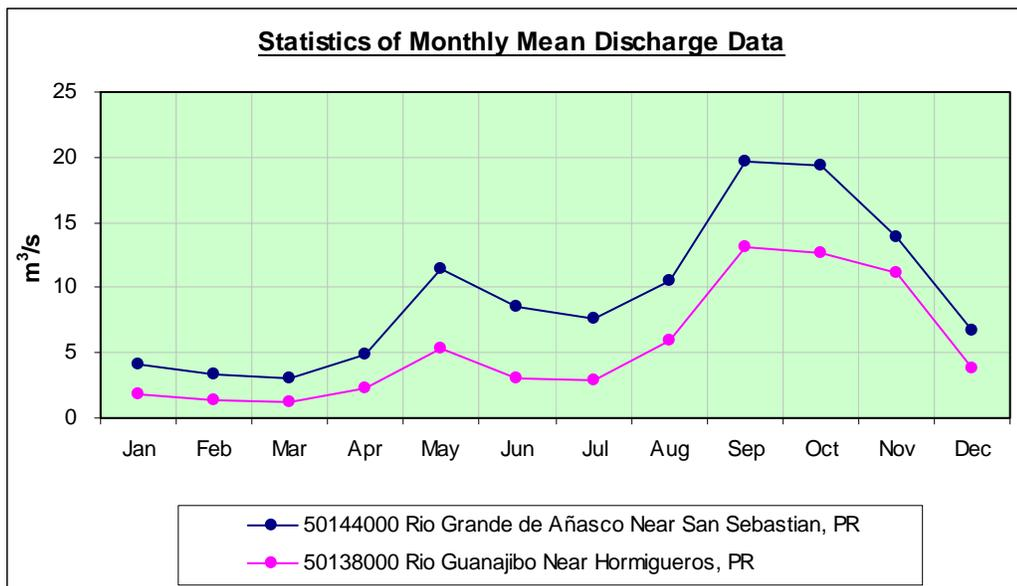
**Figure 4.3.2. Statistics of monthly mean discharge data for the 50144000 Rio Grande de Añasco near San Sebastian, PR and 50138000 Rio Guanajibo near Hormigueros, PR stations.**
