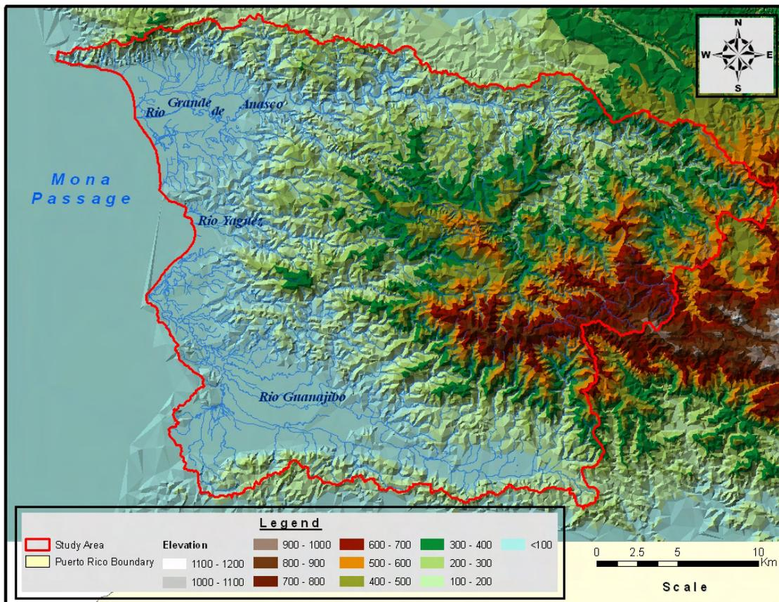
**Figure 4.1.2. Triangulated surface (TIN) of the study area land elevation (units are meters over mean sea level).**
