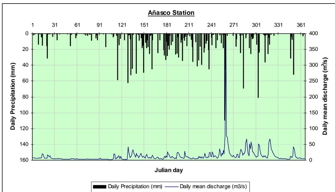
**Figure 5.3.5. Daily mean discharge and precipitation for the *Rio Grande de Añasco near San Sebastian* station (USGS 50144000).**
