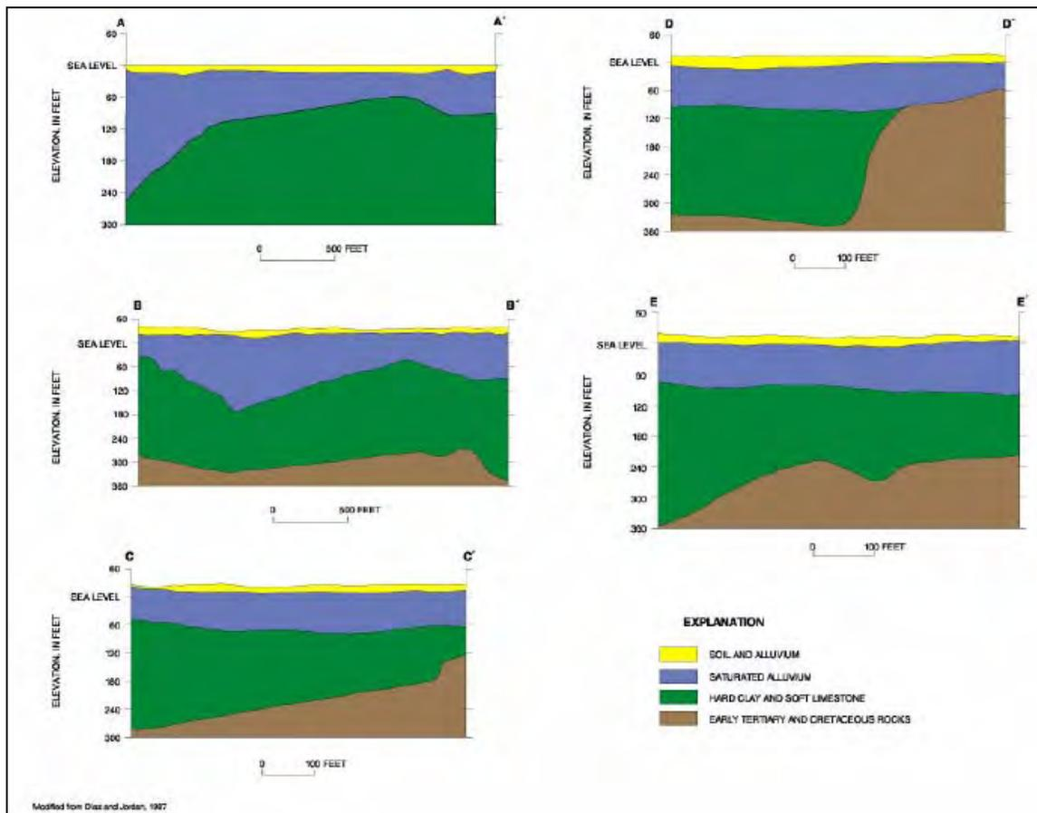
**Figure 4.4.3. Subsurface materials cross sections obtained from seismic profiles and well log information in the Río Grande de Añasco lower valley. (Location of sections shown in Figure 5.4.2) (Source: Veve and Taggart, 1996; presented with authorization from the USGS Caribbean Water Science Center).**
