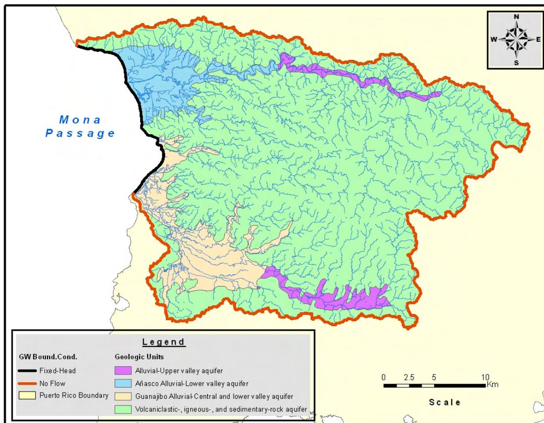
**Figure 5.6.2. Conceptualization of the geologic units spatial distribution and ground-water boundaries.**
