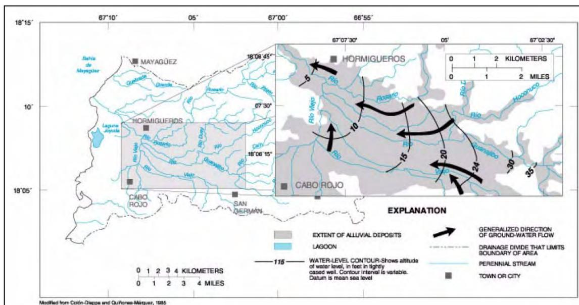
**Figure 4.4.8. Altitude of water-level surface and direction of ground-water flow during June 1980 (Source: Veve and Taggart, 1996; presented with authorization from the USGS Caribbean Water Science Center).**
