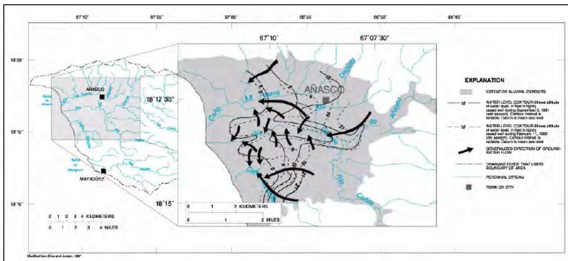
**Figure 4.4.4. Altitude of water table in the alluvial aquifer (Zone II) for September 1981 and February 1982, and direction of ground-water flow during September 1981 for the Río Grande de Añasco lower valley (Source: Veve and Taggart, 1996; presented with authorization from the USGS Caribbean Water Science Center).**
