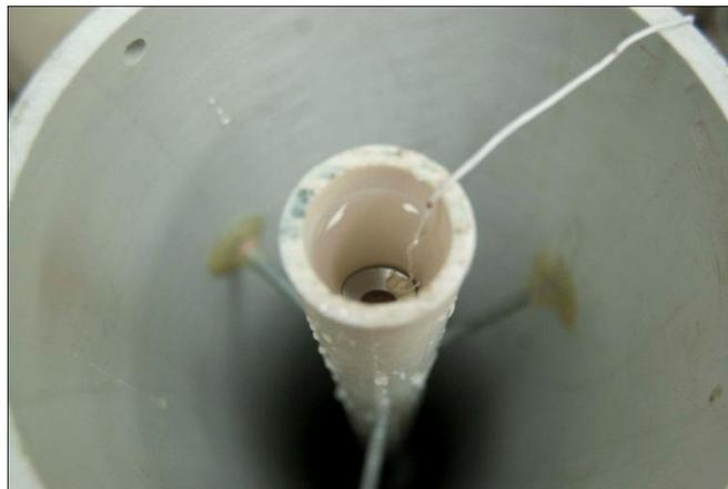
Figure 4-1 Water-filled PVC tube used for the experiment and measurements. An 80% stainless steel obstruction is located at 75cm from the bottom part of the PVC tube where the hydrophone is located.
