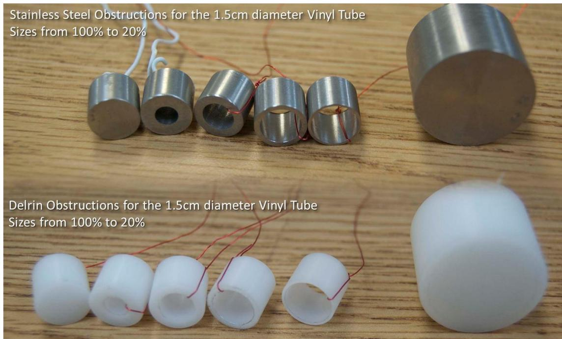
Figure 3-20 Stainless Steel and Delrin obstructions used for the 1.5 diameter vinyl tube.
