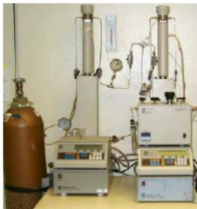
**Figure 4.5: Supercritical Fluid extraction unit**
