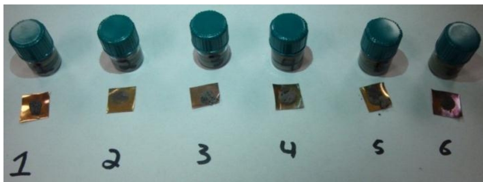
Figure 36: Some results from the preliminary solder paste test (ethylene glycol, citric acid, and hydrogenated rosin).
