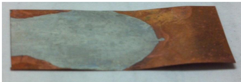
Figure 39: As reflow sample of synthesized Sn-nanoparticle paste on top of a Cu substrate.
