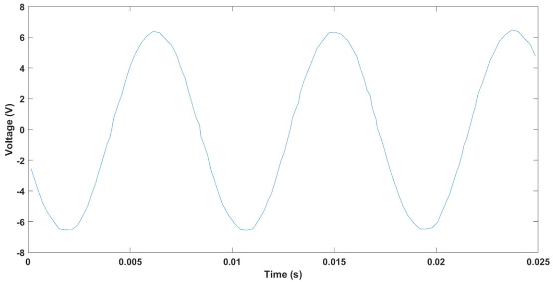
Figure 15: No Load Output Voltage using LTG Second Configuration at 114Hz
