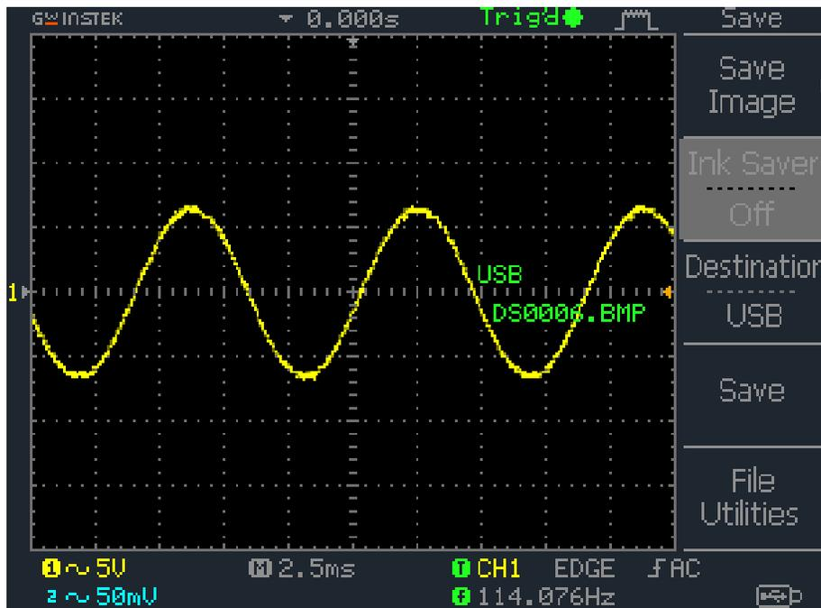
Figure 39: No Load Output Voltage using LTG Second Configuration at 114Hz
