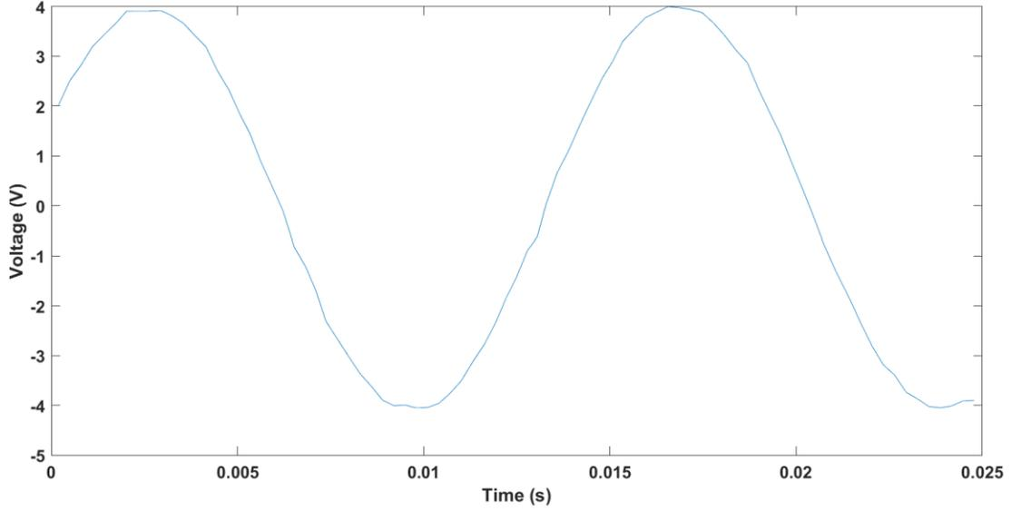
Figure 11: No Load Output Voltage using LTG Second Configuration at 70Hz
