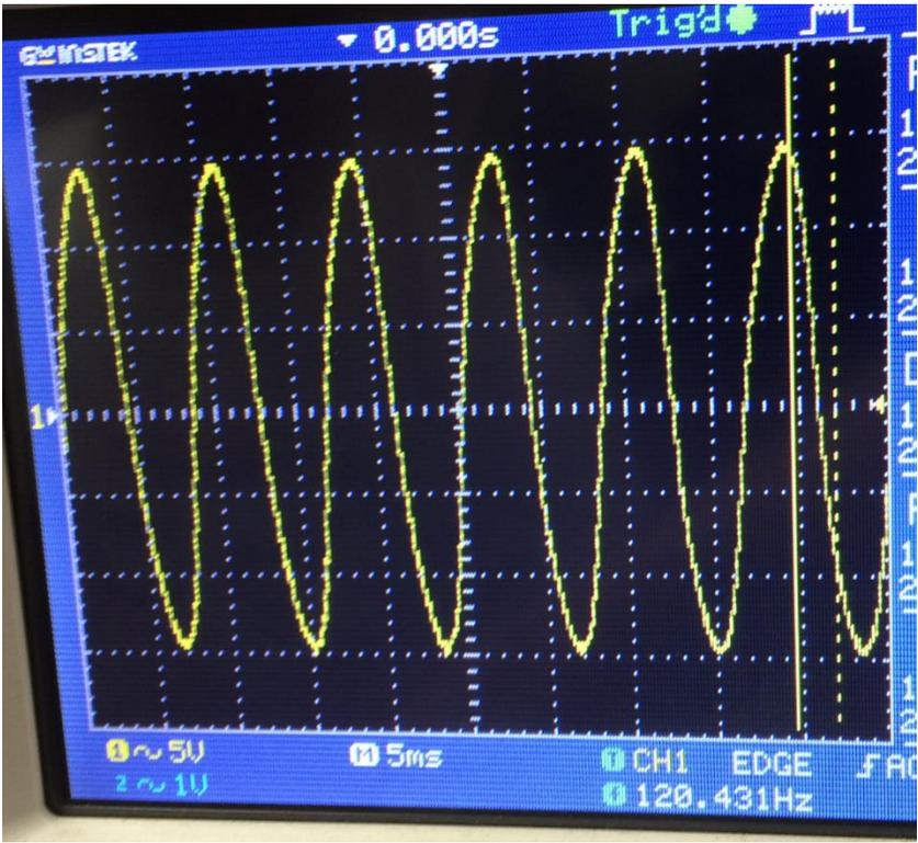
Figure 45: No Load Output Voltage using LTG Third Configuration at 120Hz with Less Waveform
