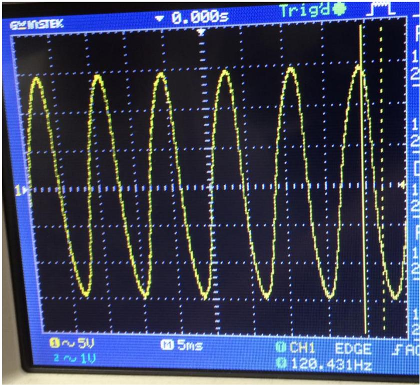
Figure 45: No Load Output Voltage using LTG Third Configuration at 120Hz with Less Waveform Distortion
