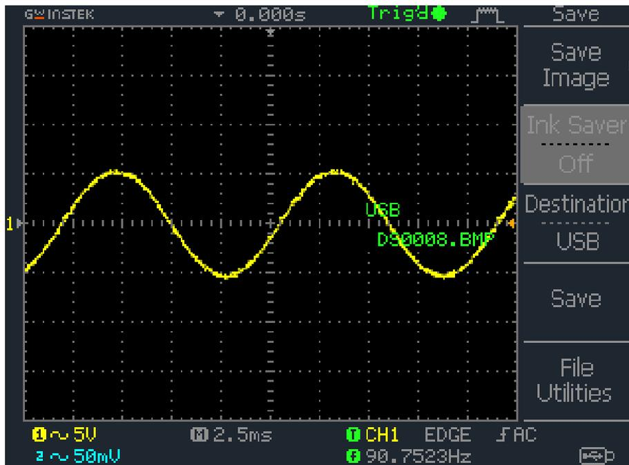
Figure 37: No Load Output Voltage using LTG Second Configuration at 90Hz
