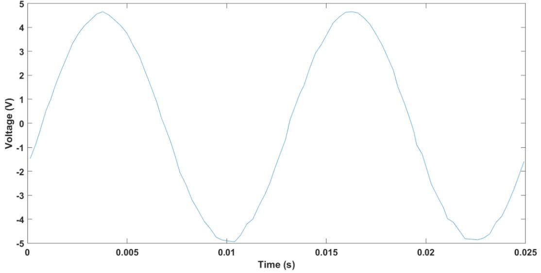
Figure 12: No Load Output Voltage using LTG Second Configuration at 80Hz
