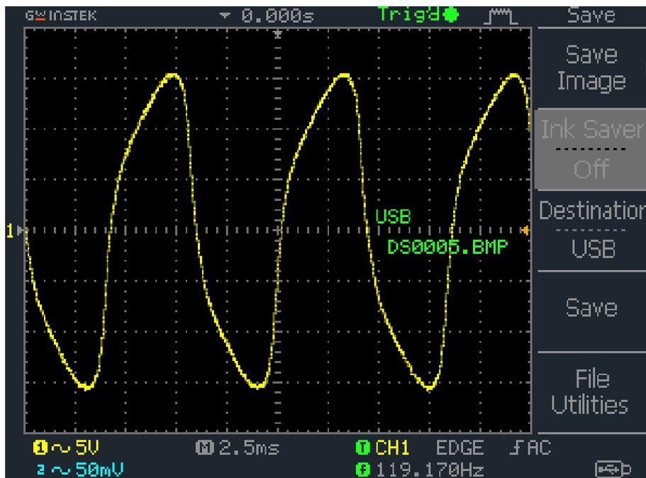
Figure 44: No Load Output Voltage using LTG Third Configuration at approximately 120Hz
