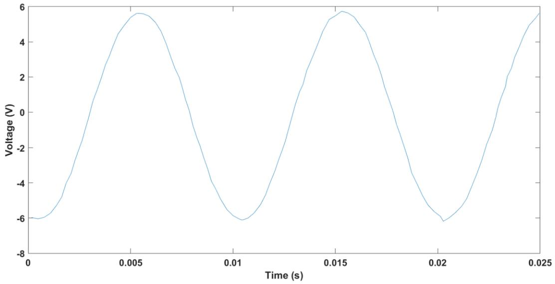
Figure 14: No Load Output Voltage using LTG Second Configuration at 100Hz
