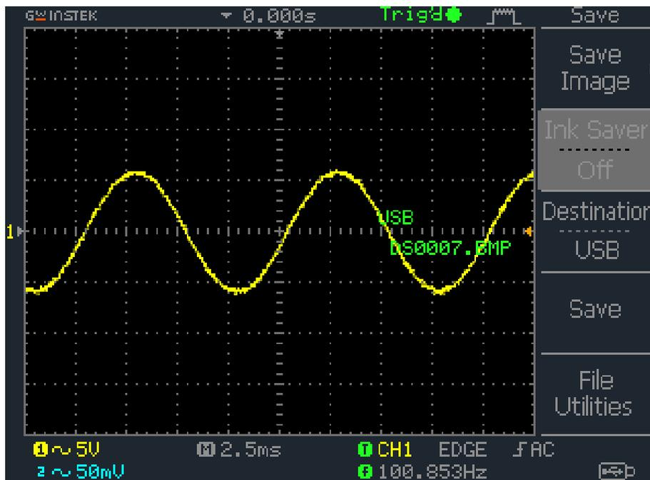
Figure 38: No Load Output Voltage using LTG Second Configuration at 100Hz
