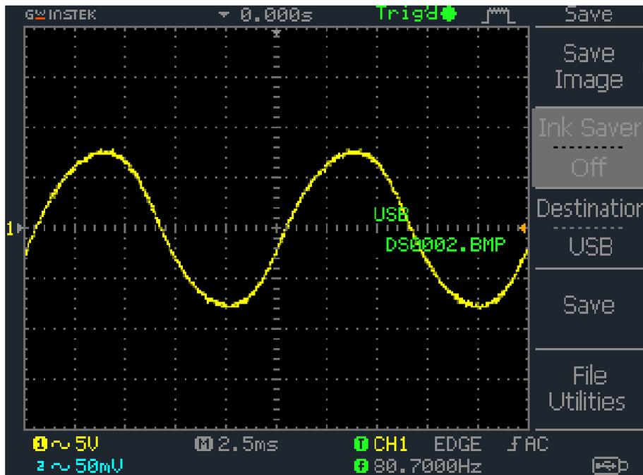
Figure 41: No Load Output Voltage using LTG Third Configuration at 80Hz
