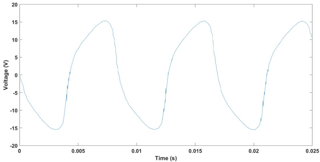
Figure 22: No Load Output Voltage using LTG Third Configuration at 119Hz
