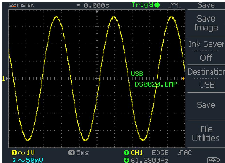
Figure 30: No Load Output Voltage using LTG Second Configuration
