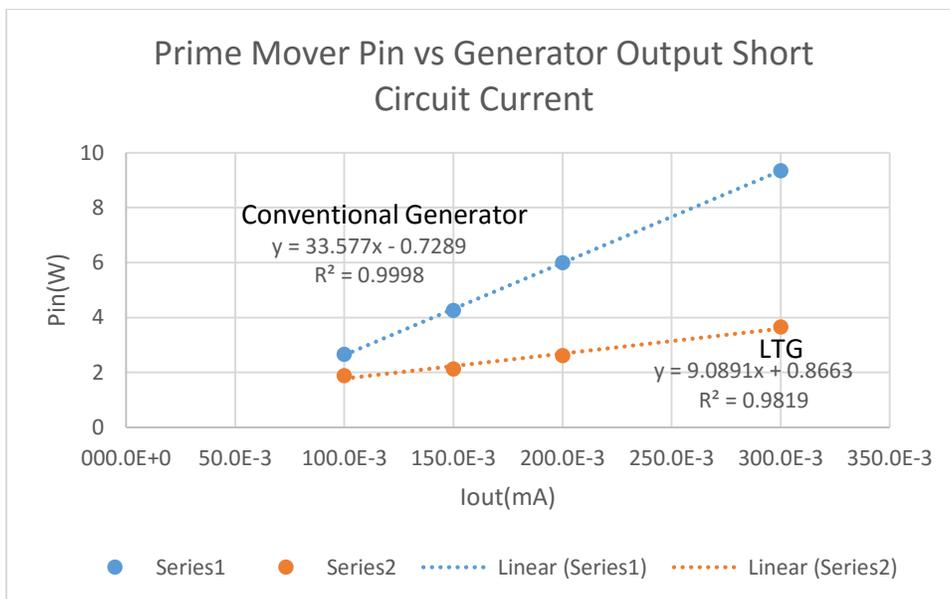
Figure 25: LTG Second Configuration Prime Mover Input Current versus Short Circuit Output Current
