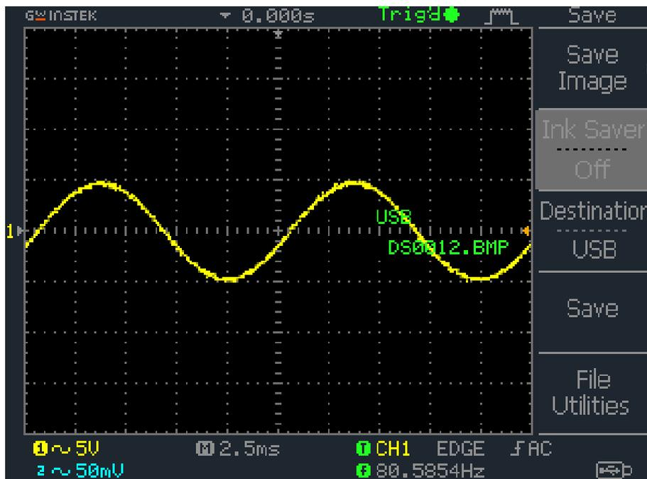
Figure 36: No Load Output Voltage using LTG Second Configuration at 80Hz
