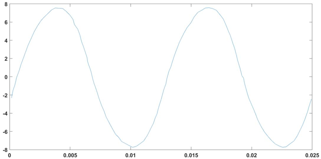
Figure 19: No Load Output Voltage using LTG Third Configuration at 80Hz
