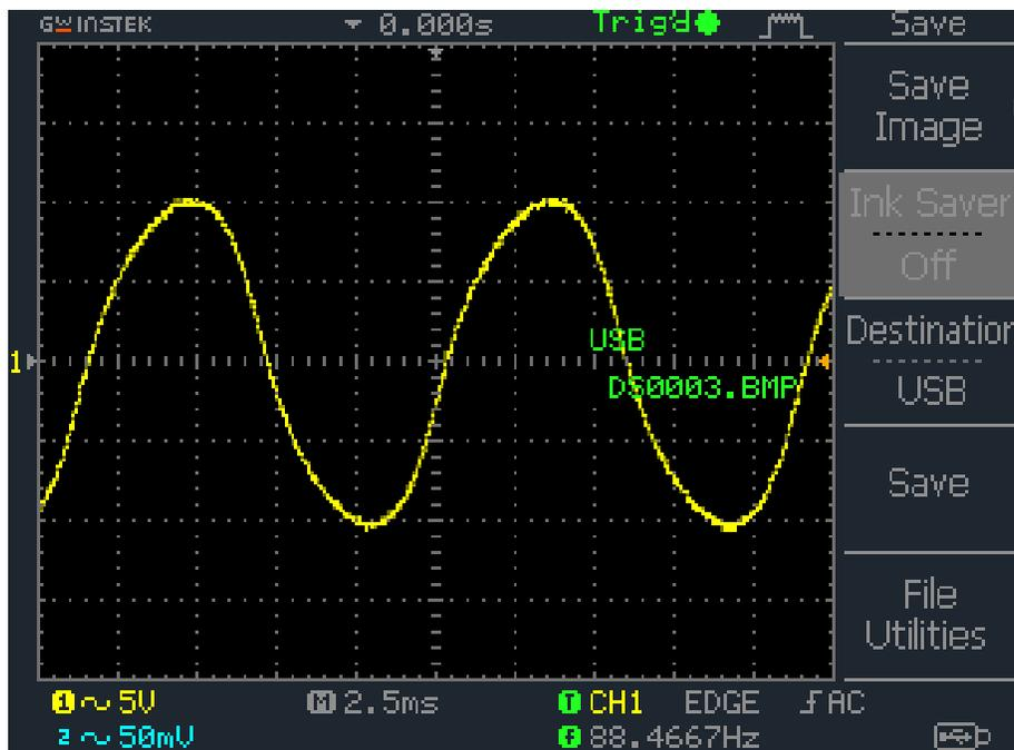
Figure 42: No Load Output Voltage using LTG Third Configuration at approximately 90Hz
