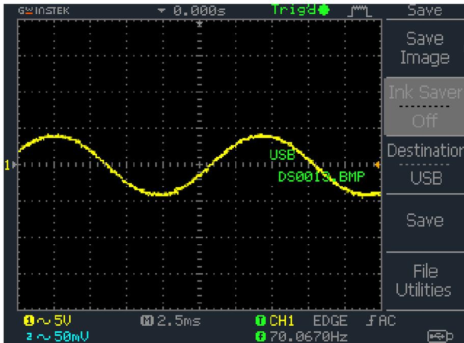
Figure 35: No Load Output Voltage using LTG Second Configuration at 70Hz
