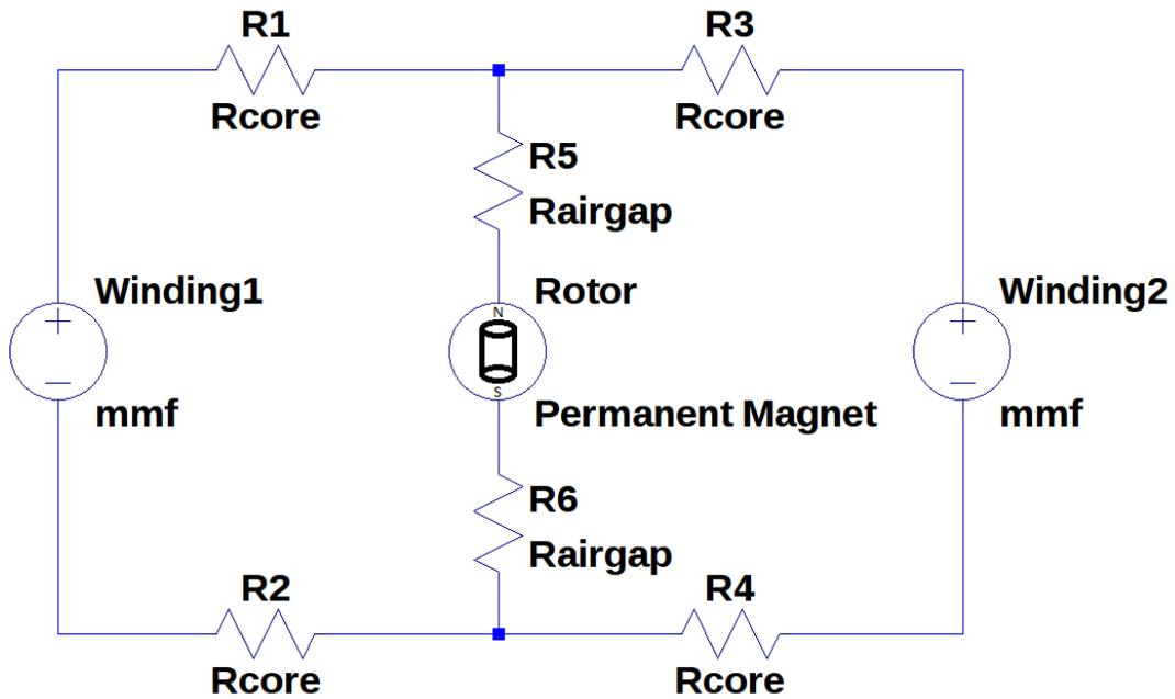
Figure 27: Magnetic Circuit of the Low Torque Generator for Two Windings on the Stator
