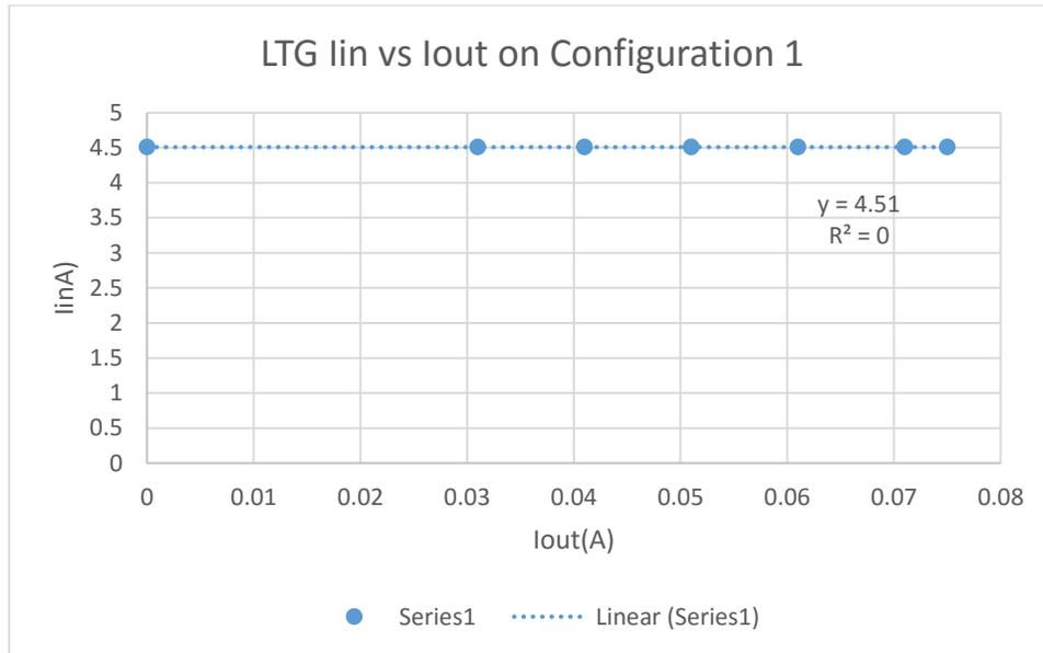
Figure 23: LTG First Configuration Prime Mover Input Current versus Output Current
