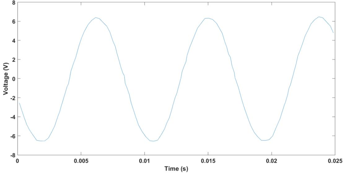
Figure 15: No Load Output Voltage using LTG Second Configuration at 114Hz
