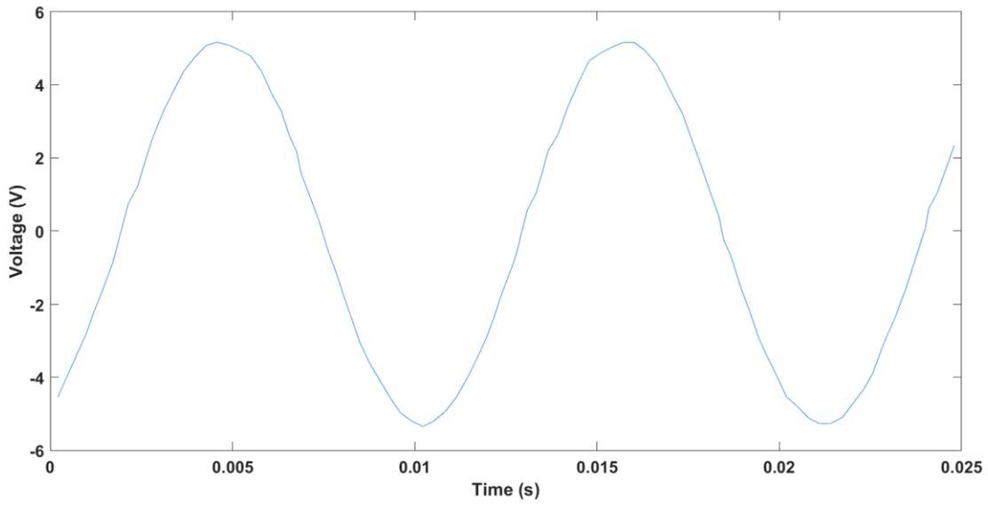
Figure 13: No Load Output Voltage using LTG Second Configuration at 90Hz
