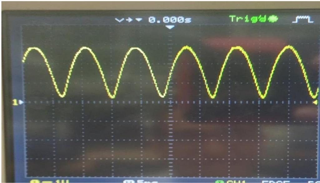
Figure 31: Bridge Rectification of the LTG Second Configuration
