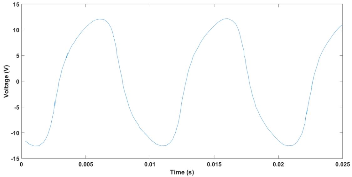
Figure 21: No Load Output Voltage using LTG Third Configuration at approximately 100Hz
