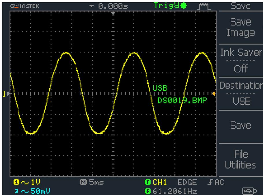
Figure 29: No Load Output Voltage using LTG First Configuration
