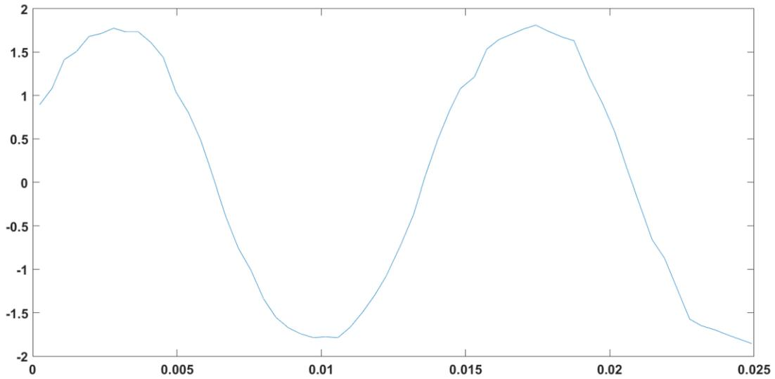
Figure 18: No Load Output Voltage using LTG Third Configuration at approximately 70Hz
