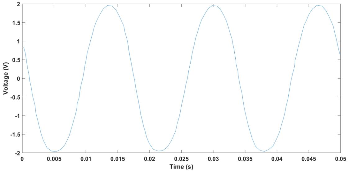
Figure 7: No Load Output Voltage using LTG First Configuration
