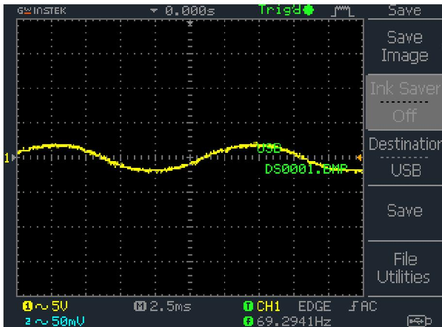
Figure 40: No Load Output Voltage using LTG Third Configuration at approximately 70Hz
