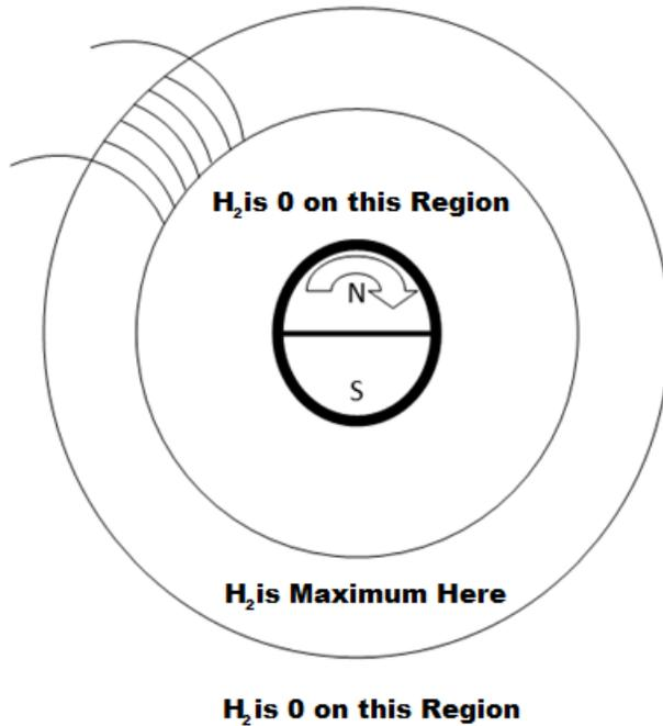
Figure 2: Magnetic Field Intensity  $H_2$  per Region of the LTG
