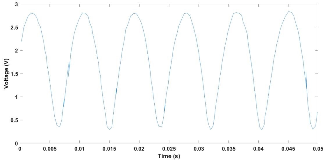
Figure 16: Output Voltage of Bridge Rectifier for LTG Second Configuration
