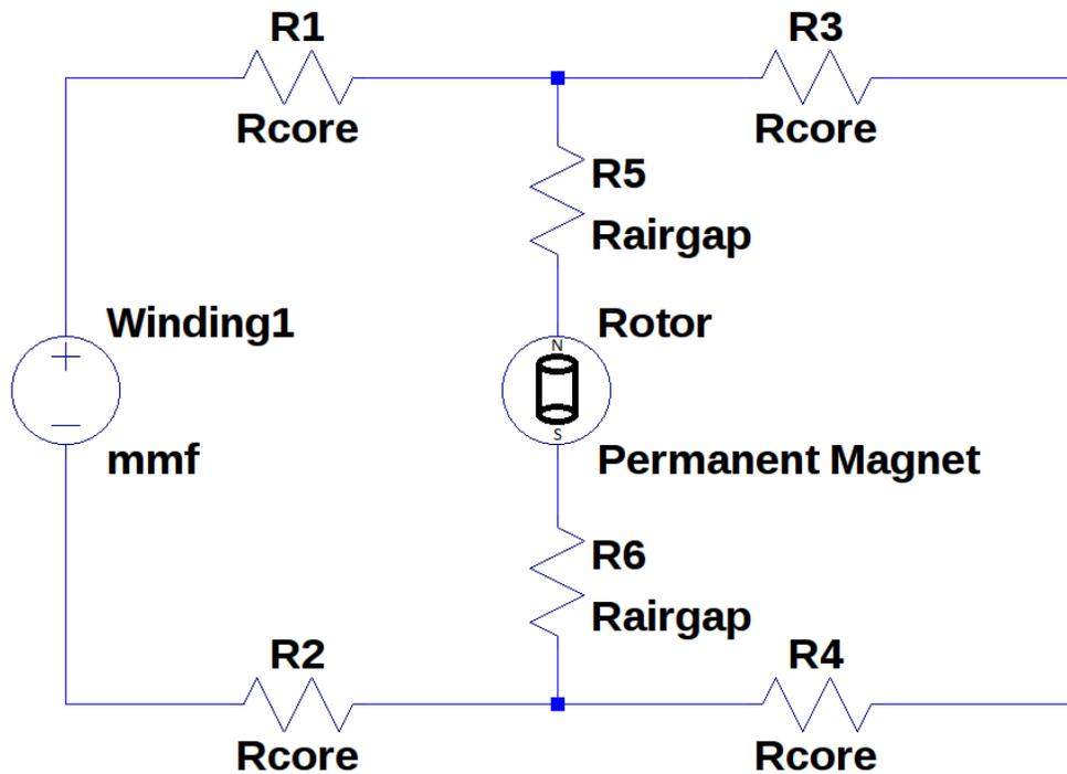
Figure 26: Magnetic Circuit of the Low Torque Generator for One Winding on the Stator
