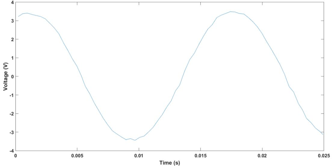
Figure 10: No Load Output Voltage using LTG Second Configuration at 60Hz
