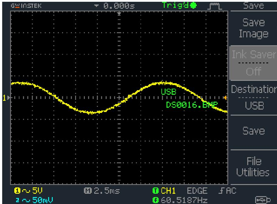
Figure 34: No Load Output Voltage using LTG Second Configuration at 60Hz
