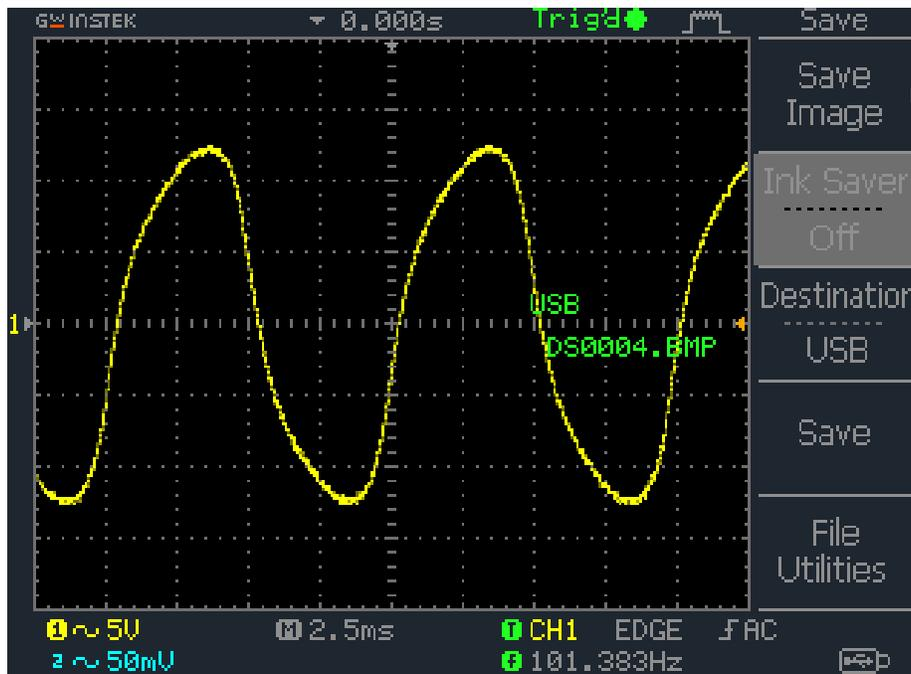
Figure 43: No Load Output Voltage using LTG Third Configuration at approximately 100Hz
