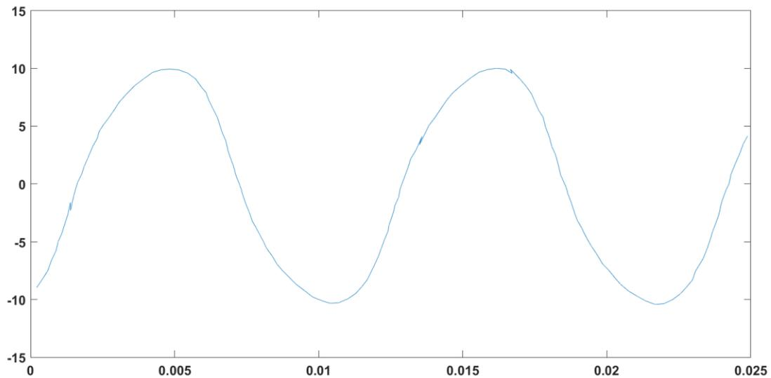
Figure 20: No Load Output Voltage using LTG Third Configuration at approximately 90Hz
