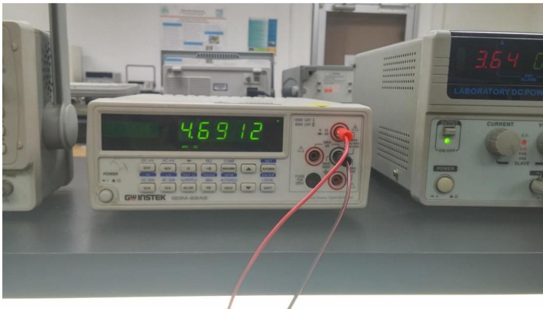
Figure 32: Lamp Voltage of the LTG Second Configuration using the Bridge Rectifier Circuit
