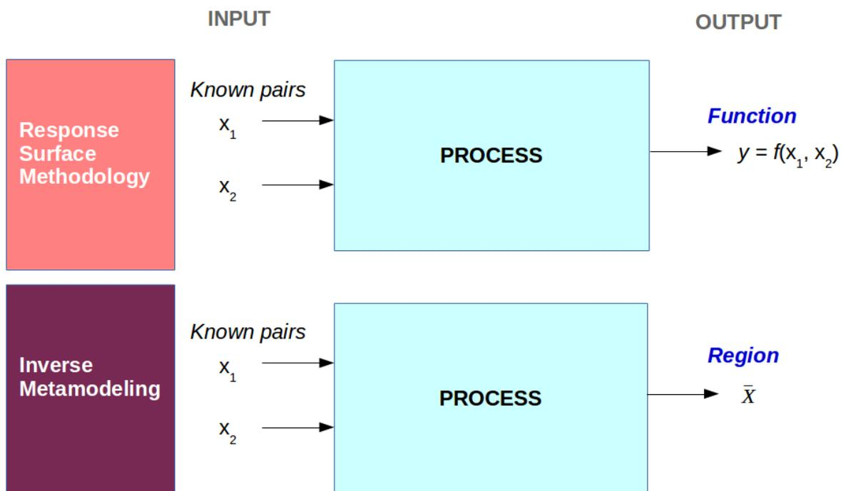
Figure E1. System diagrams comparing the Response Surface Methodology and the Inverse Metamodeling technique.
