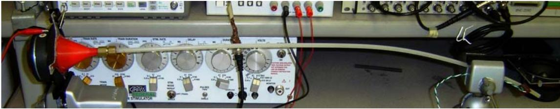
Fig. 4.3 Pulse-echo acoustic reflectometry system
