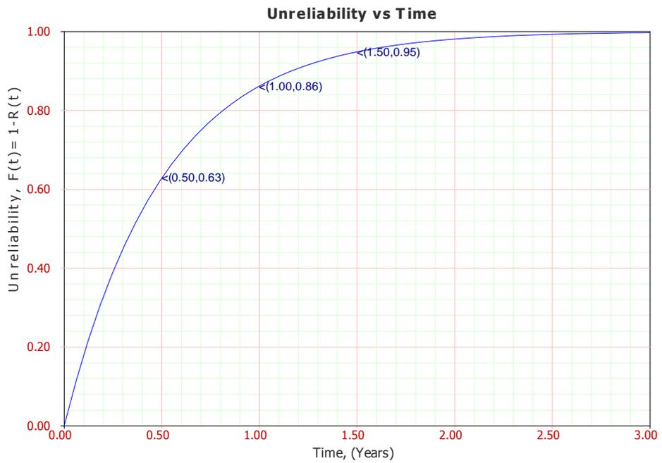
**Figure 3-10 Unreliability vs. Time plot for 2500 KVA SUB (including utility)**
