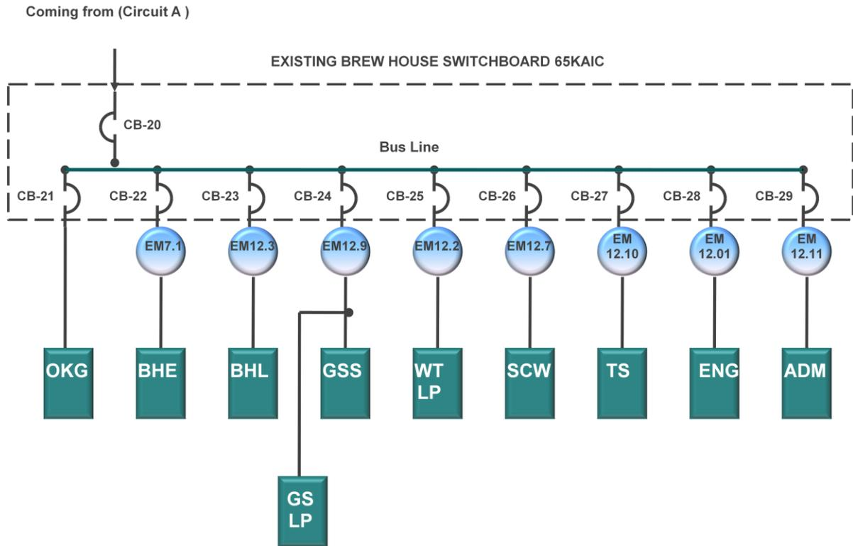
Figure A-3: 4200 KVA Substation One Line Diagram for Section II Circuit B (Brew House). Refer to Appendix B for more details on components ratings and descriptions.
