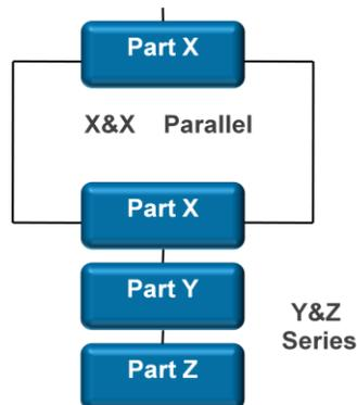
**Figure 2-6 System consisting of parallel and series redundancies.**
