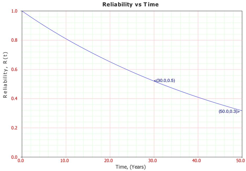
**Figure 3-7 Reliability vs. Time plot for 2500 KVA SUB (without utility)**
