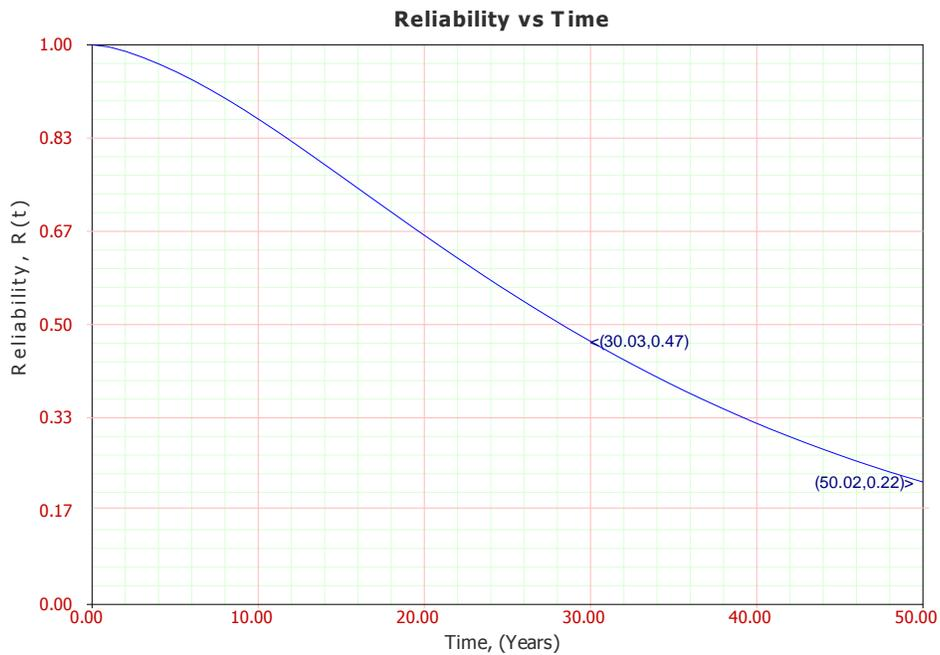
**Figure 3-11 Reliability vs. Time Function plot for 4200 KVA SUB (without utility)**
