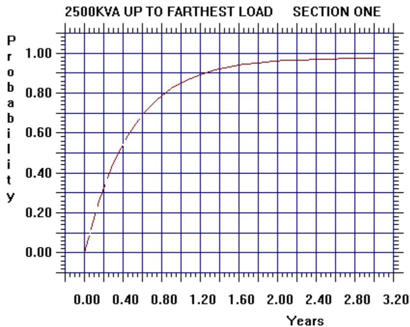
**Figure 3-29 2500 KVA Substation Section 1 (with utility and up to farthest load)**
