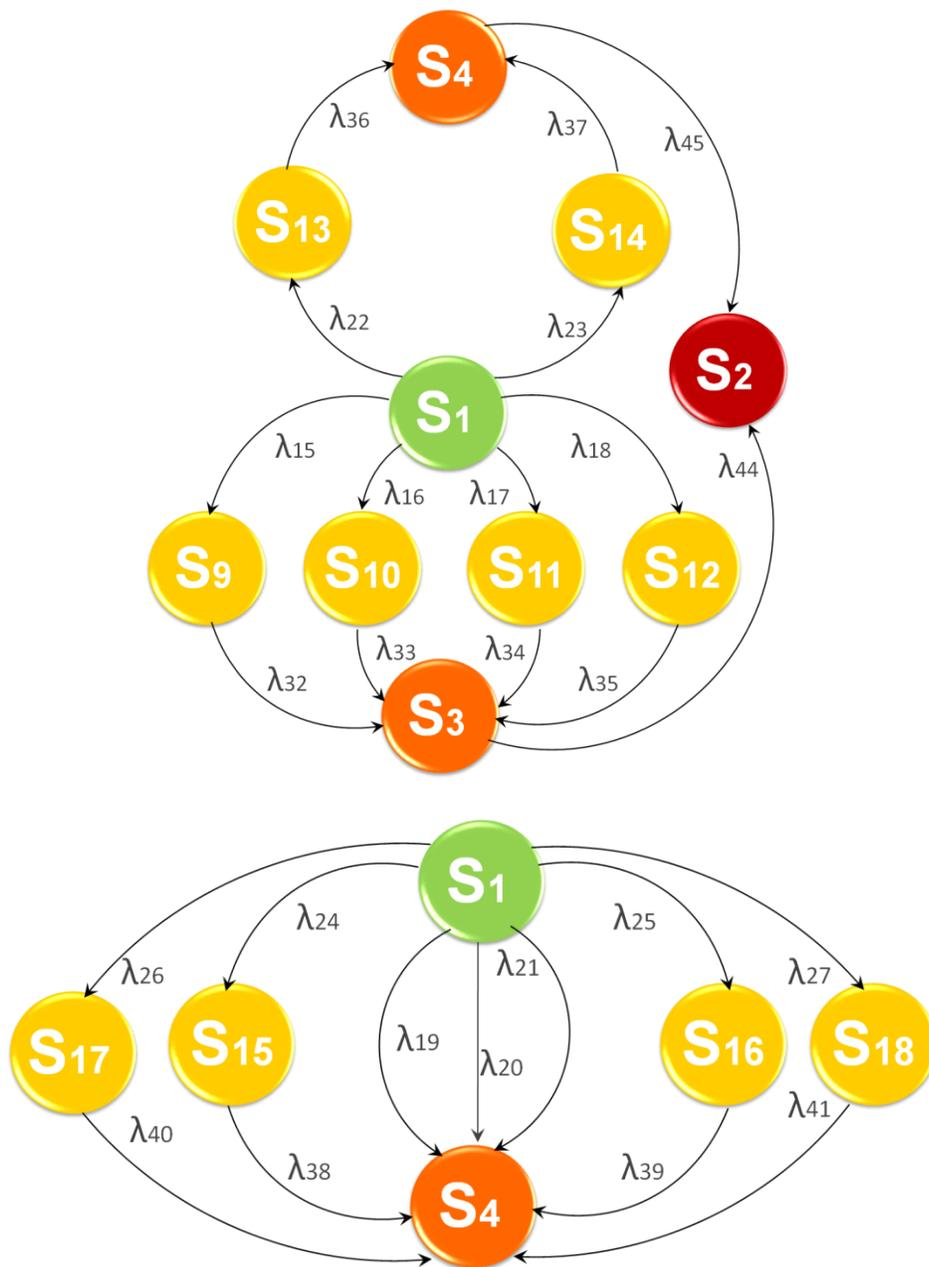
**Figure 3-25 4200 KVA State Diagram up to the Bus Bar.**
