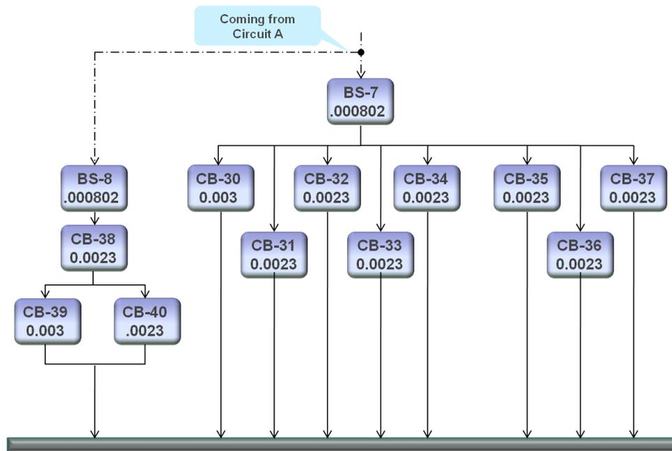
**Figure 3-21 RBD for 4200 KVA Substation for Circuit C**
