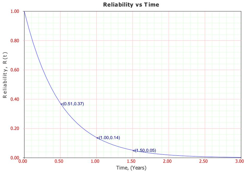
**Figure 3-9 Reliability vs. Time plot for 2500 KVA SUB (including utility)**
