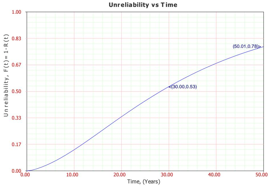
**Figure 3-12 Unreliability vs. Time Function plot for 4200 KVA SUB (without utility)**
