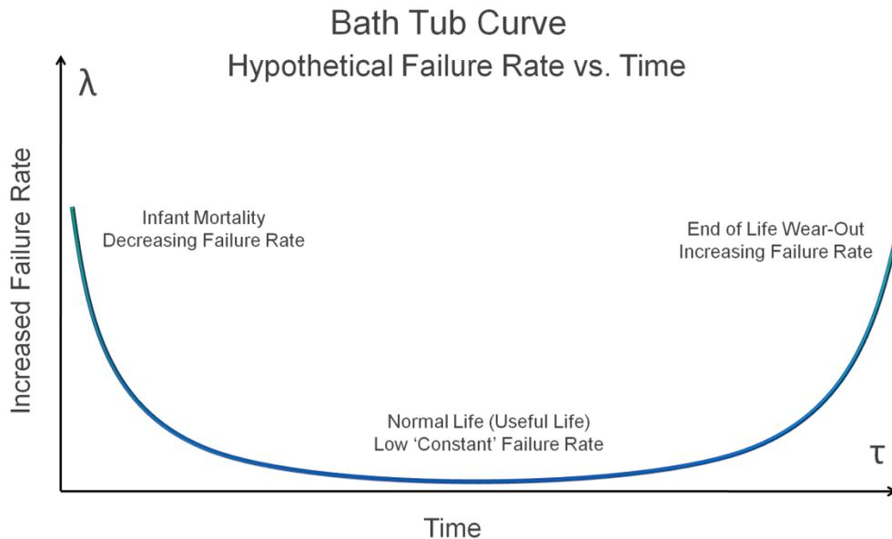
**Figure 3-6 Bath Tub Curve**
