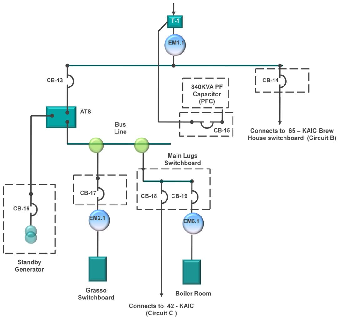
**Figure 3-18 4200 KVA One Line Diagram for Section II Circuit A. Taken from Appendix A**
