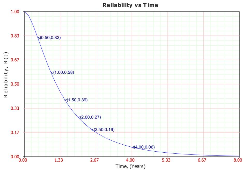
**Figure 3-13 Reliability vs. Time Function plot for 4200 KVA SUB (including utility)**
