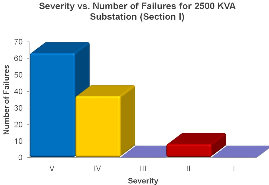
**Figure 3-3 FMEA Severity vs. Number of Failures for 2500 KVA Substation.**
