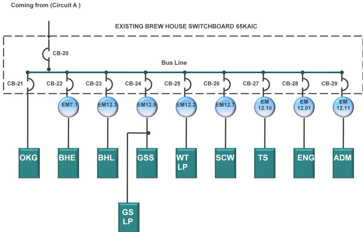
**Figure 3-20 4200KVA One Line Diagram for Section II Circuit B. Taken from Appendix A**
