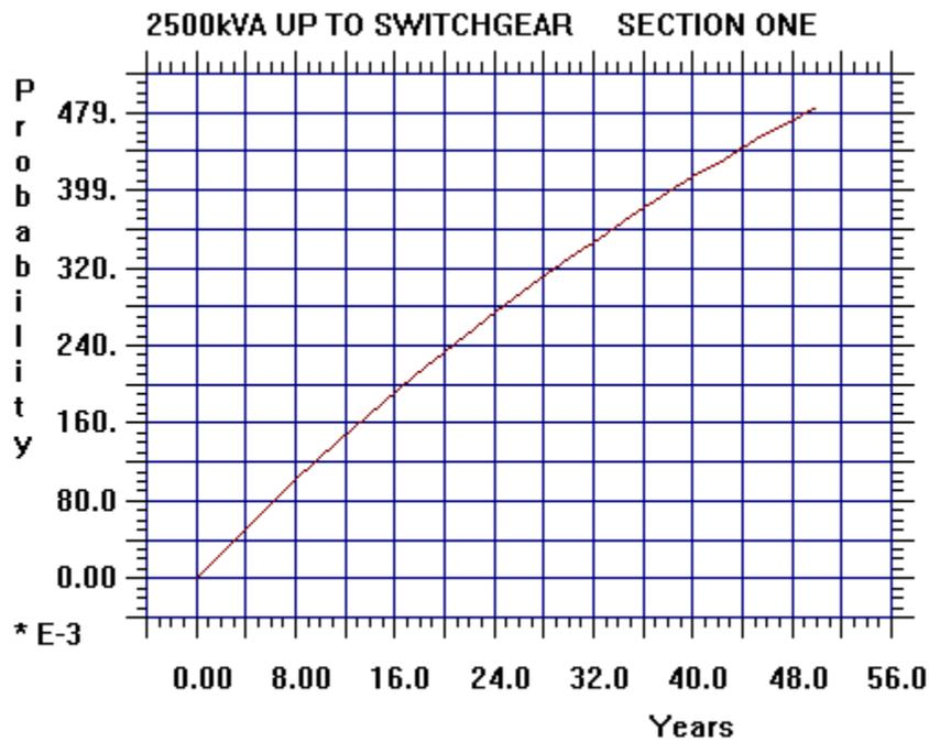
**Figure 3-28 2500 KVA Substation Section 1 without utility and up to switchgear**
