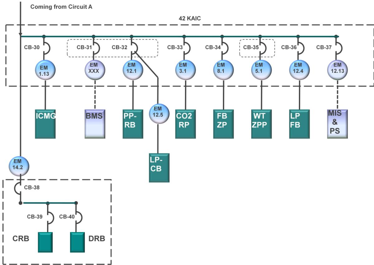
**Figure 3-22 4200 KVA One Line Diagram for Section II Circuit C. Taken from Appendix A**
