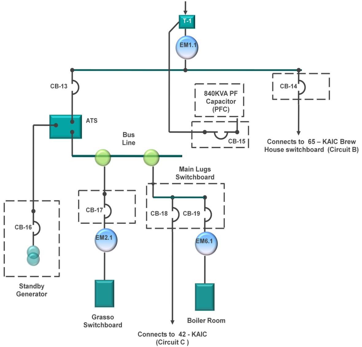
Figure A-2: 4200 KVA Substation One Line Diagram for Section II Circuit A. Refer to Appendix B for more details on components ratings and descriptions.
