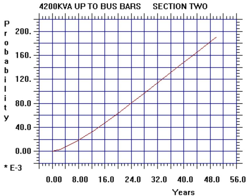
Figure 3-32 4200 KVA Substation Section 2 (without utility and up to bus bar)
