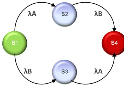
**Figure 2-8 State diagram for a parallel configuration.**
