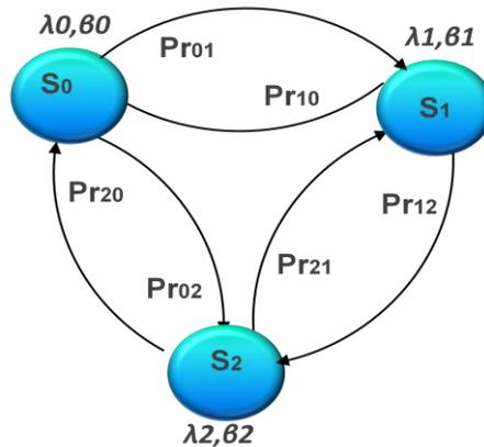
**Figure 1-2 Three State Weibull Markov model with parameters. Taken from [4]**
