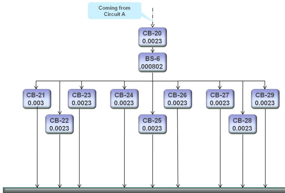
**Figure 3-19 RBD for 4200 KVA Substation for Circuit B**
