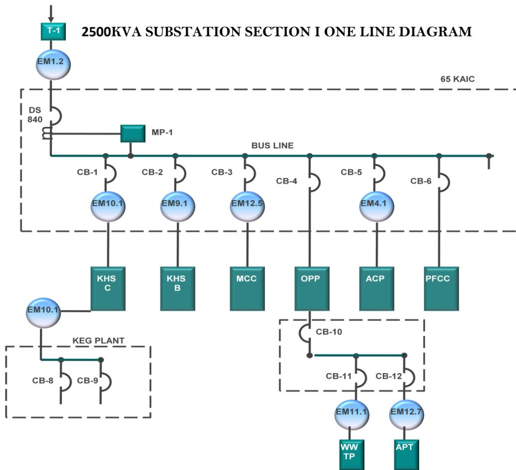
**Figure 3-16 2500 KVA One Line Diagram. Taken from Appendix A**
