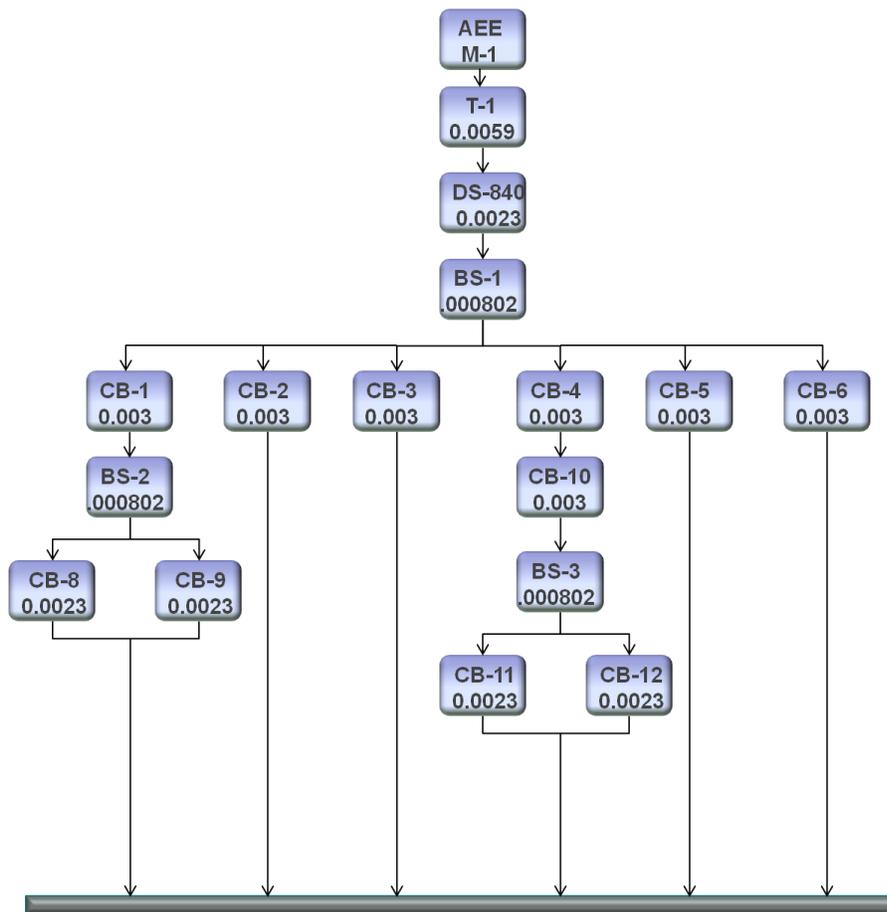
**Figure 3-15 RBD for 2500 KVA Substation**
