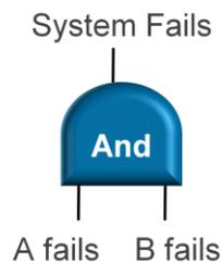
**Figure 2-7 FTA diagram for a parallel configuration.**
