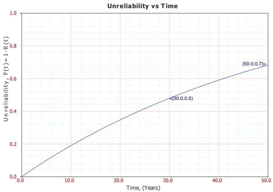
**Figure 3-8 Unreliability vs. Time plot for 2500 KVA SUB (without utility)**
