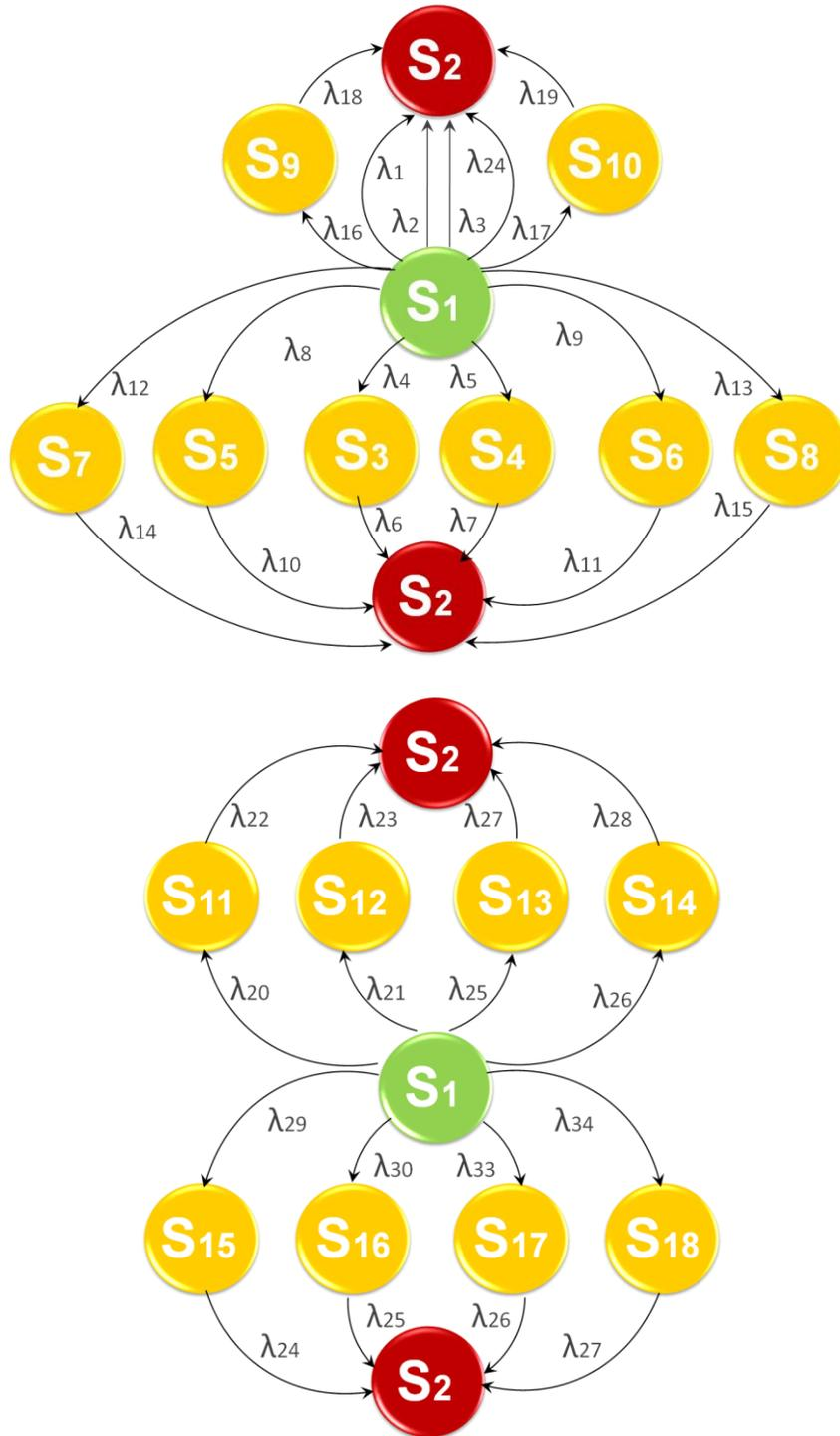
Figure 3-26 4200 KVA State Diagram up to farthest load (worst case scenario)
