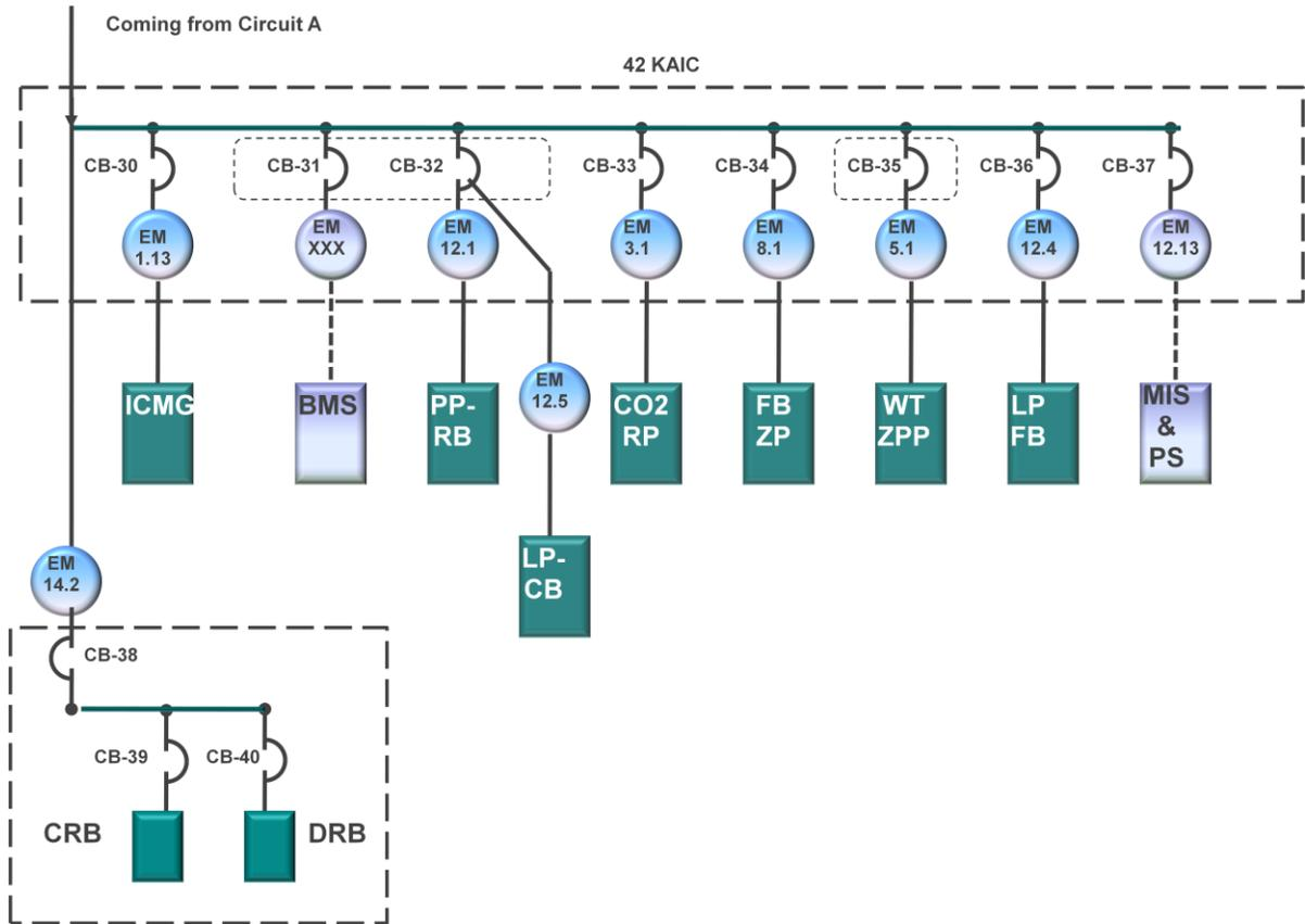
Figure A-4: 4200 KVA Substation One Line Diagram for Section II Circuit C. Refer to Appendix B for more details on components ratings and descriptions.
