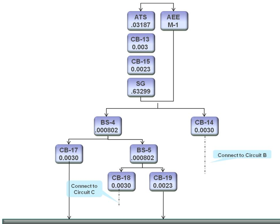
**Figure 3-17 RBD for 4200 KVA Substation for Circuit A**
