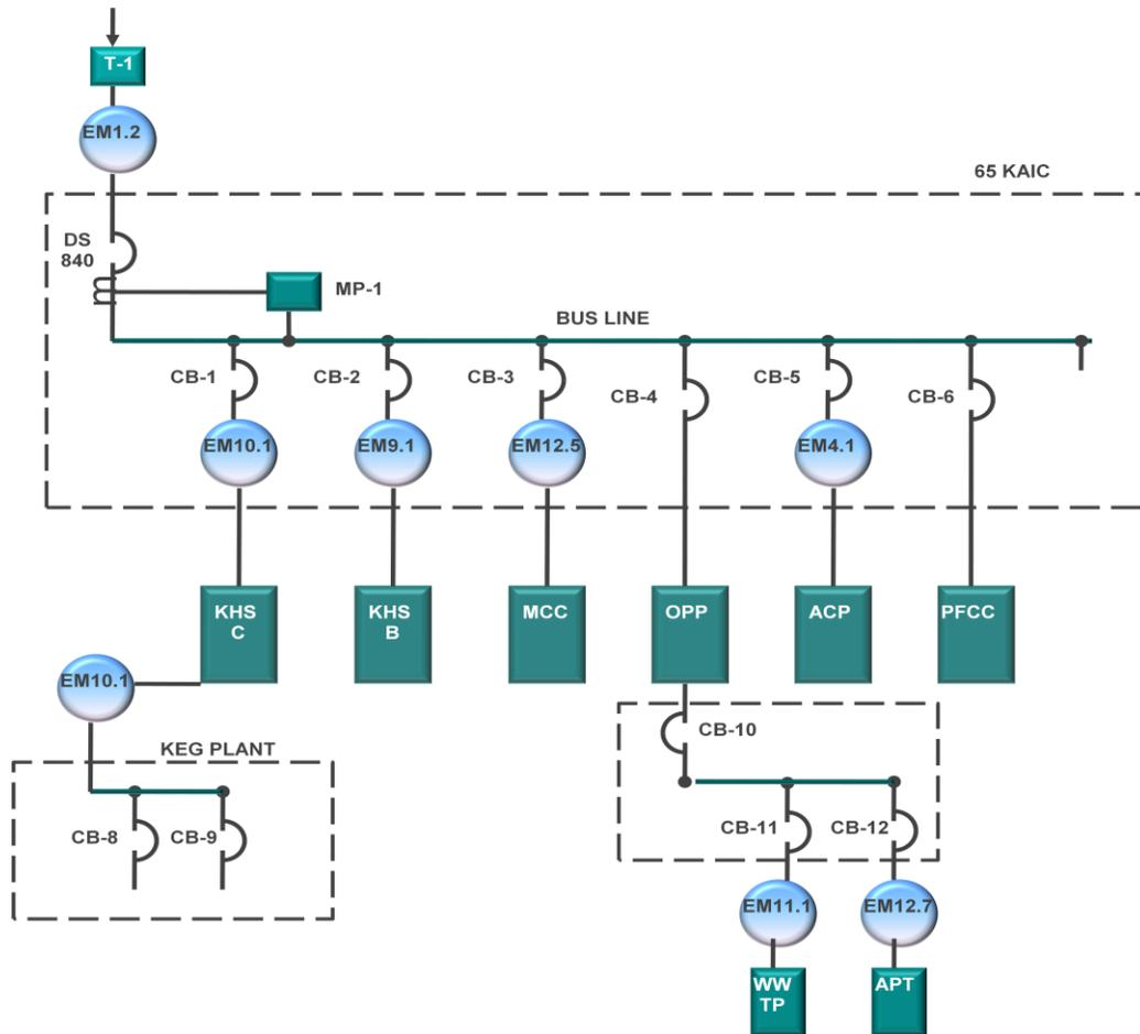
Figure A-1: 2500 KVA Substation One Line Diagram. Refer to Appendix B for more details on components ratings and descriptions.
