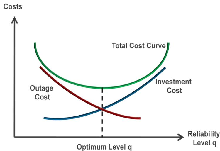
**Figure 1-1 Graph of the optimum reliability level minimizing the total cost. Taken from [3]**
