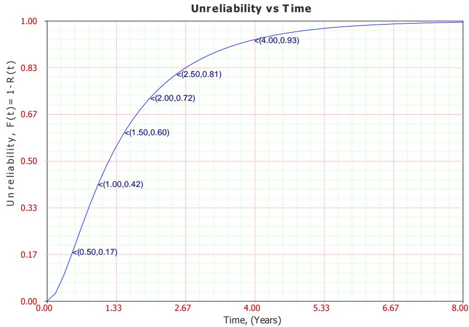
**Figure 3-14 Unreliability vs. Time Function plot for 4200 KVA SUB (including utility)**
