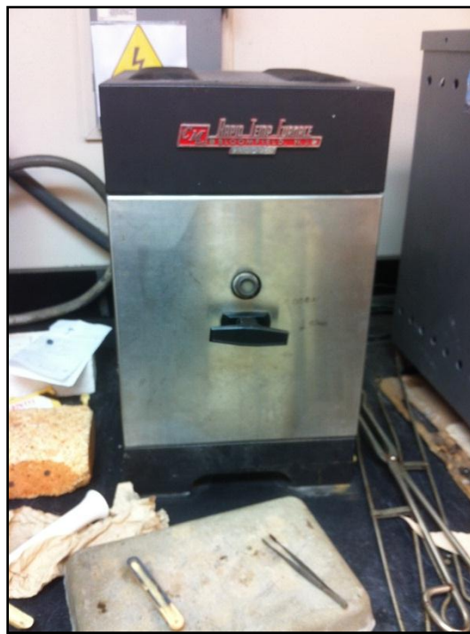
Figure 3.9: High temperature oven used in experimentation.
