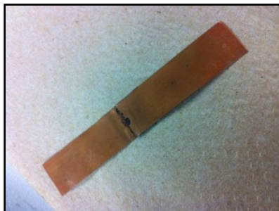
Figure 3.11: Copper Strips joined together by nano-copper solder.
