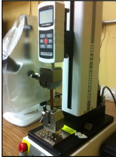
Figure 3.10: Tensile Strength Tester
