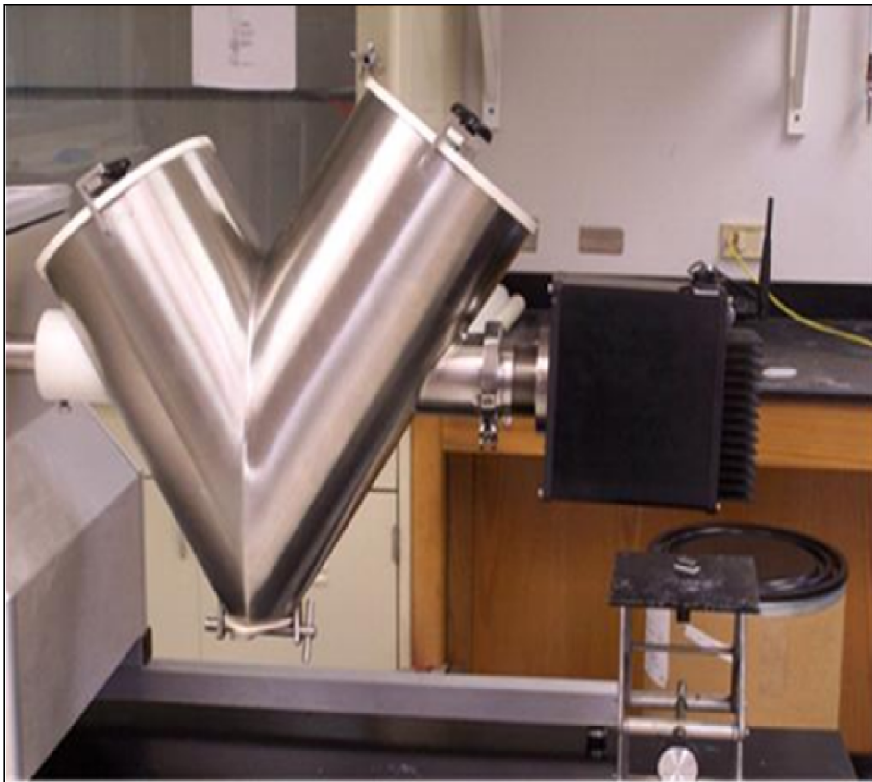
Figure 3.1. V-blender used to mix the placebos with NIR infrared spectrometer attached.
