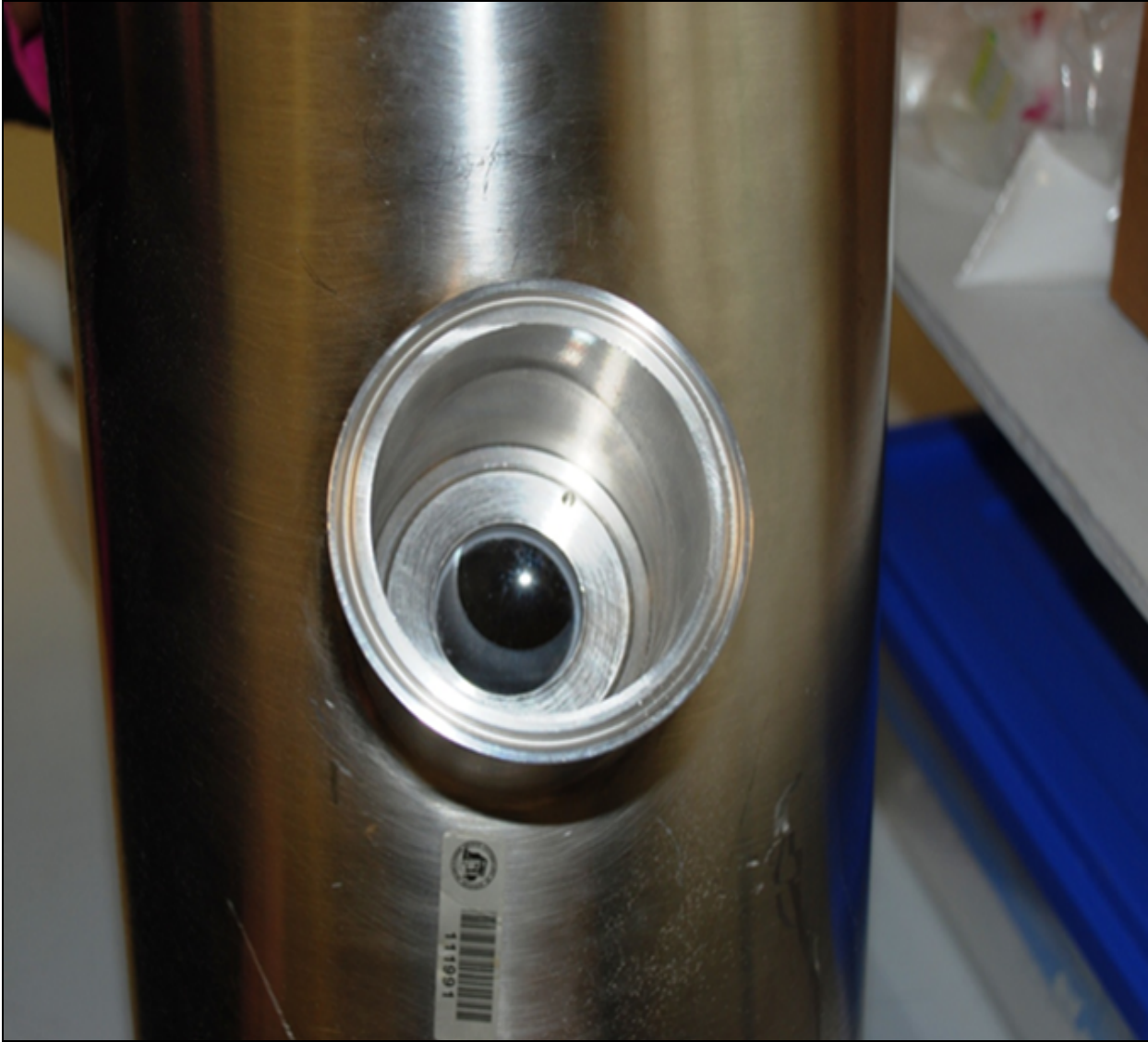
Figure 5.2 Sapphire window in interface coupling the V-blender and NIR spectrometer.
