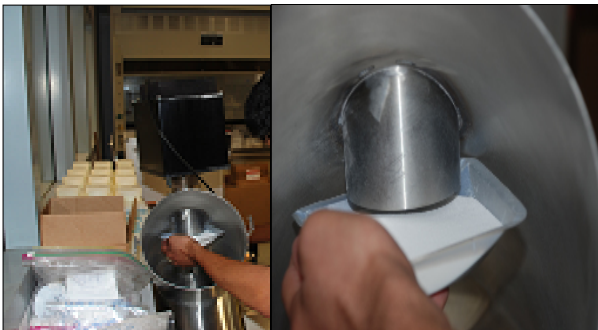
Figure 5.1 Method used to obtain spectra inside v-blender in static mode.
