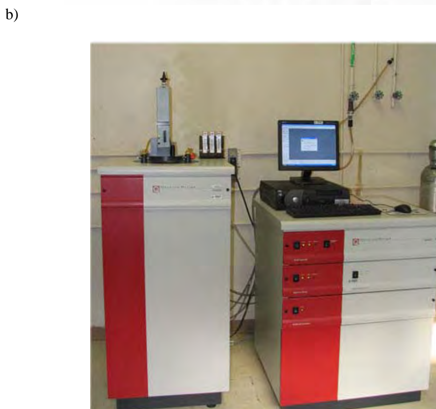
Figure 2.16: (a) Schematic representation of the SQUID unit; (b) Photograph of Quantum Design MPMSXL available at UPRM.
