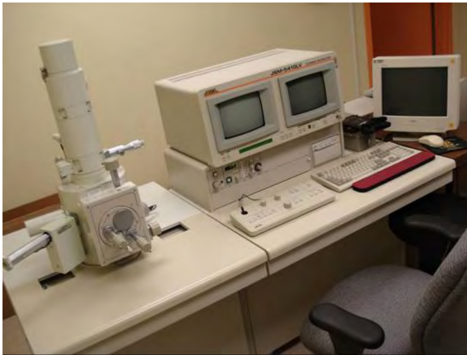
Figure 2.15: (a) Schematic representation of the SEM [34]; (b) Scanning Electron Microscopy (JEOL model JSM-5410 LV available in the Biology microscopy laboratory at UPRM).
