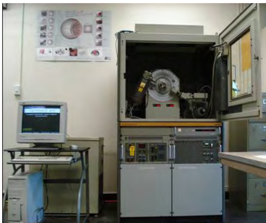
Figure 2.14: (a) Schematic representation of the X-ray diffractometer; (b) Photograph of XRD SIEMENS D500, available on the materials research laboratory at UPRM.
