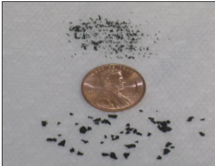
Figure 13. Crumb rubber at different mesh sizes (Mesh 30 above the cent and mesh 14-20 below the coin)
