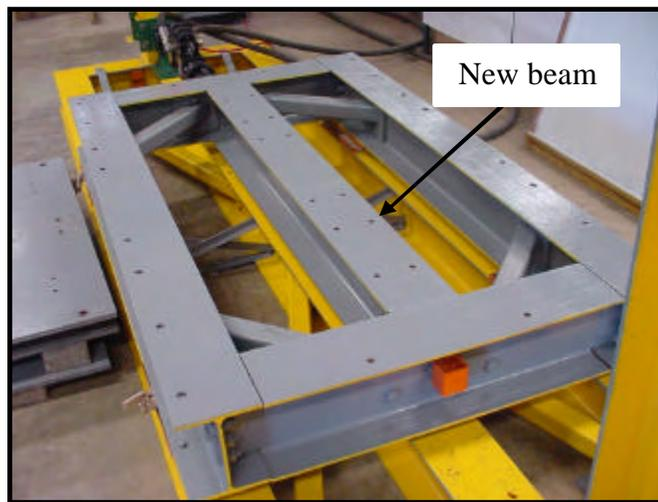
Figure 8.2 New Beam Welded to Simulator Frame.
