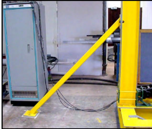
Figure 8.1 Lateral Bracing of Reaction Frame.
