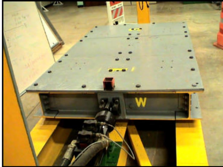
Figure 8.11 Attachment of Actuator to Simulator Platform.
