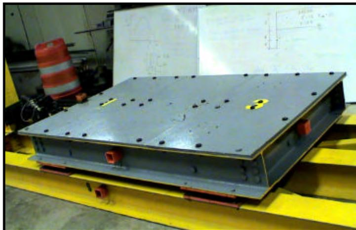
Figure 8.10 Steel Plates Attached to Simulator Frame.
