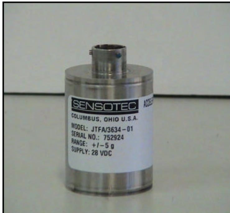
Figure 3.14 Piezoresistive Accelerometer.
