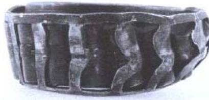
Figure 3. Thermal overheating results on bearings. Taken from [7].
