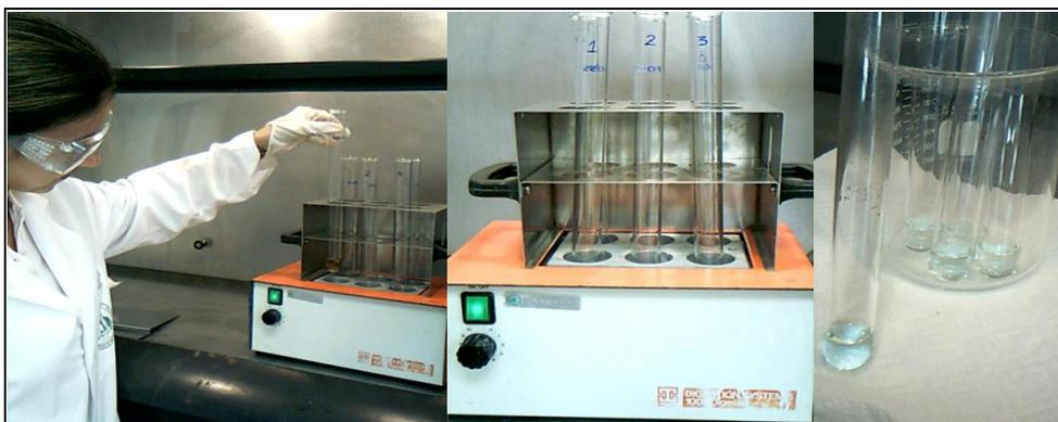
**Figure 11** Nitrogen content (sample digestion)
