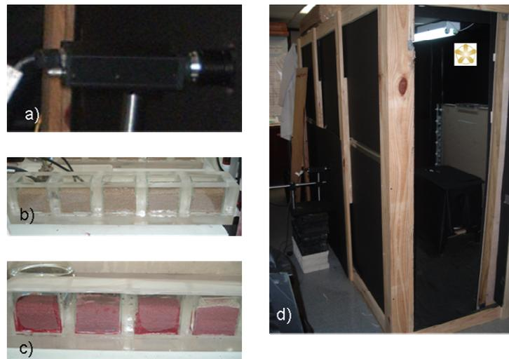
**Figure 5.2 Image acquisition and analysis system: (a) digital camera, (b) calibration soil cells, (c) stained soil cells, and (d) studio room**
