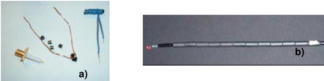
**Figure 3.12 a) Materials for construction of loop antennas, and b) loop antenna**
