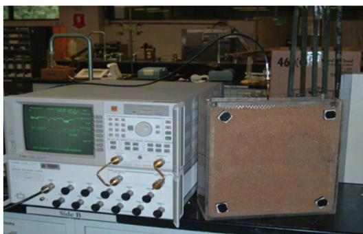
**Figure 3.7 Network Analyzer, multiport test set, and soilBed(type 2, Table 3.2)**
