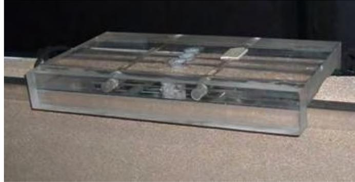
**Figure 3.3 Soil delivery guide**
