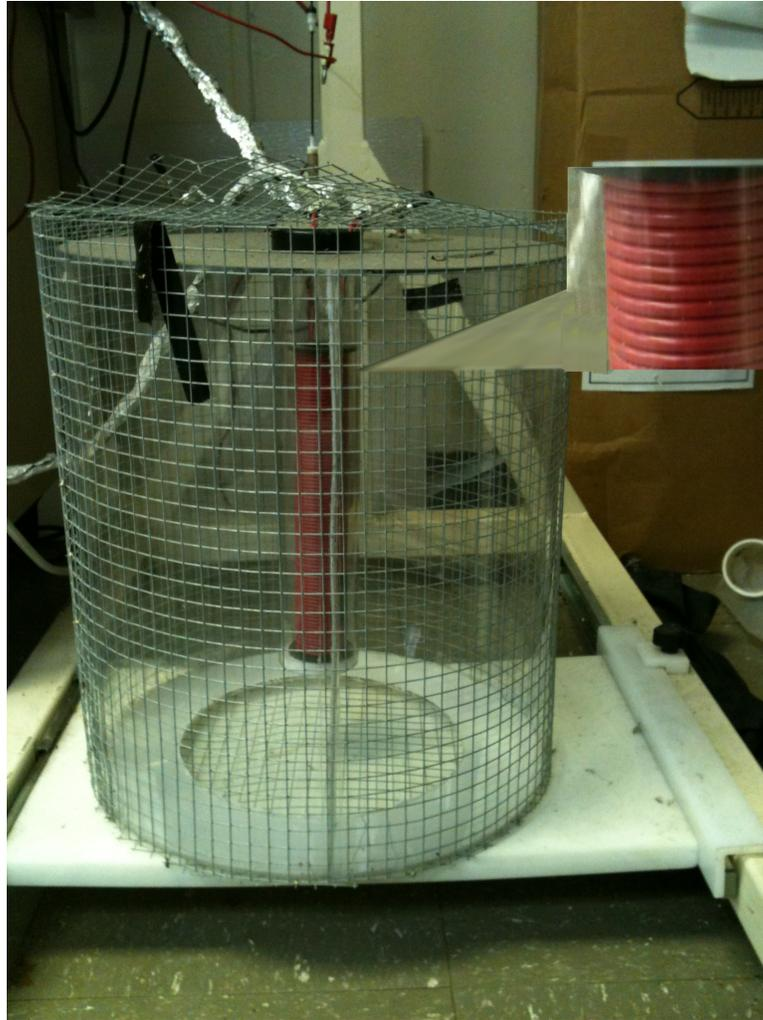
Figure 3–2: Picture of the coils. A Carol A 18 AWG wire was used for the primary and secondary coils.
