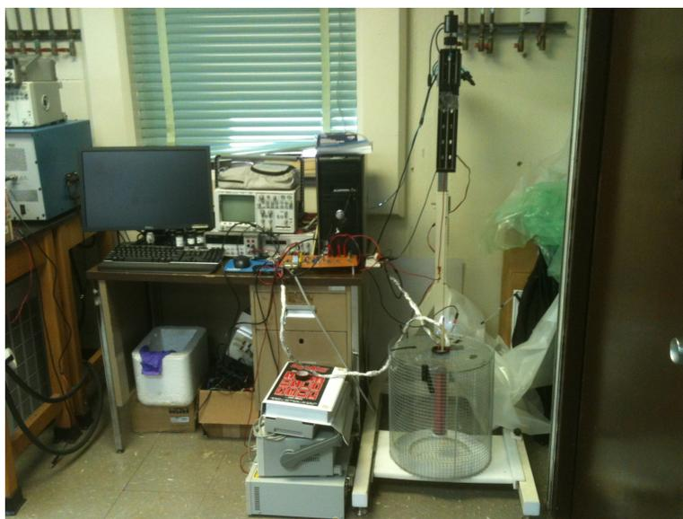
Figure 3–6: Complete AC susceptometer equipment at laboratory facility.
