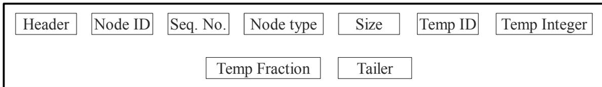
**Figure 27: Data packet protocol designed for the temperature node.**
