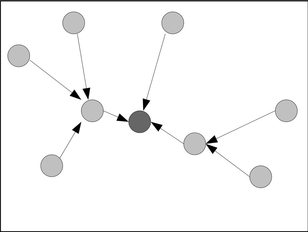
**Figure 24: Diagram depicting a multihop multipoint to point network with sensor nodes (light gray) sending data to a base station (dark gray).**
