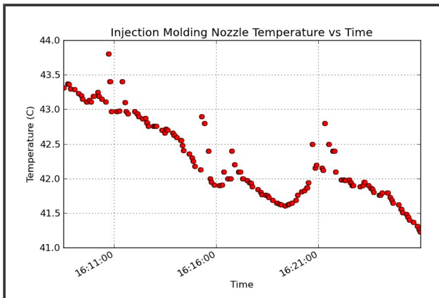
**Figure 40: Temperature of air around injection molding nozzle.**
