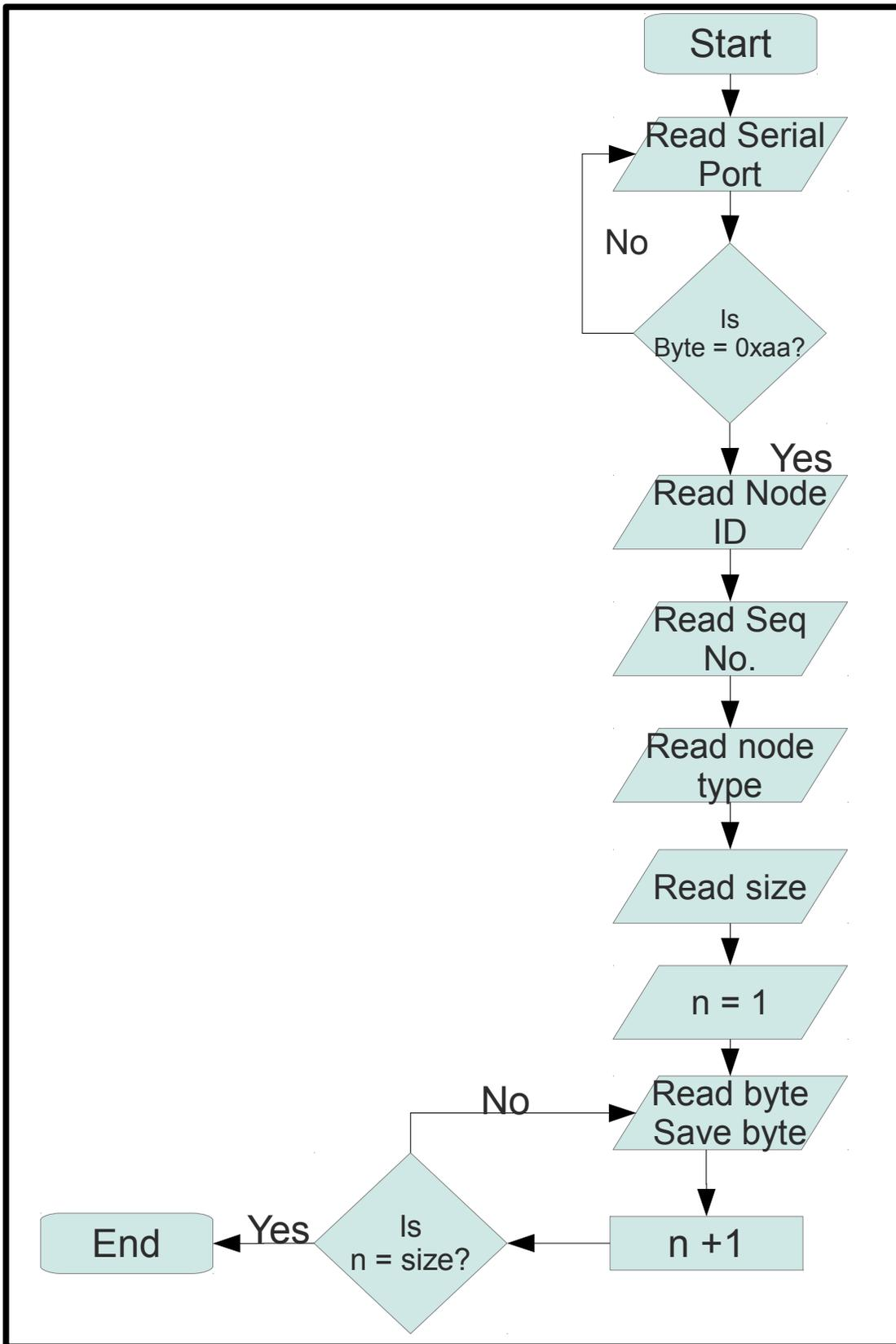
Figure 29: Flowchart describing the data capturing algorithm used to read and save data from the serial port.
