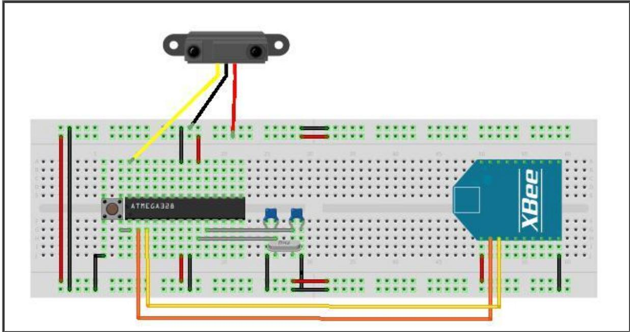
Figure 19: Counter node design on breadboard on a standalone microcontroller setup.
