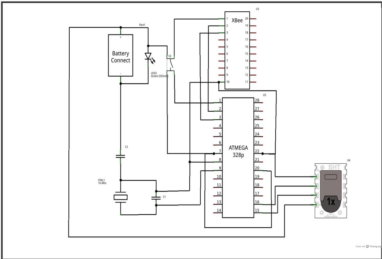
**Figure 18: Circuit schematic of temperature sensor node, including all peripheral components.**
