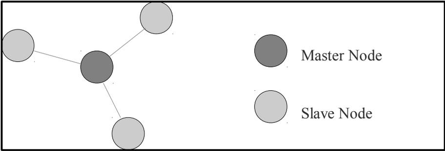
**Figure 5: Bluetooth piconet configuration with three slaves connecting to a master.**
