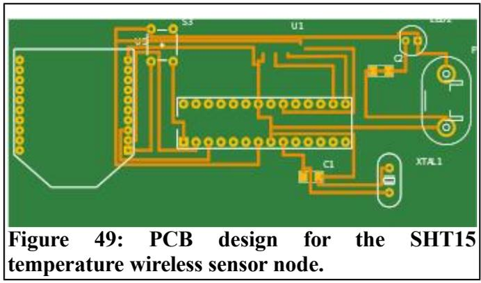
**Figure 49: PCB design for the SHT15 temperature wireless sensor node.**
