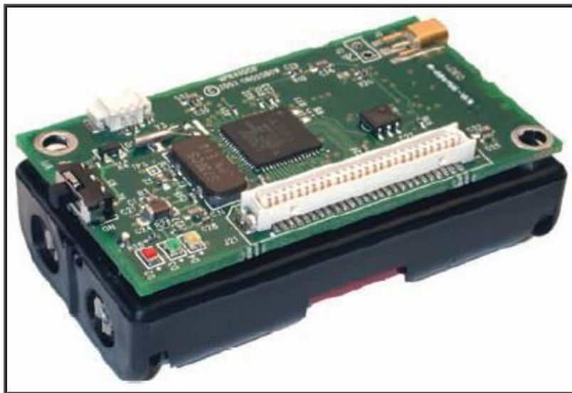
**Figure 3: Photograph of a Mica2 Mote, a revision of the Mica Mote.**
