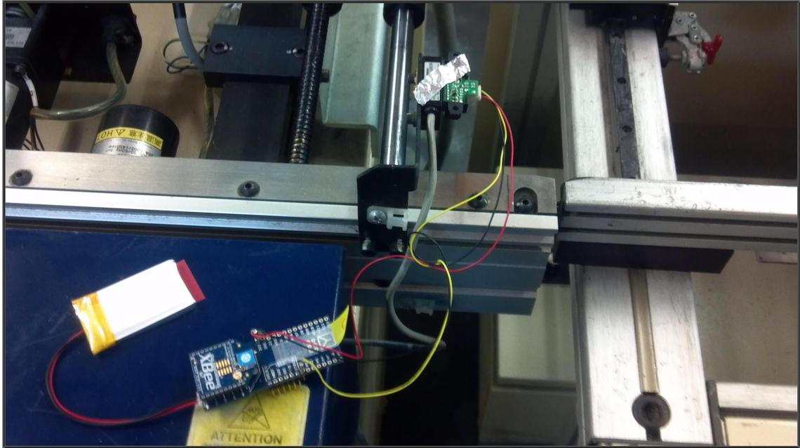
Figure 36: Counter node deployment on top of conveyor line.
