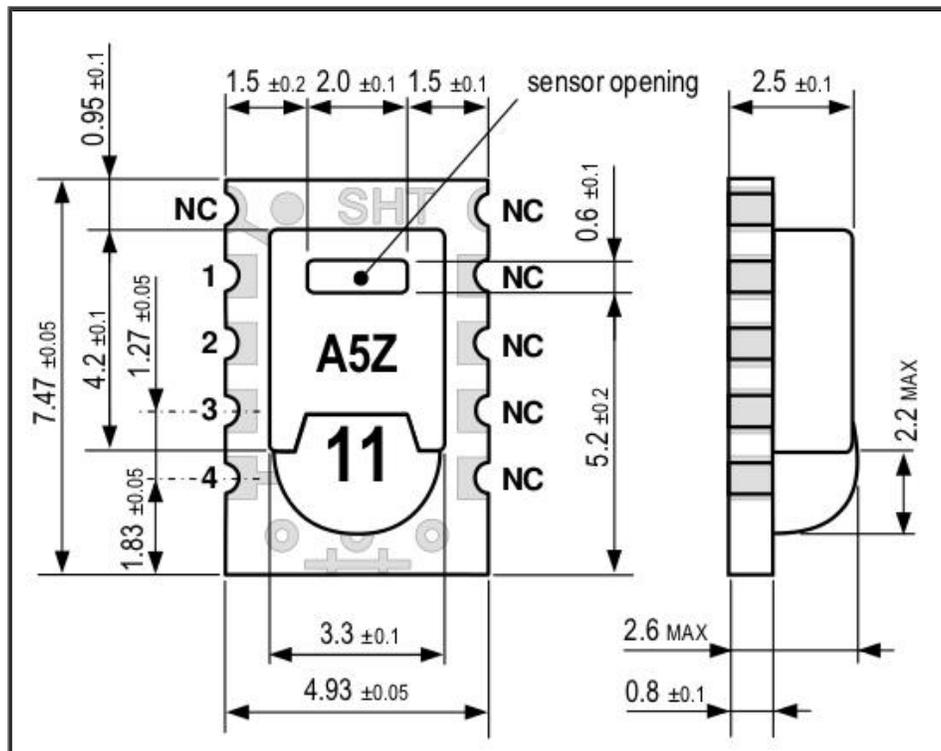
**Figure 14: Mechanical drawing of an SHT15 Temperature and Humidity sensor as provided by manufacturer Sensirion.**
