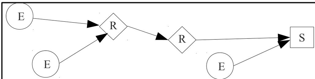
**Figure 1: Proposed WSN featuring a multi-hop topology. Pictured are End Devices (E), Routers (R), and a Sink (S).**
