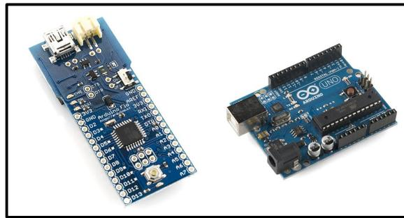
**Figure 10: Arduino Fio (left) and Arduino Uno (right) development boards. Images provided by Sparkfun Electronics.**
