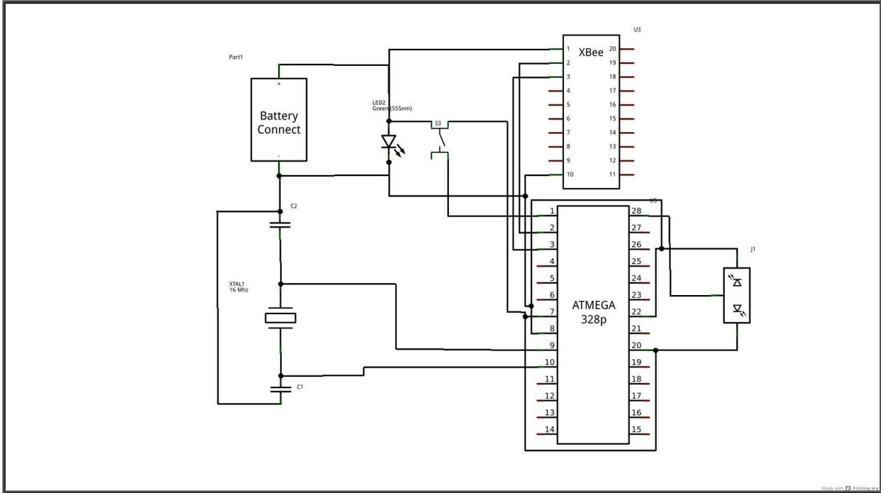
**Figure 17: Schematic for the counter node, including peripherals such as the microcontroller clock, capacitors, and power supply.**
