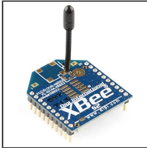
**Figure 12: Xbee Series 2 radio with wire antenna. Image provided by distributor Sparkfun Electronics.**
