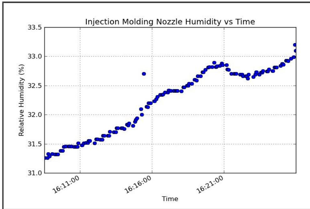
**Figure 41: Relative humidity of air around injection molding nozzle.**
