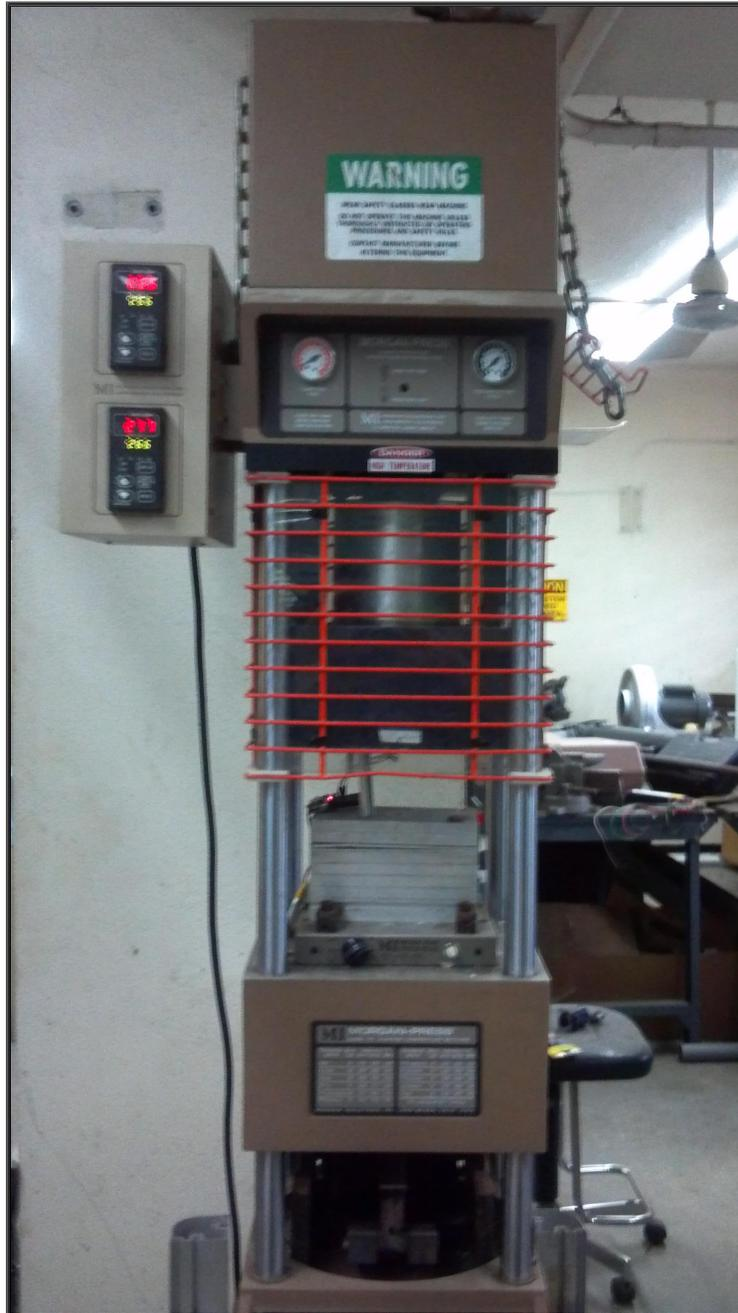
**Figure 32: Injection molding machine on which Sensor node 1 was placed to measure nozzle temperature.**
