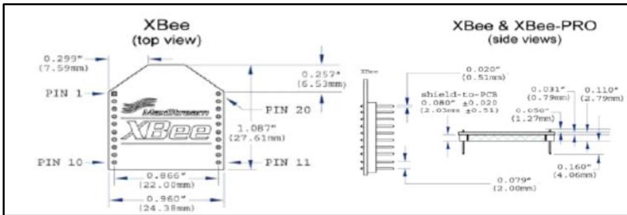
Figure 13: Mechanical drawings of Xbee radios as provided by manufacturer Digi, Inc.
