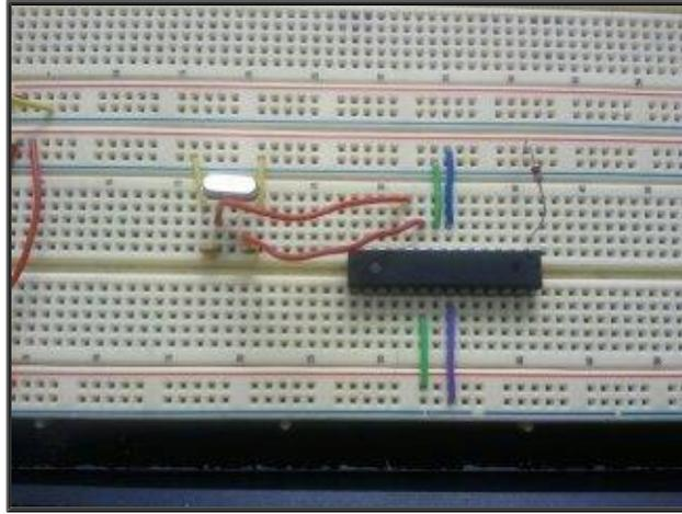
**Figure 11: Photograph of assembled microcontroller (DIP) with peripheral components such as crystal oscillator and capacitors.**
