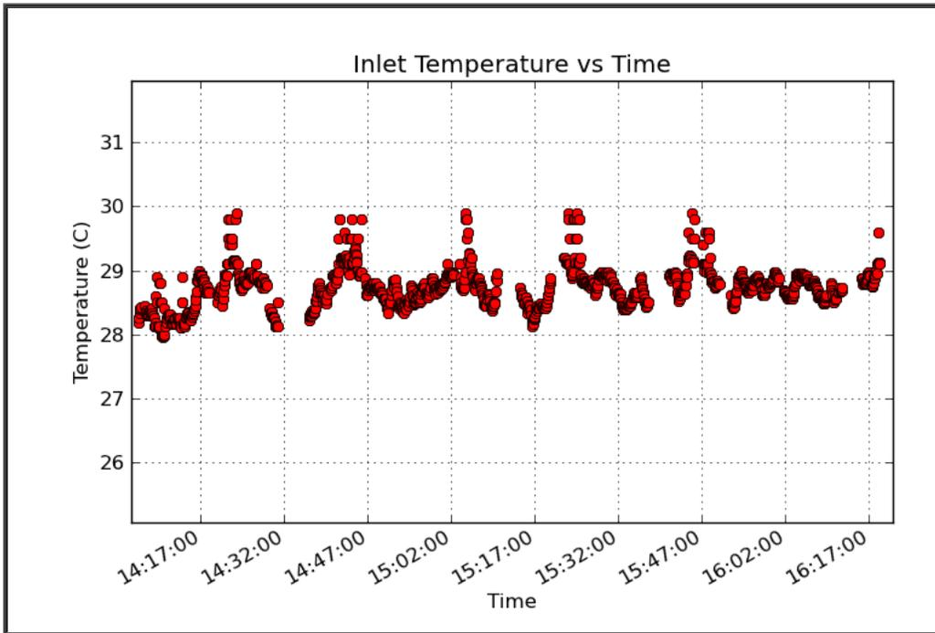
Figure 44: Inlet temperature of reflow oven.
