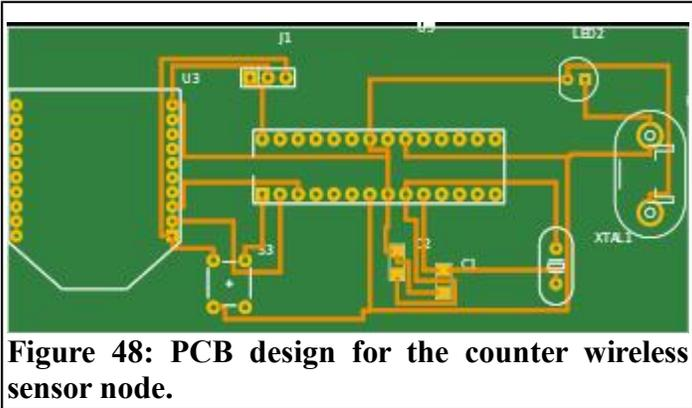
**Figure 48: PCB design for the counter wireless sensor node.**
