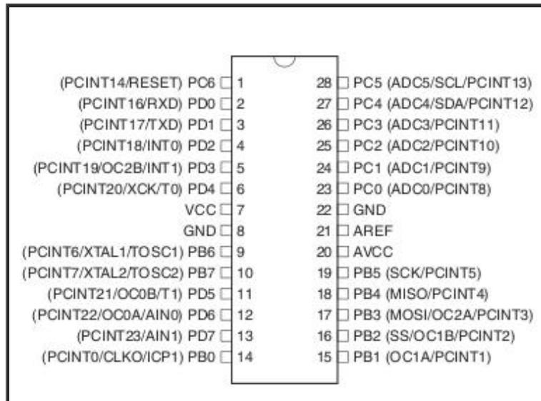
**Figure 9: I/O diagram of an Atmega 328p microcontroller in a dual inline package (DIP).**
