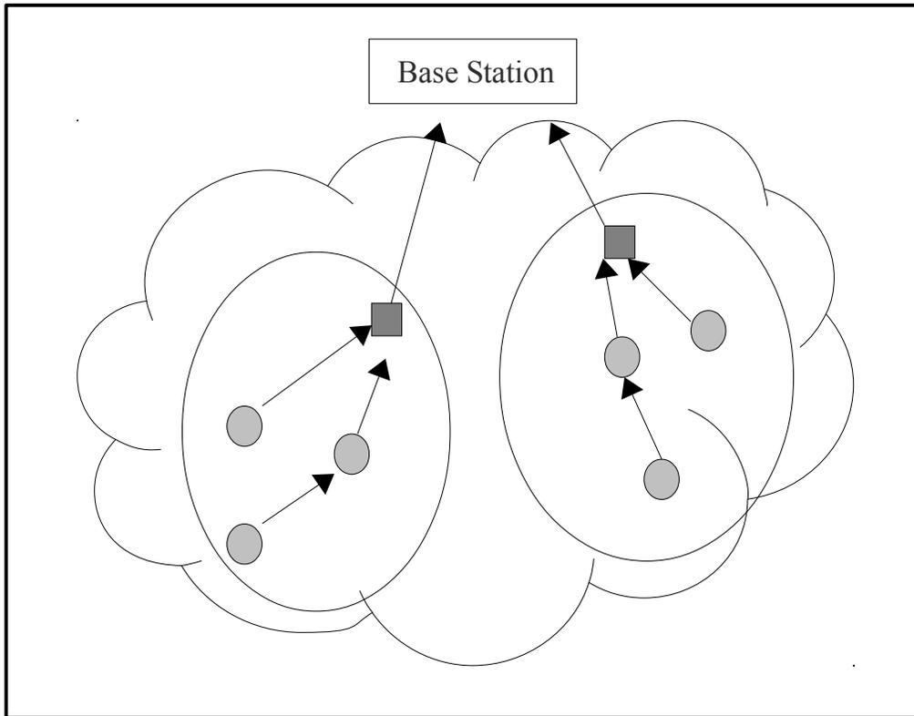
**Figure 25: Diagram of a multihop clustered network topology. Circles denote sensor nodes, squares denote cluster heads.**
