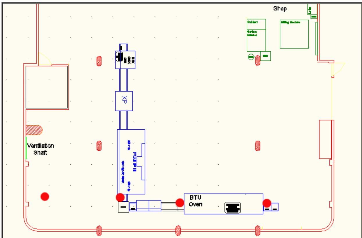
Figure 35: Layout of Manufacturing Line. Node locations are denoted by red circles.
