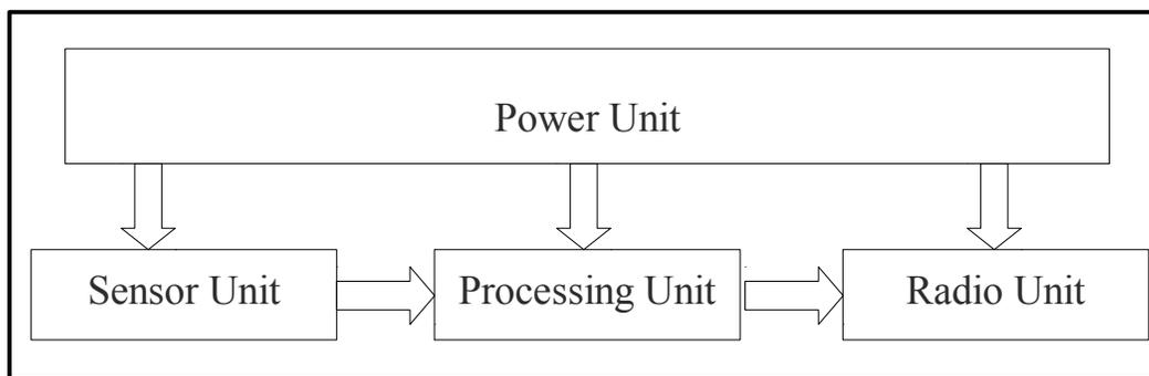
**Figure 2: Diagram of proposed wireless sensor network node.**
