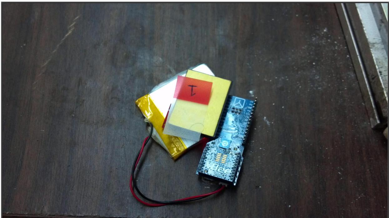
**Figure 34: Deployment of sensor node 1 on work table of manufacturing laboratory.**
