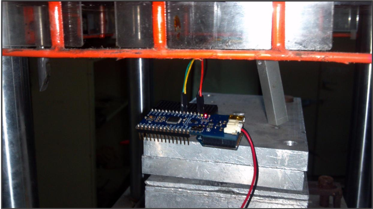
**Figure 33: Deployment of sensor node 2 on the injection molding machine. The sensor itself is not visible due to the tight spacing inside the injection chamber.**
