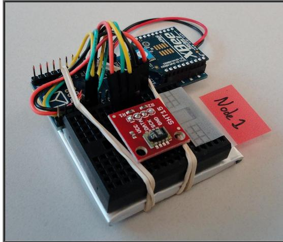
**Figure 21: Photograph of assembled temperature sensing node using an Arduino Fio board. Lithium Polymer battery can be seen under the board in grey.**
