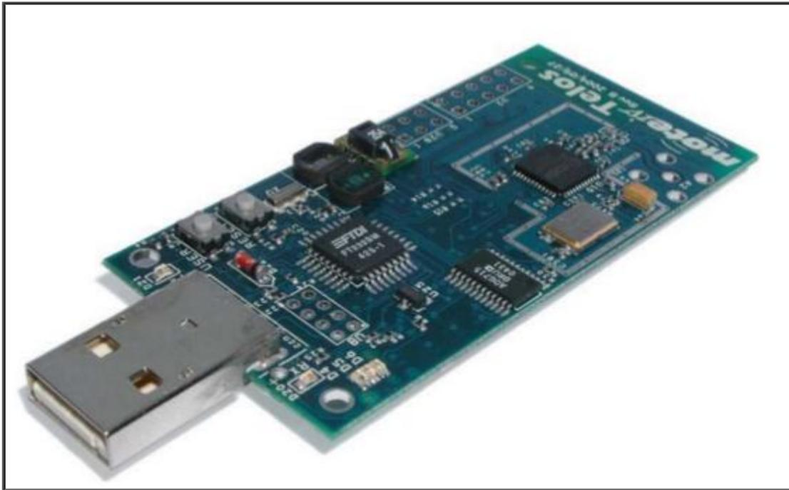
**Figure 4: Photograph of a Telos wireless module.**
