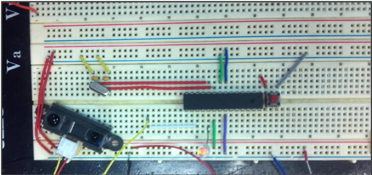
**Figure 22: Counter node on a standalone Atmega 328p. Xbee module is not attached due to pin spacing issues.**
