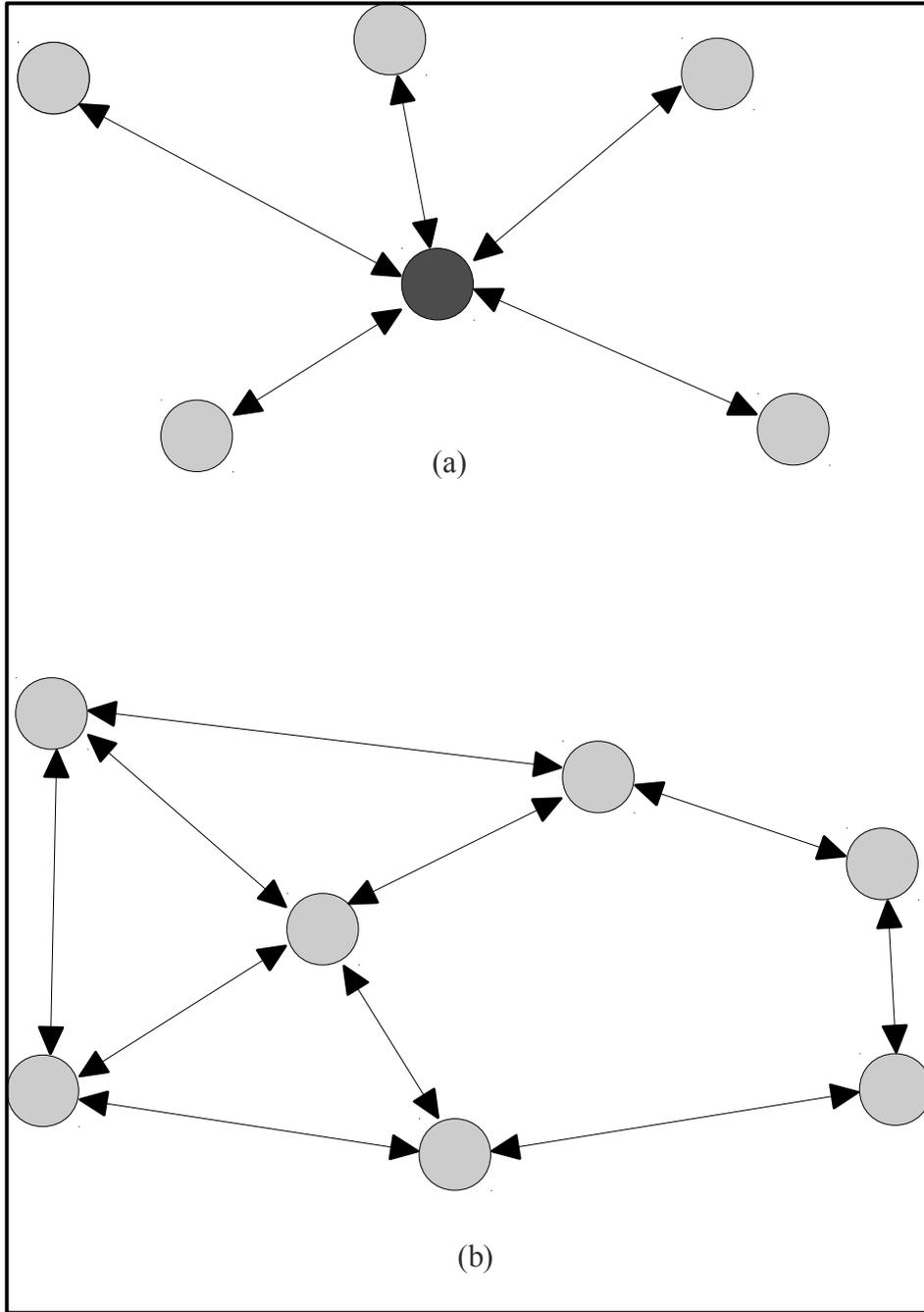
**Figure 23: The network topologies possible with the IEEE 802.15.4 Standard. (a) Shows a Star topology with various nodes communicating with a single base station, (b) shows a P2P network where all nodes can communicate with any adjacent nodes.**
