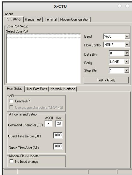
**Figure 30: X-CTU graphical user interface PC Settings tab.**
