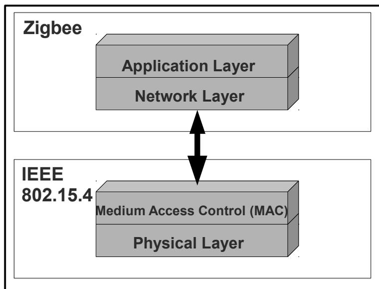
**Figure 6: Zigbee Standard Stack.**
