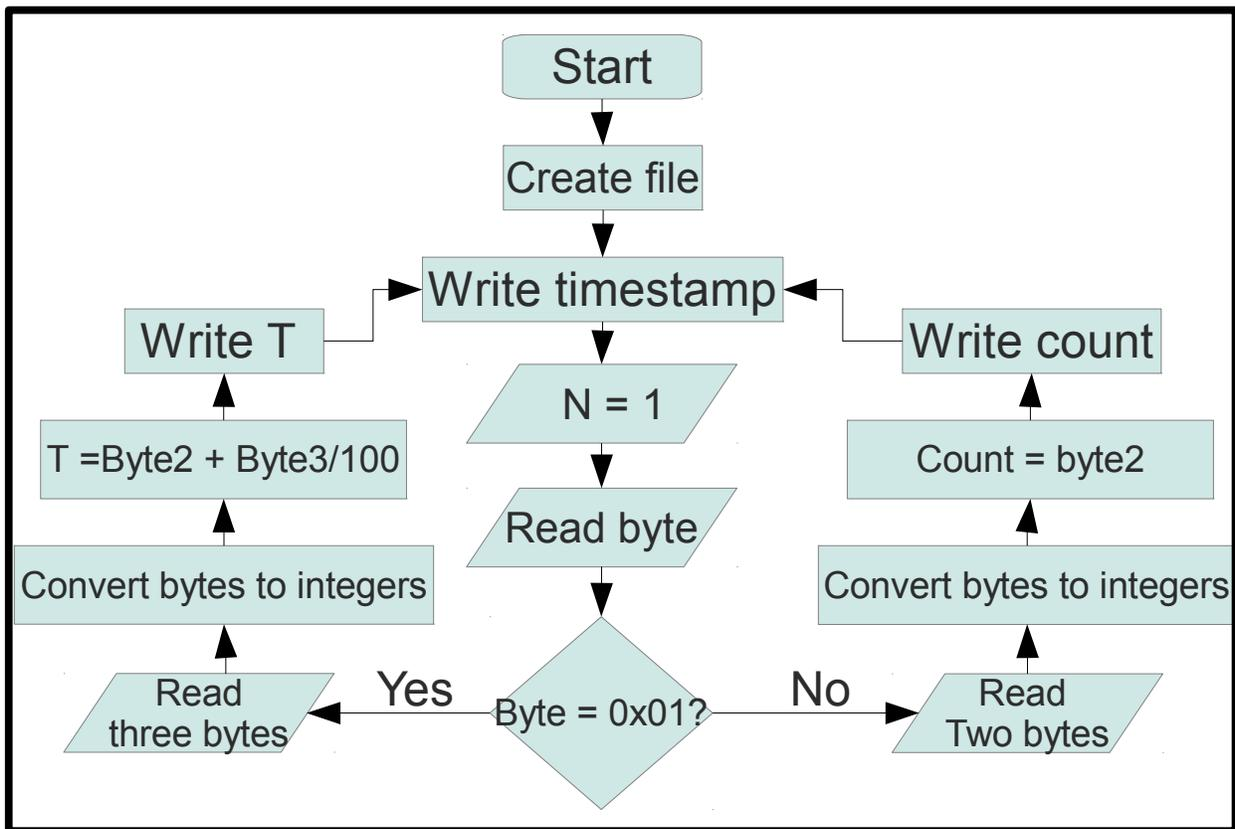
Figure 28: Flowchart of data parsing algorithm for two types of single sensor nodes.
