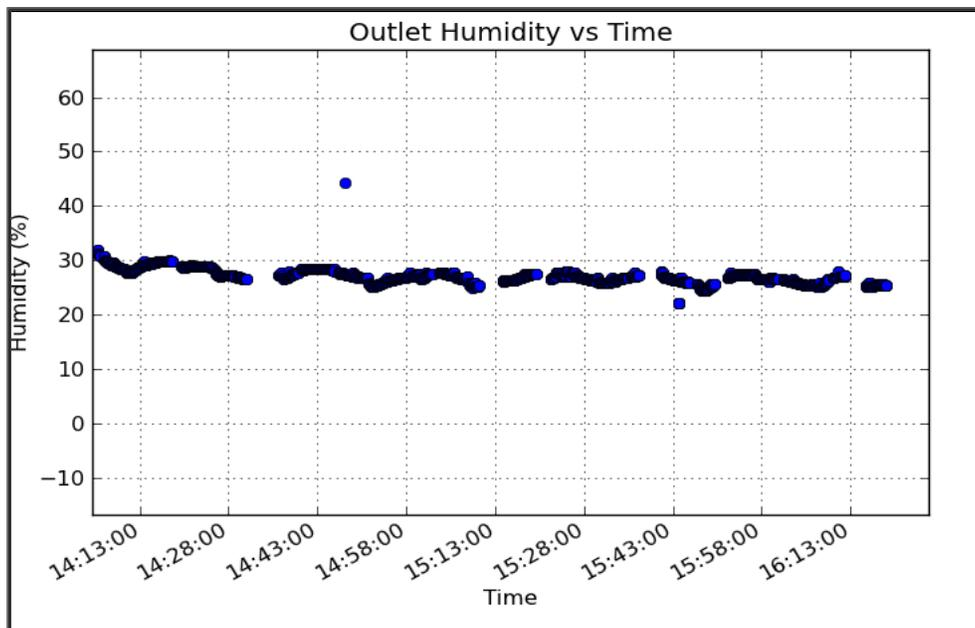
**Figure 47: Reflow oven outlet humidity.**
