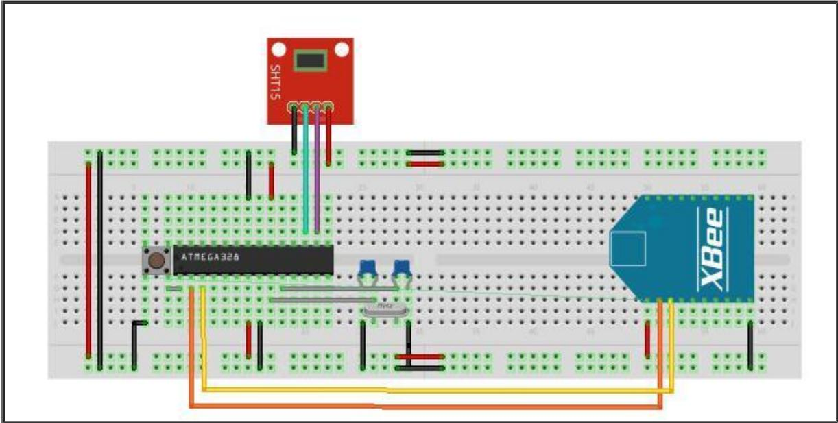
Figure 20: Temperature node design on breadboard on a standalone microcontroller setup.
