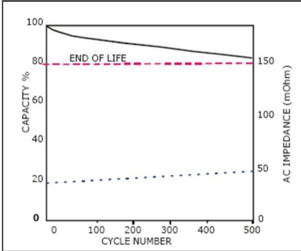
**Figure 8: Decrease in maximum capacity of Lithium Polymer batteries as shown by Salameh, et. al.**
