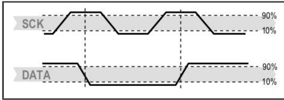
**Figure 15: Example of the starting sequence code. The high and low pulses can be seen on both the SCK (upper) and DATA (lower) lines.**
