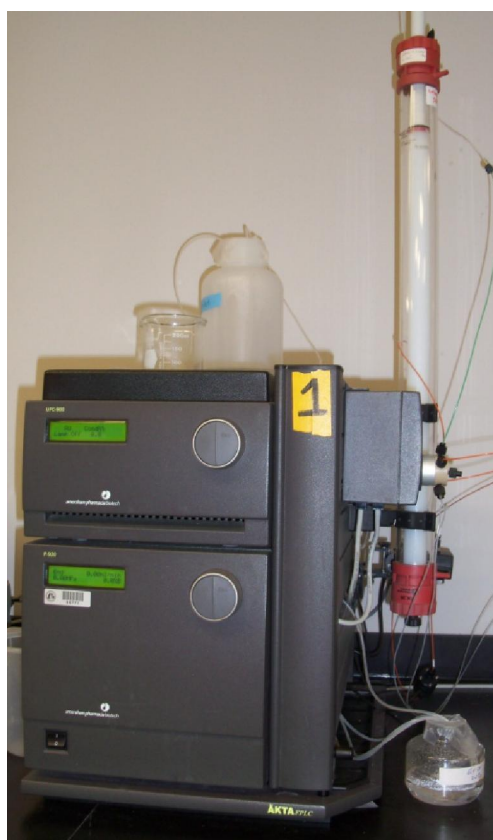
Figure 2.2. Fast performance liquid chromatography (FPLC) equipment used for the separation and purification of the different hemoglobins.
