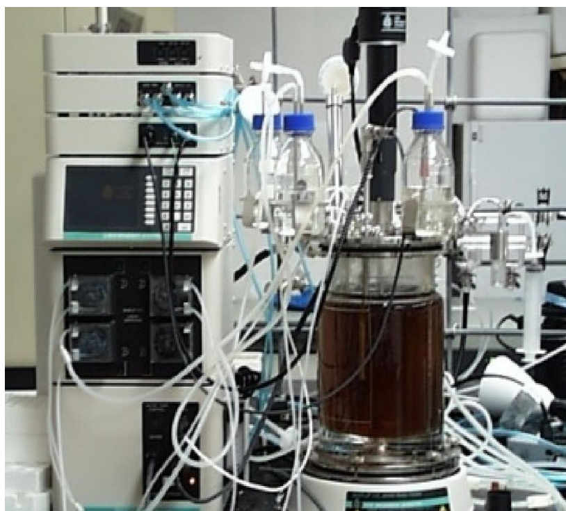
Figure 2.4. Fermentation system for bacterial growth and protein expression. It shows the control unit the vessel, and the connections.
