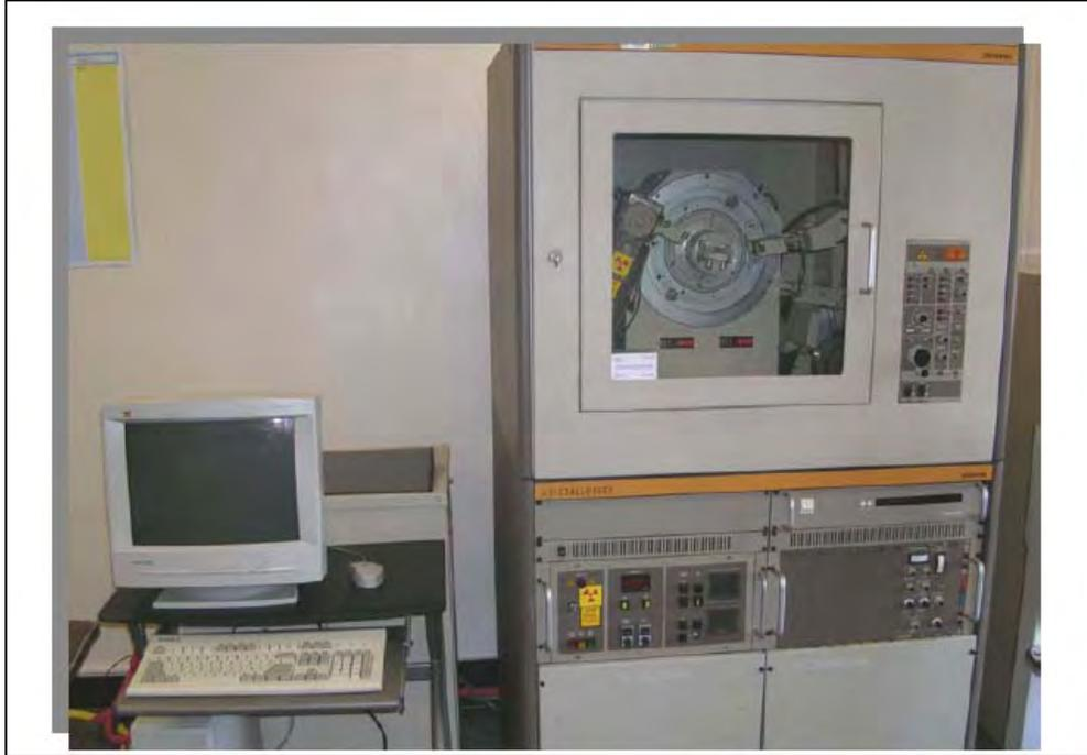
Figure 16. XRD Siemens D500 unit at the Department of Engineering Science and Materials UPRM.
