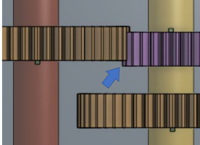
Figure 17: Experiment 2 Example of Misalignment Error between Gears
