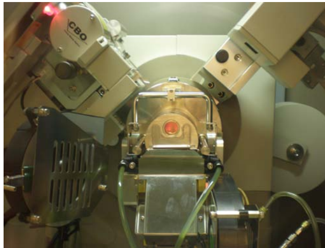
Figure 3.6 Rigaku XRD executing a high temperature test.
