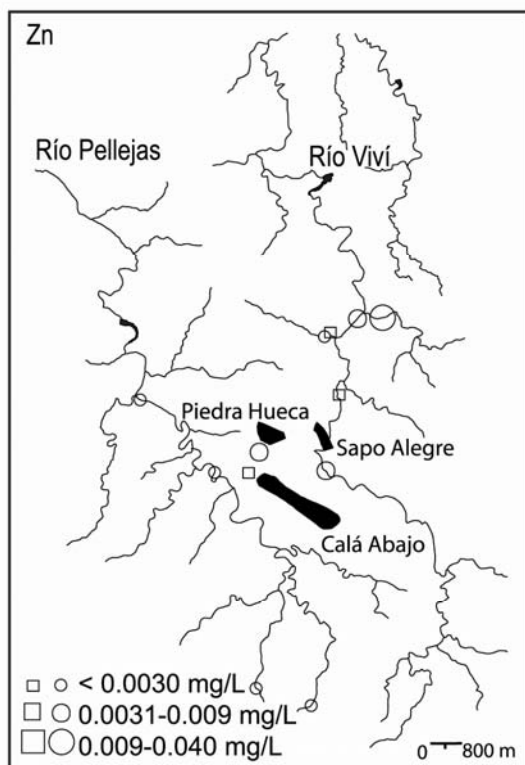
Figure 12 Cont. Maps showing concentrations of selected cations, anions and hardness of water for surface (circles) and groundwater sites (squares).
