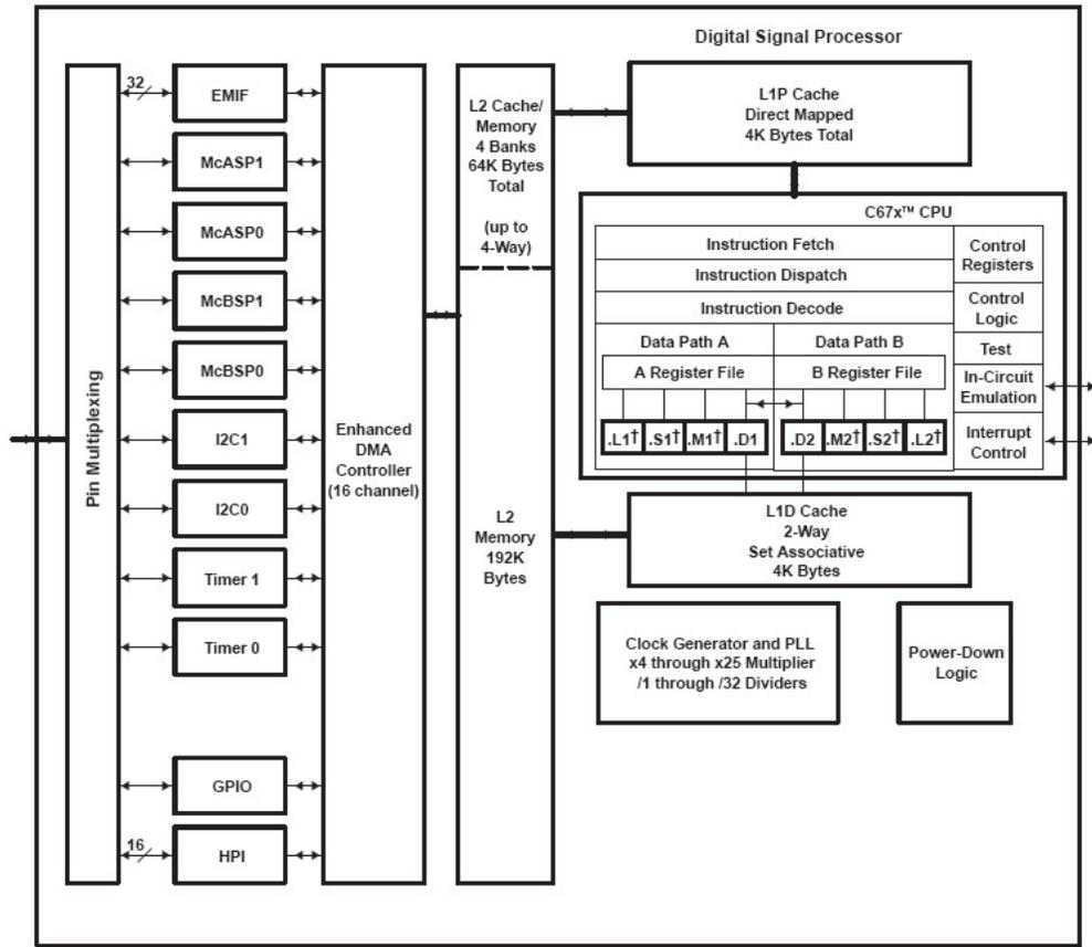
Figure 25 Block diagram of C6713 DSP. Taken from [33]
