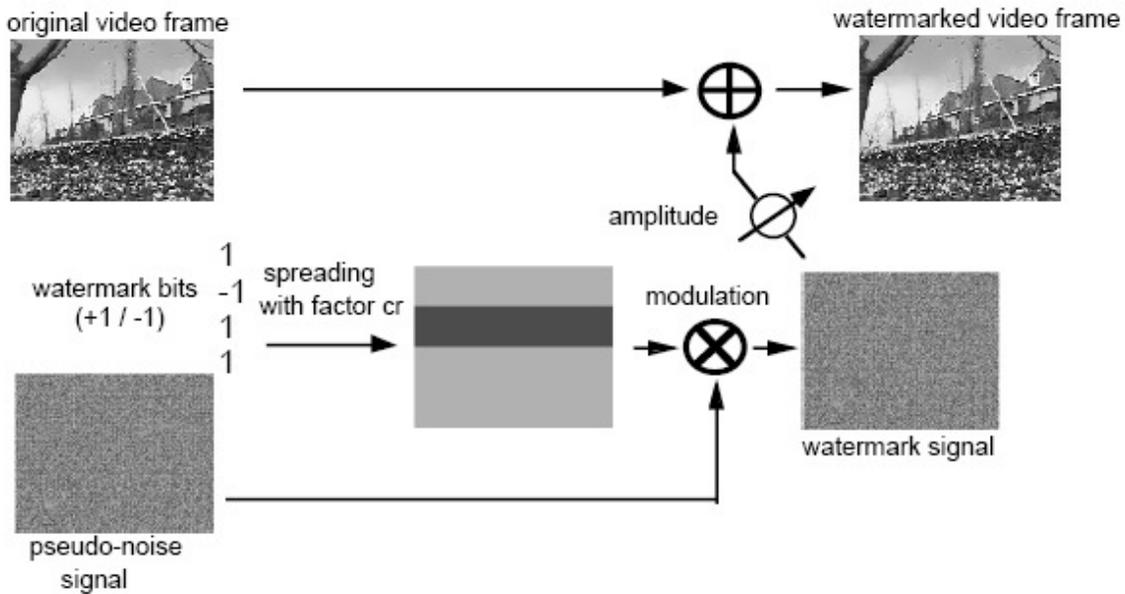
Figure 13 Watermark generation and addition to the video signal. Taken from [42]
