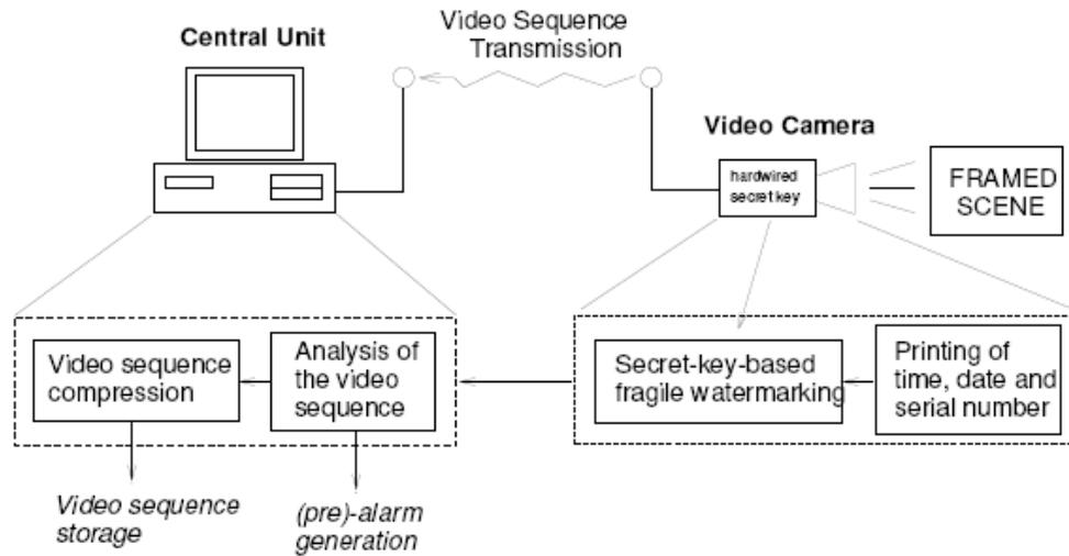
**Figure 9 Watermarking Authentication System for AVS data. Taken from [29]**
