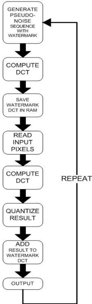
**Figure 20 Dataflow description for the developed architecture**
