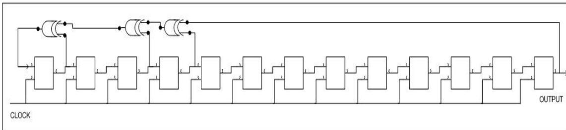
**Figure 21 13-bit Linear Feedback Shift Register with Maximum Sequence Length**
