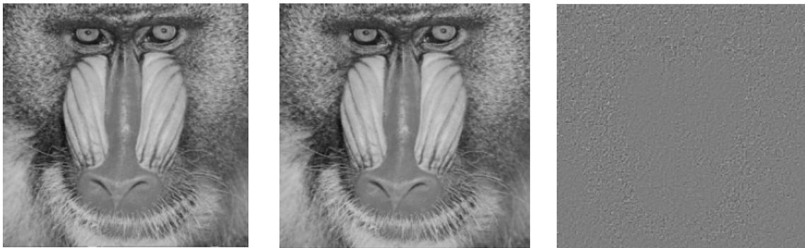
**Figure 3 Example of watermarking of an Image. Left picture: original image. Middle picture: watermarked image. Right picture: difference between original and watermarked images. Taken from [1]**
