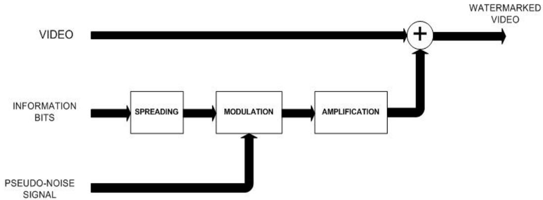
Figure 12 Watermark generation and addition to the video signal [42]
