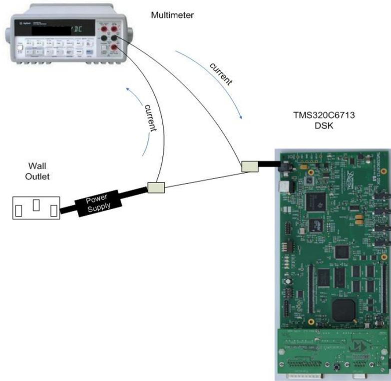
**Figure 27 Configuration for measuring the power dissipation of the DSP device**
