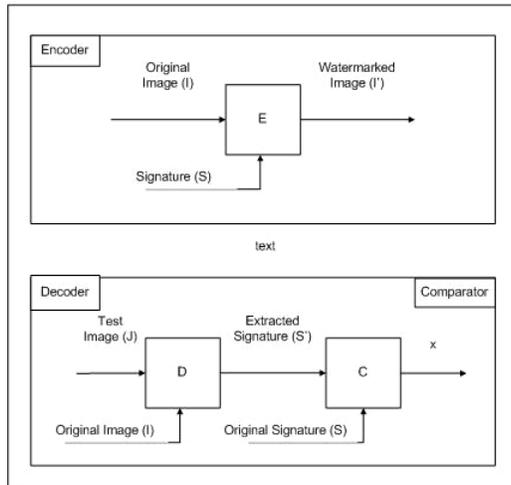
**Figure 4 Block diagram of the encoder and decoder stages of a watermarking system [6]**
