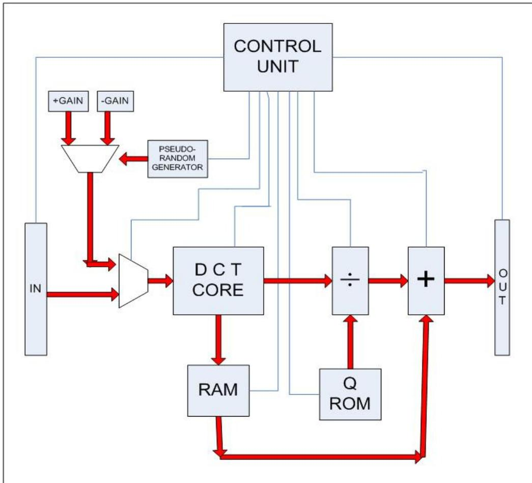
**Figure 19 Architecture of the proposed watermarking system**
