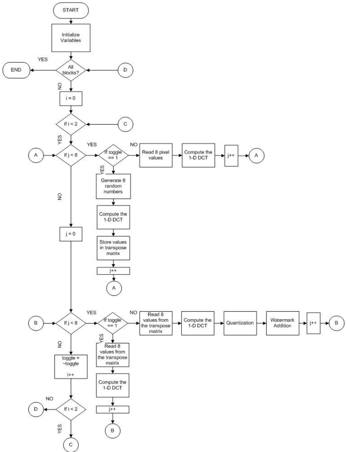
Figure 26 Flowchart of developed DSP code
