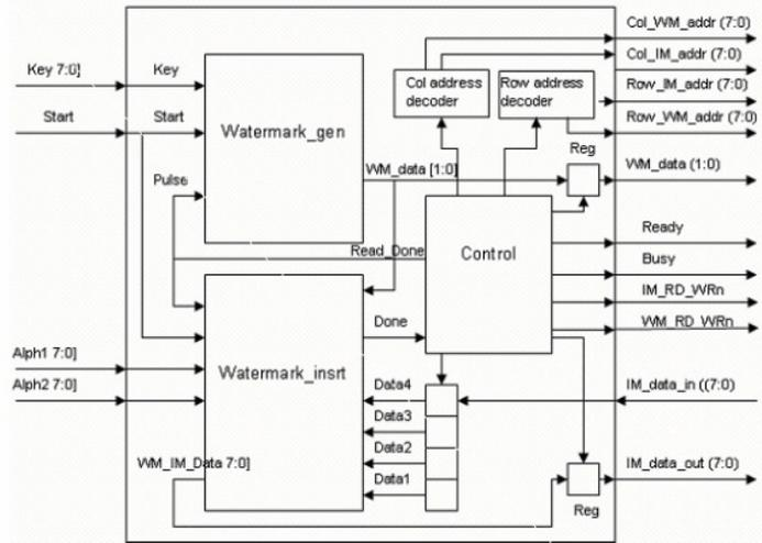
**Figure 8 Block Diagram of the Mohanty FPGA Implementation. Taken from [12]**
