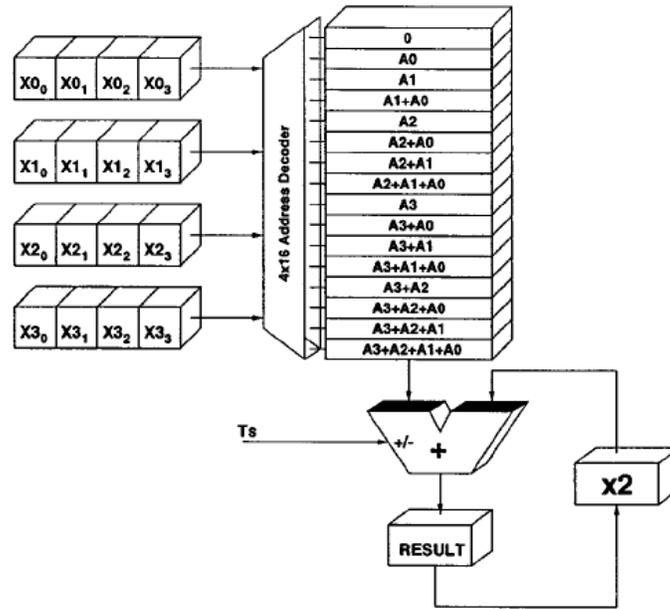
Figure 24 Block diagram of the RAC structure. Taken from [51]
