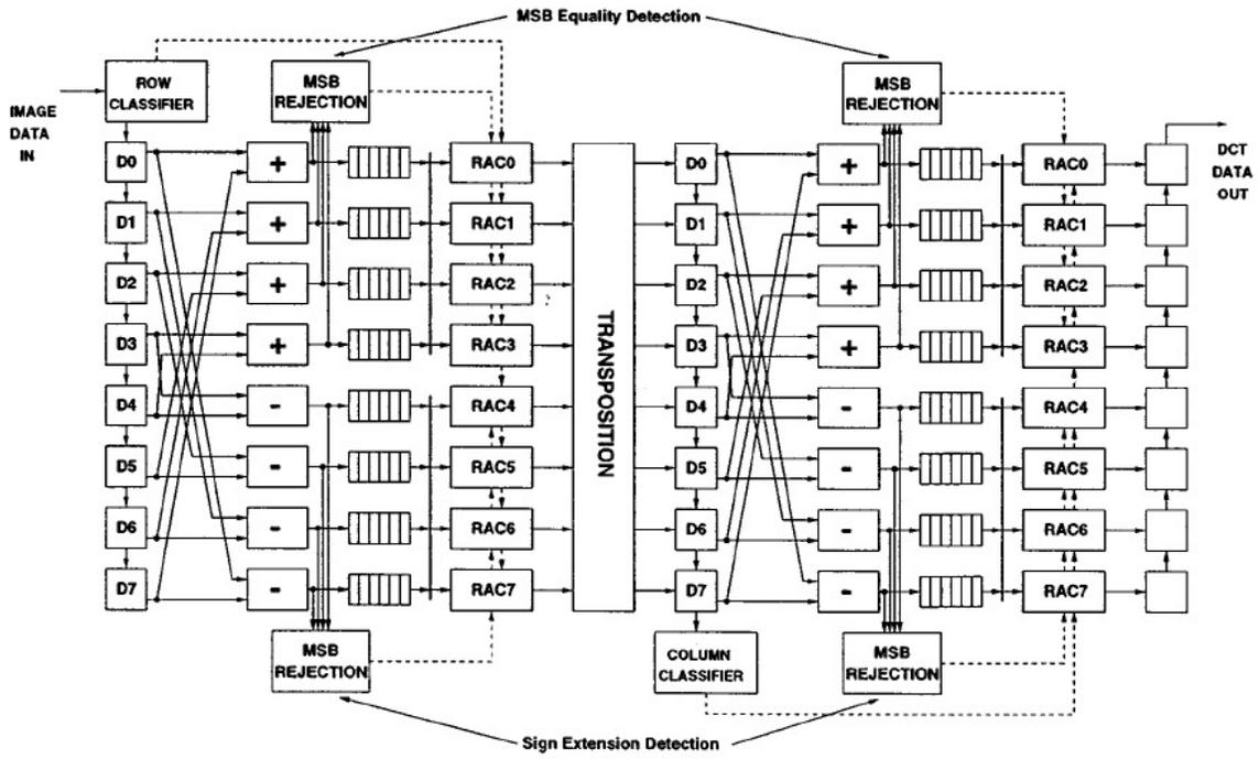
Figure 23 Block diagram of DCT Core, in detail. Taken from [51]
