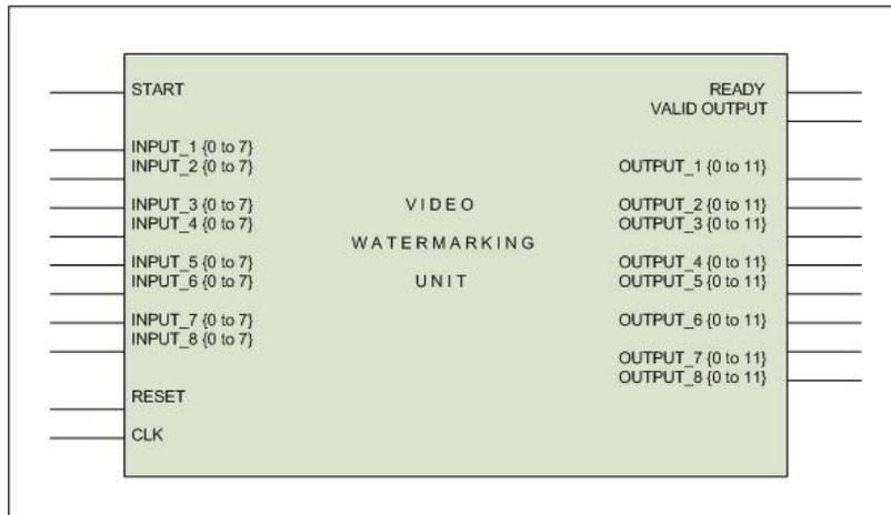
**Figure 18 Top view of the proposed watermarking implementation**
