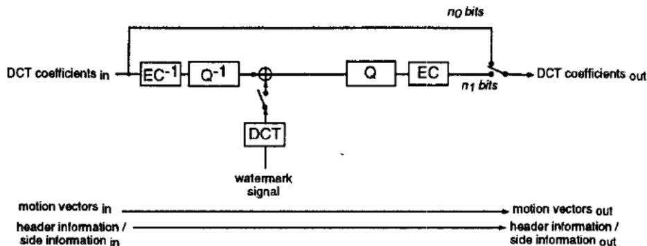
**Figure 16 Watermarking in MPEG-2 domain. Taken from [42]**
