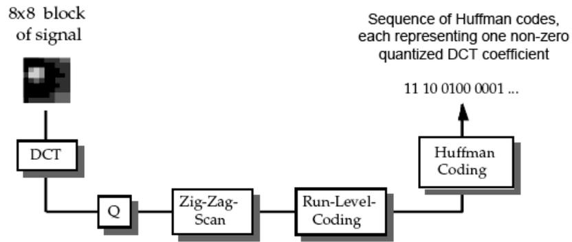
**Figure 11 Simplified block diagram of JPEG compression. Taken from [40]**
