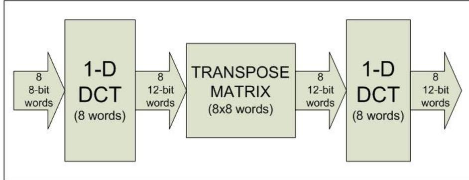
**Figure 22 Simplified block diagram of DCT core**
