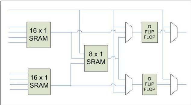
**Figure 17 Simplified FPGA programmable logic block**
