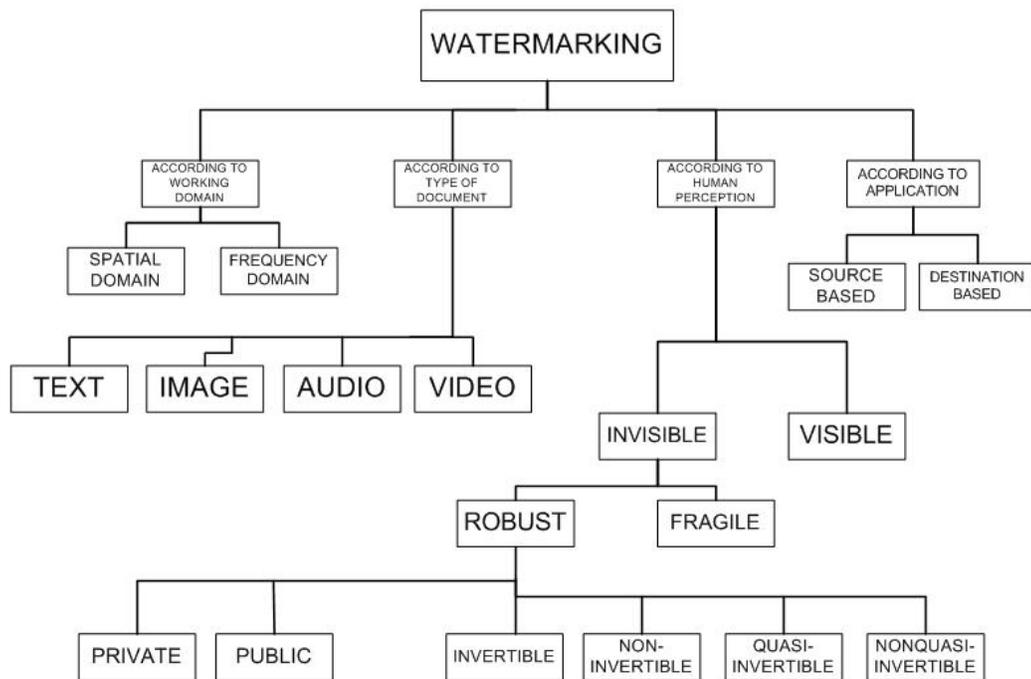
**Figure 5** Types of digital watermarking schemes [6]
