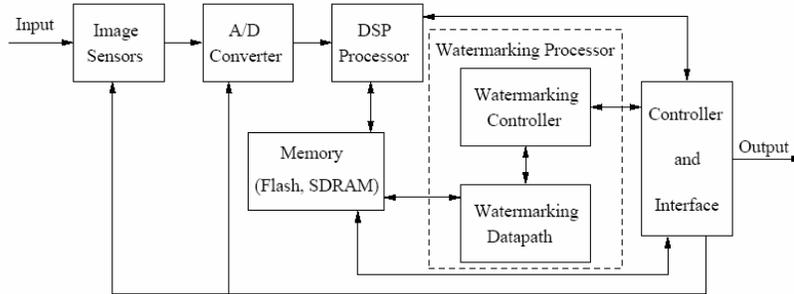
**Figure 7 Diagram of the Mohanty VLSI implementation. Taken from [13]**
